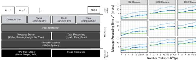
Pilot-Streaming on Serverless High-Level Architecture and Interactions: Pilot-Streaming enables the unified management of batch and streaming compute tasks on serverless infrastructure. It orchestrates the setup of Kinesis and Lambda and manages the streaming workload.
