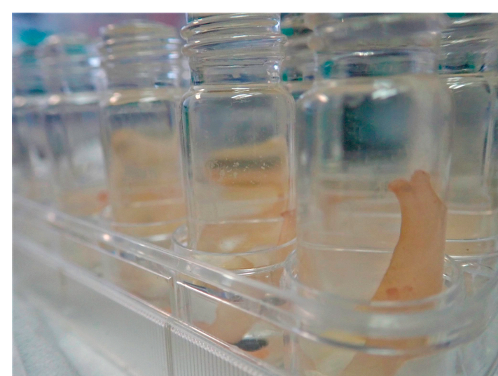
Fig. 5. Geoduck respiration rate measurements completed in 4-ml vials (PreSens).
