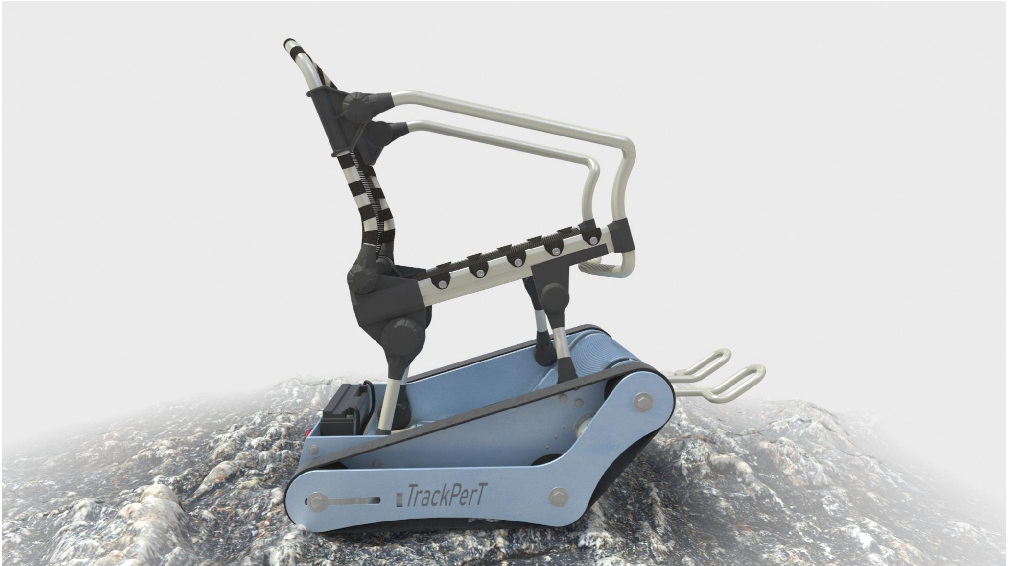
Figure 2: A side view of the novel wheelchair. Note the foot rests to the front, to provide a bracing point for user stability. Note also the relatively low slung seat which will aid stability in offroad environments.
