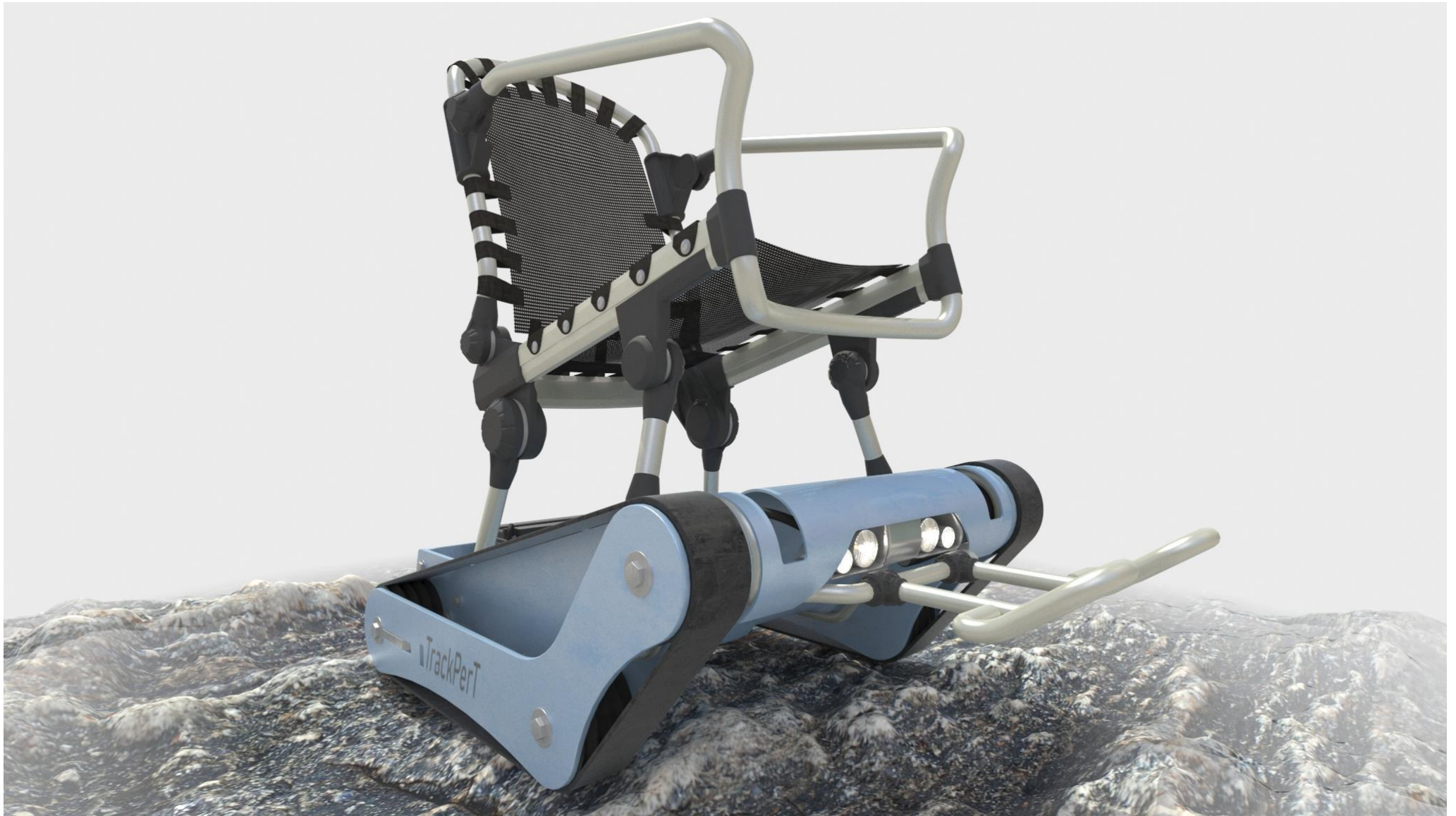
Figure 3: A front view of the novel wheelchair. Note that the youthful and 'aggressive' styling, and front-facing headlights. This view shows the raised front tracks, which allows bumps and curbcuts to be traversed.
