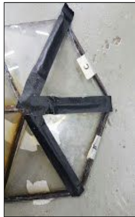
Method B- Slotting the acrylic into the metal frame
