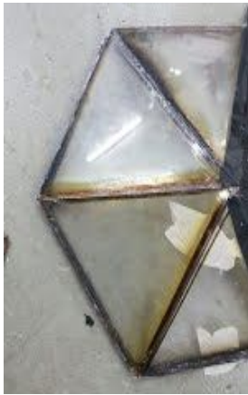
Method A- Overlapping the acrylic onto the metal frame
