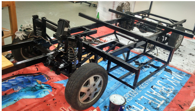
The painted and modified chassis.
