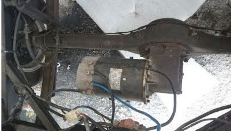
Photo showing the DC motor mounted to the shaft.
