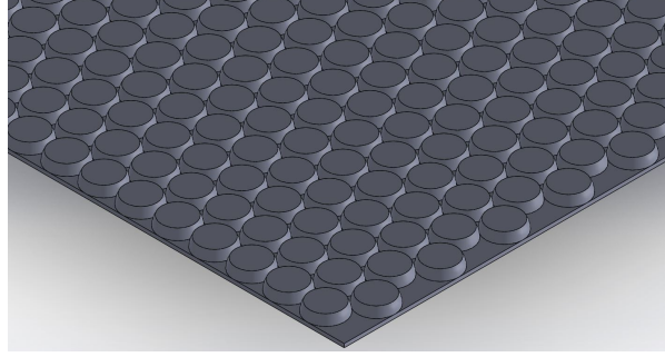
Figure 40: Isometric view of the micro-textured 3D CAD model, obtained through linear pattern of the unit cell shown in Figure 39a.
