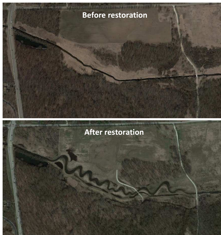
Figure 2. Aerial photographs of (A) pre-restoration (2013) and (B) restored (2017) study stream reach geomorphology. Aerial imagery obtained from Google Earth.
