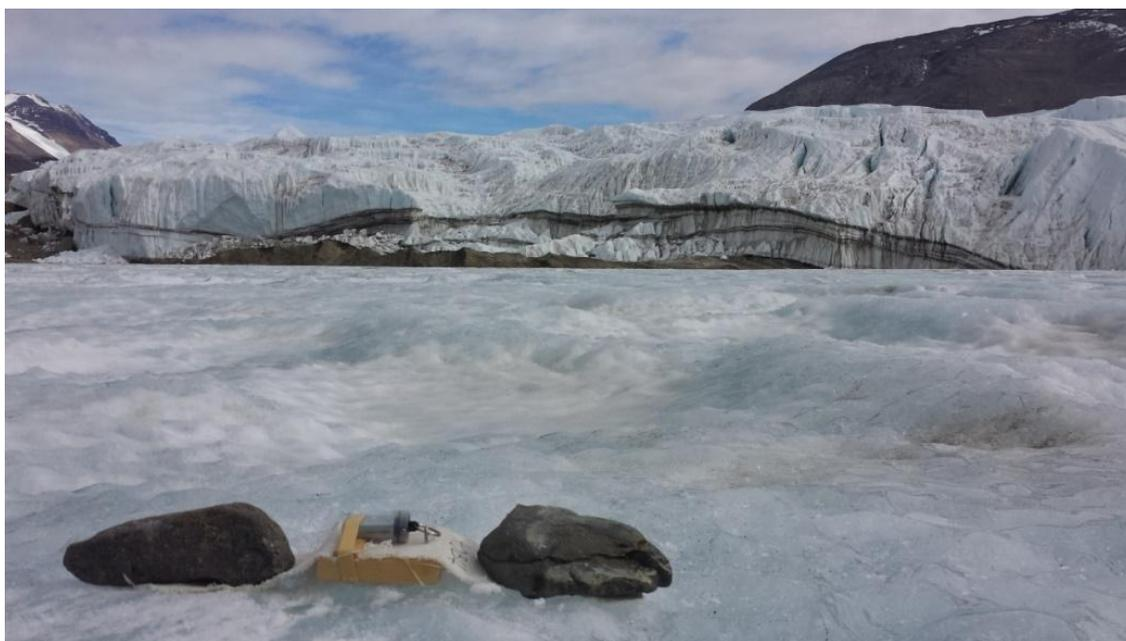
**Fig. 6.** Onset HOBO sensor and sensor mount deployed at West Lobe Bonney.
