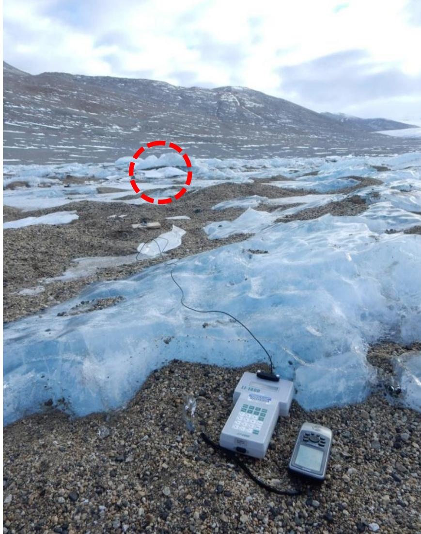
**Fig. 5.** LI-1400 Li-Cor handheld data logger and LI-190 Li-Cor Quantum sensor used to collect field measurements. Logger is shown beside a handheld GPS unit in the foreground. The logger was connected to the Quantum sensor via a  $\approx 3$  m long cable, pictured in the background (circled to help identify).
