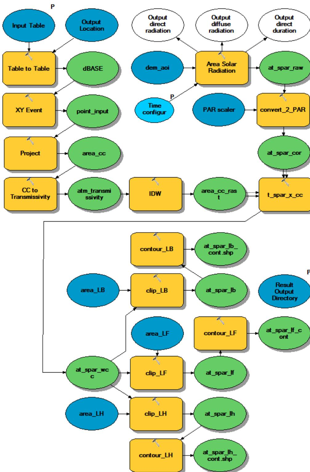
**Fig. 11, Appendix A.** Area T-sPAR model flow chart viewed in the ArcGIS model editor. Inputs are in blue, processes in yellow, outputs in green. Dotted lines indicate precondition fields. The letter “P” indicates fields that can be manipulated by the user.
