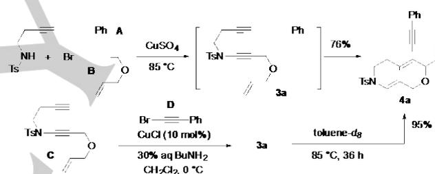
Scheme 2. Initial observation of unexpected transformation in the coupling of sulfonamide with bromoalkyne
