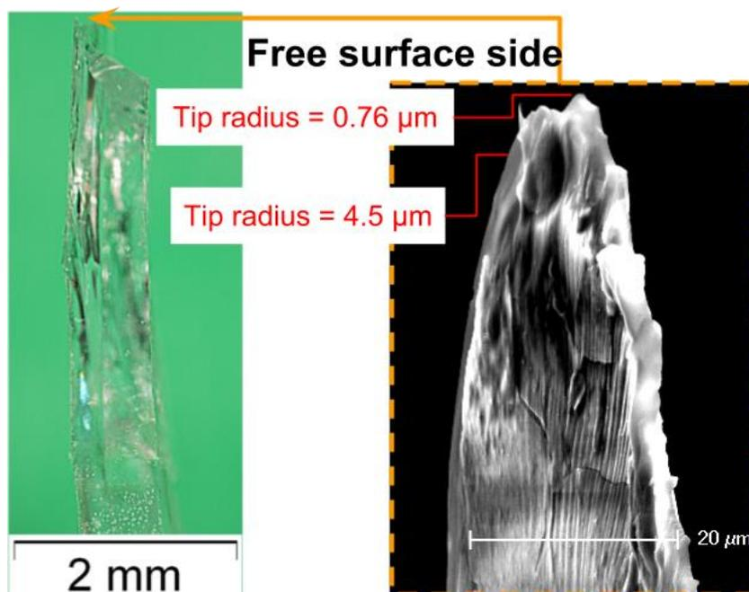
Figure 7.17 – Optical and scanning electron micrographs of a tip of a free surface profile of a low temper rectangular sample. Optically measured tip radius was 6.1  $\mu\text{m}$ .
