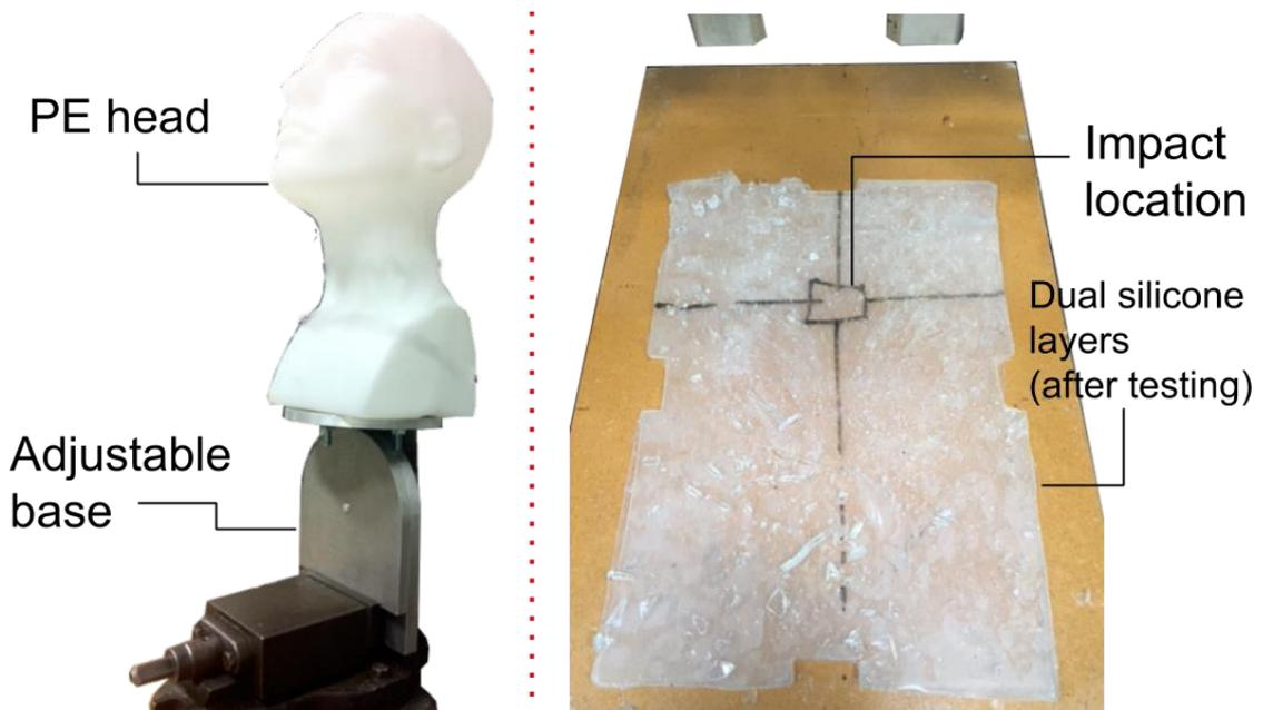
**Figure 5.11 – Targets used in drop tower testing. Left – polyethylene mannequin head on adjustable base; right – silicone layers (layer 1: ~1 mm thick layer of 10A Shore hardness, layer 2: ~2 mm thick layer of ~55A Shore hardness) together on a wooden platform after a test run with an annealed pint glass, showing debris left on the layer.**
