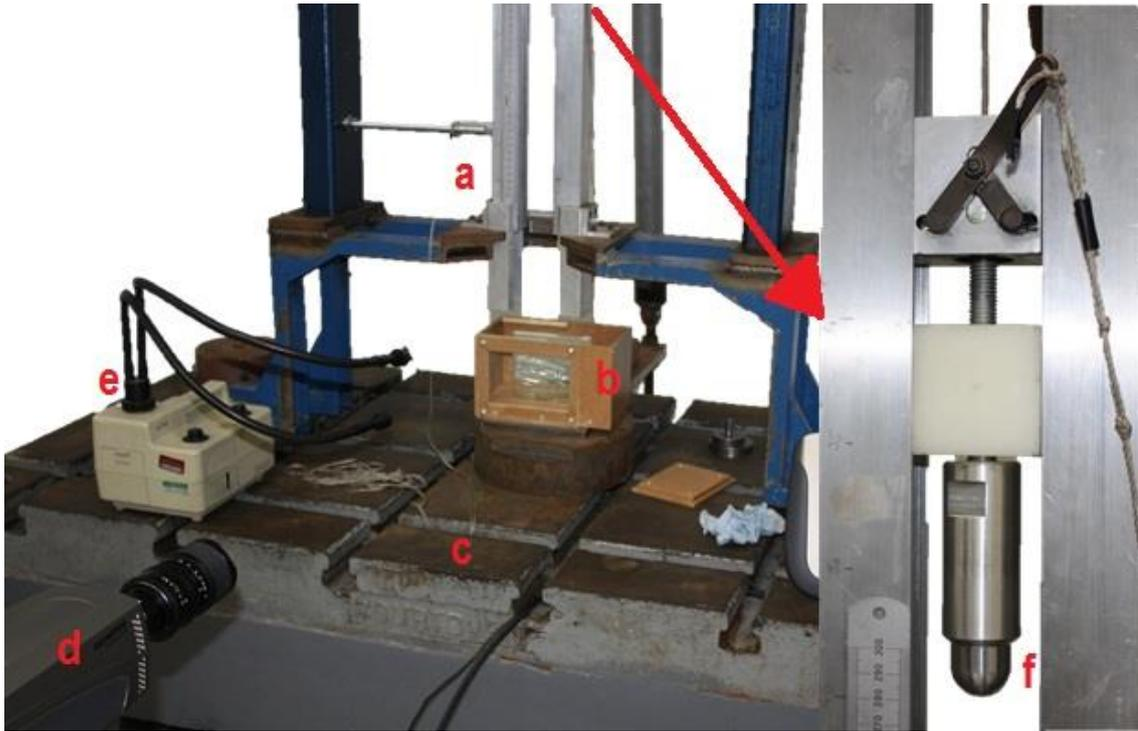
Figure 3.18 – Apparatus used for systematic impact testing. a: Drop tower guide rails extending beyond the top of the picture to a maximum height of 3.5m. b: Glass securing box. c: Cast iron table. d: High speed video camera. e: Light source. f: Enlarged picture of steel impactor from higher up the guide rails.
