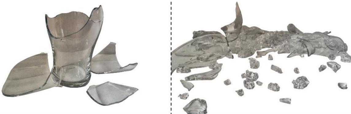
**Figure 1.1 – Typical fracture of annealed (left) and tempered (right) pint glasses.**
