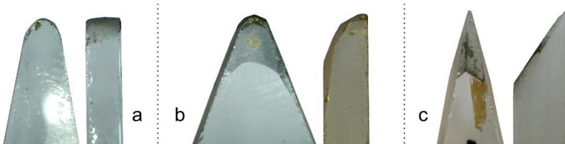
**Figure 6.20 – Examples of three machined glass fragments used in DOE penetration tests. For each, the free surface profile is shown on the left, and the x-axis edge profile on the right. a: inc. ang.: 20°, tip rad.: 1 mm, thickness: 2 mm, x-profile: wedge. b: inc. ang.: 40°, tip rad.: 1 mm, thickness: 3 mm, x-profile: rounded edge. c: inc. ang.: 20°, tip rad.: 0.1 mm, thickness: 4 mm, x-profile: sloped edge.**
