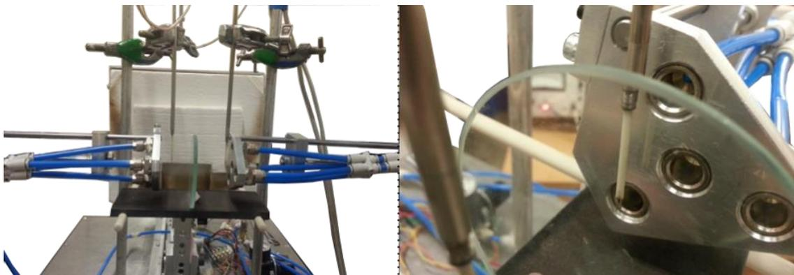
Figure A.1 – Hot wire anemometer setup. Left – anemometers set up to simultaneously take measurements from opposite ports of the jet arrays, right – the position of a single anemometer set up centrally in front of a port.
