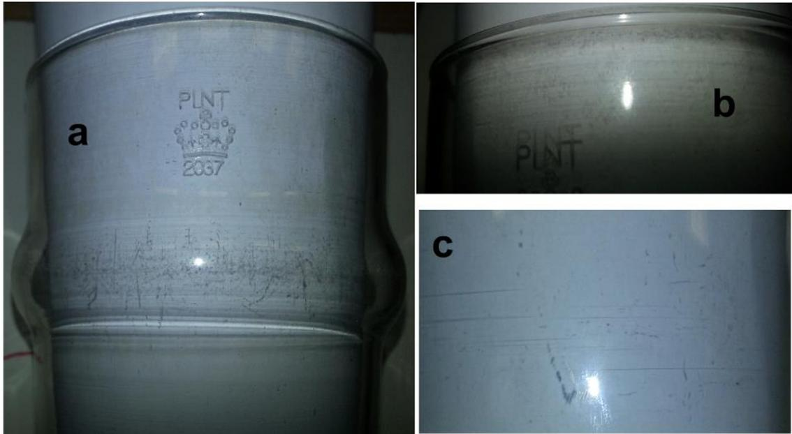
**Figure D.2 – Examples of surface damage on used pint glasses. a: damage in side-by-side contact area on a large-bulge Nonic glass; b: mottled damage below rim on a large-bulge Nonic glass, c: close-up view of side-by-side area damage on a Tulip glass.**
