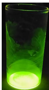
Figure 4.24: A potential dual-modal fluorescence/MR imaging probe \text{Tb}(\text{GdC8})_3 under a UV lamp at 300 nm.
