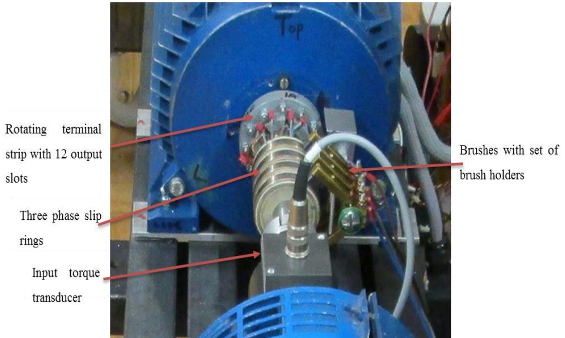
Figure 8.18: Section-A of the complete Lab. bench components
