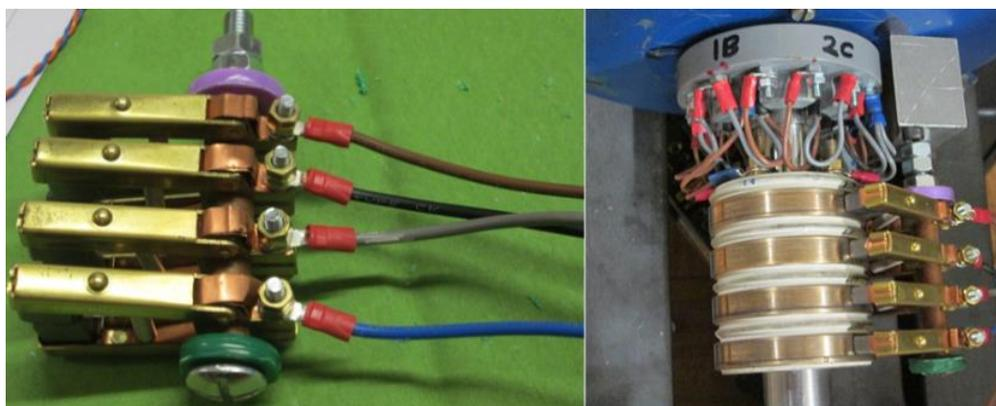
Figure 8.8: Slip rings and rotating terminal strip
