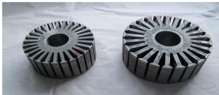
Figure 8.5: the lamination of (a) the inner rotor and the VFRT rotor
