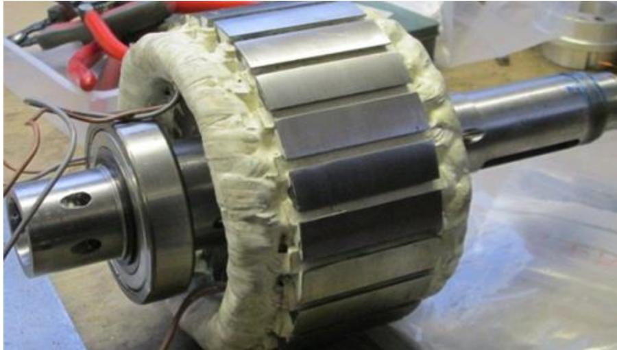
Figure 8.10: The rotor of the VFRT machine
