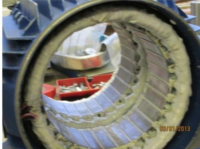
Figure 8.3: Twin stators fabricated in a single frame
