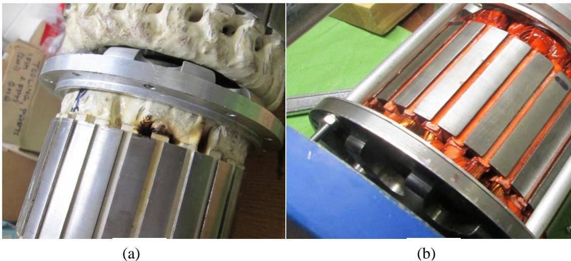
Figure F1.1: The inner rotor windings at (a) inter-turn short circuit and (b) after re-winded
