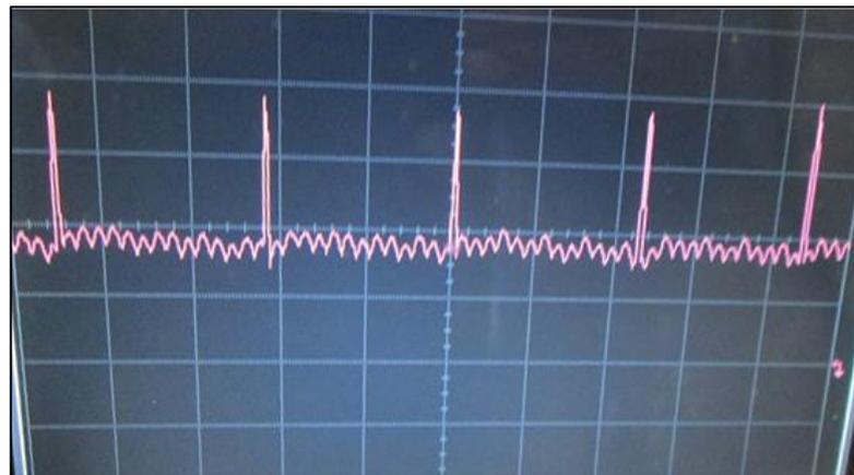
Figure 8.28: Commutation circuit noise with time switching at 20 ms/div and 1V/div
