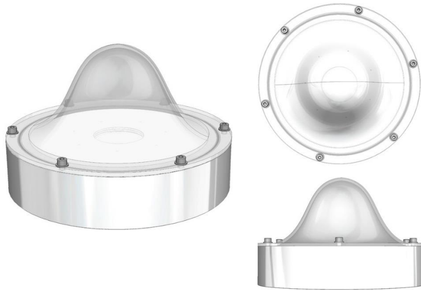
Figure 5.1: Sketch of the breast phantom showing, left, an isometric view and, right, a plane and side view.
