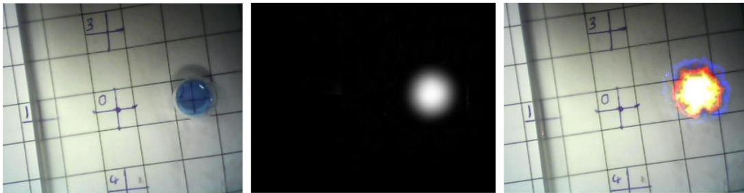
Figure 3.16: Example of superimposed gamma and optical image from a ^{99\text{m}}\text{Tc} (25 MBq) source. Imaging distance from collimator face was 80 mm and the acquisition time was 204 second. Optical image (left), gamma image (middle) and combined gamma and optical image (right).
