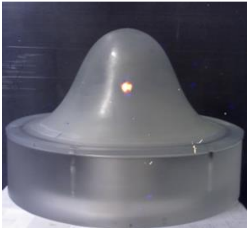
Figure 5.16: Superimposed gamma and optical images from a ^{57}\text{Co} source inside the breast phantom positioned at a distance of 43 mm beneath the surface (lateral view). The imaging distance was 100 mm to the side of the phantom (lateral view).
