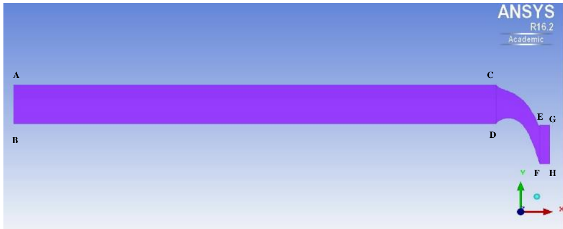
Figure 4-9: Cylindrical hub surface of the stator 1 half-stage rendered as a composite of three s(u, v) parametrised surfaces imported in ICEM CFD as a composite of three NURBS surfaces.
