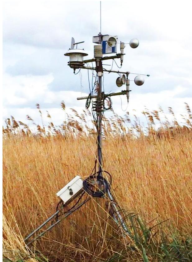
**Figure 20:** Setup of the AWS at Sedge Fen with the relative humidity and temperature probe, two cup anemometers and radiation sensor, white weatherproof boxes house datalogger and instrument control units (© G. Pan).
