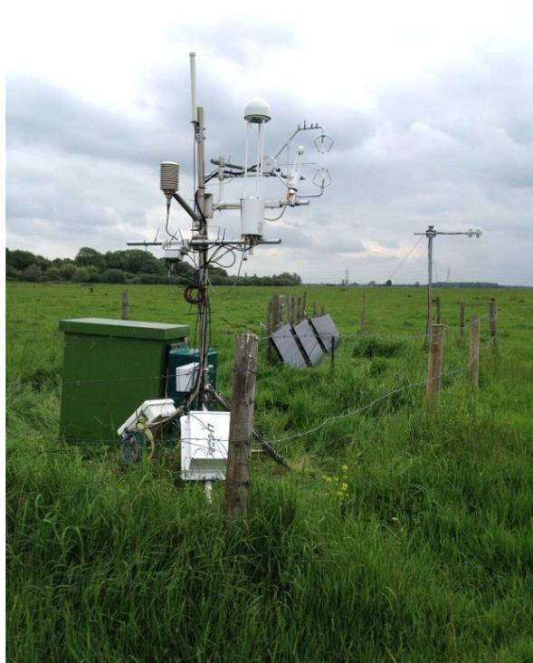
**Figure 18:** Setup of the EC station at Baker's Fen with sonic anemometer, the IRGAs, radiometers, relative humidity and temperature probe, solar panels and the power control system in the green box within a fence enclosure (© G. Pan).
