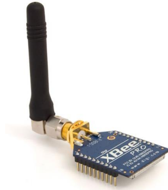
Figure 3- 5: Xbee 802.15.4 PRO with RPSMA connector and whip antenna.
