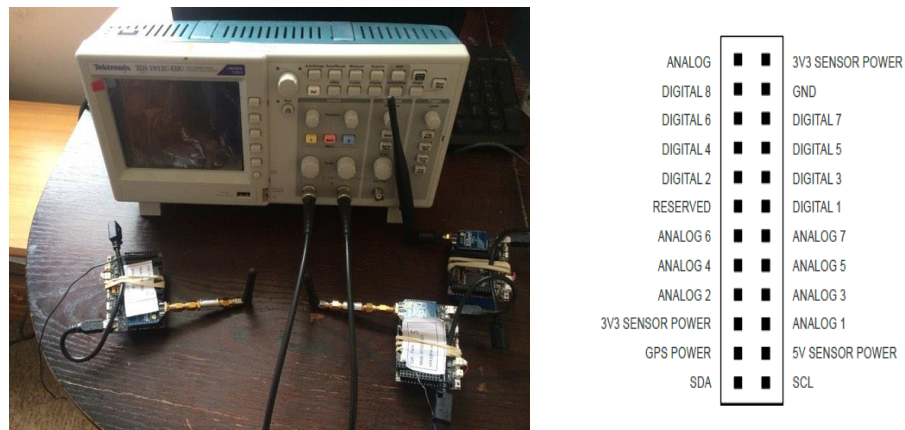
Figure 3- 29: (left) Testbed used to test the difference between RTC of the synchronized Waspnote nodes, (right) Description of sensor connector pins.
