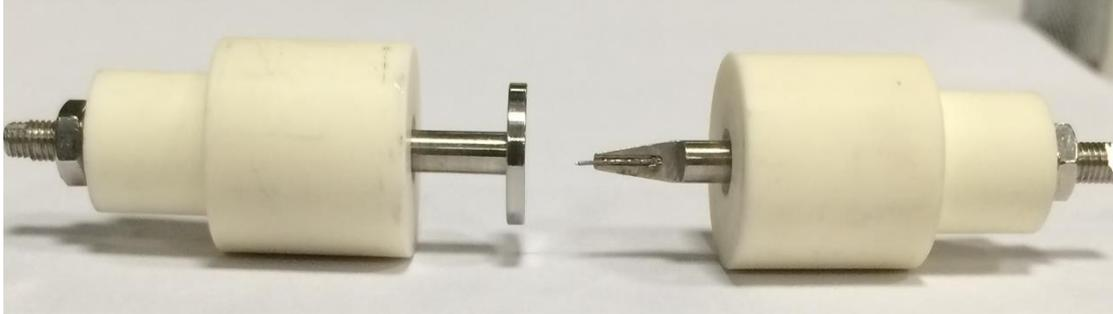
Figure 3.9: Image of Macor ceramic piece holding the tip-plane electrodes that are sealed with indium (indium does not appear in the image, and the Macor (the only item in the cell was bought from external company not built by the university).
