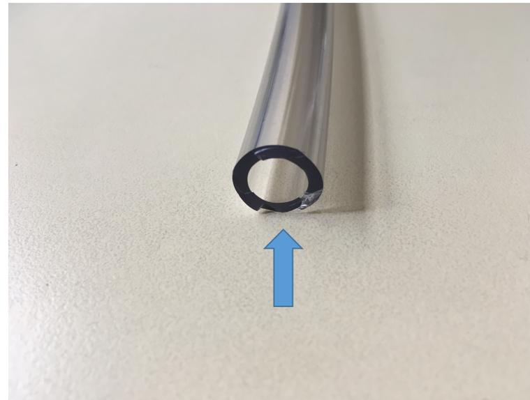
Figure 3 – The Bespoke Aortic Cannula, complete with a 'cuff' (3A) which reduced the risk of proximal slippage within the aorta following suture ligation. The 'bevelled' distal end aimed to improve laminar flow and thus minimise the risk of graft thrombosis (3B).
