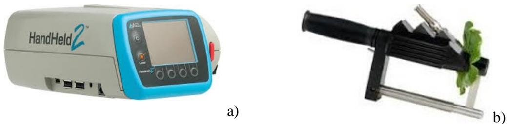
**Figure 3.10.** a) ASD HandHeld 2 spectrophotometer, b) plant probe + leaf clip
