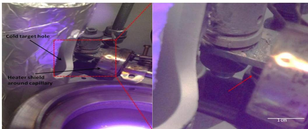
Figure 2-3. The picture on the left shows the cold trap, the liquid jet, the capillary heater and the sputter target (clockwise) giving an idea of distance between capillary and cold target. The dotted rectangle marks the region of the liquid jet and shown as zoomed picture on the right. The red arrow points onto the liquid jet which is collimated for at least 2 cm.
