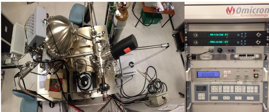
Figure A.2-1. Left: Top view of the XPS spectrometer. Right: Ion gauge controllers showing the pressures of the different chambers.
