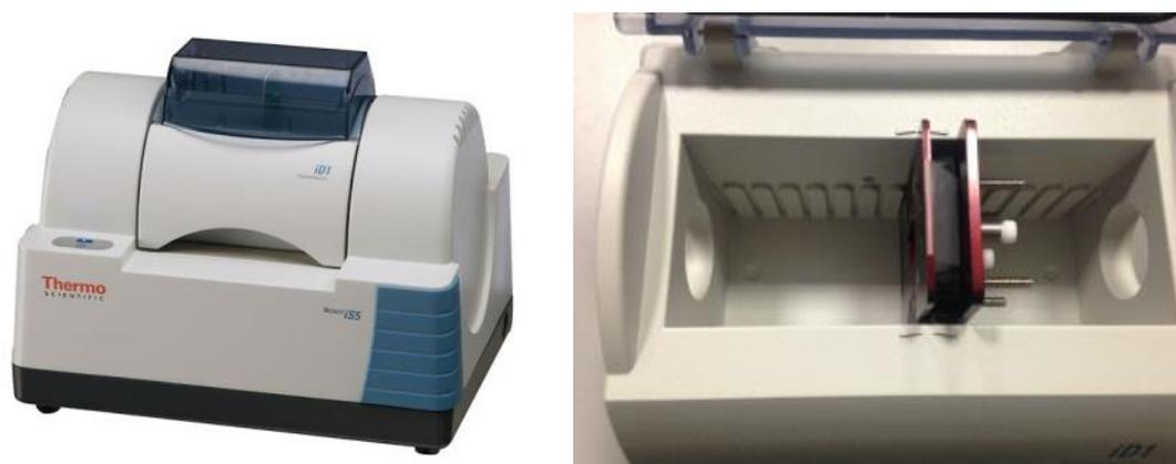
Figure A.3-2. The iD1 transmission accessory. Left, the device has been installed in an iS5 spectrometer, to measure transmission spectra. The position of the liquid cell in the transmission accessory is shown in the picture on the right.
