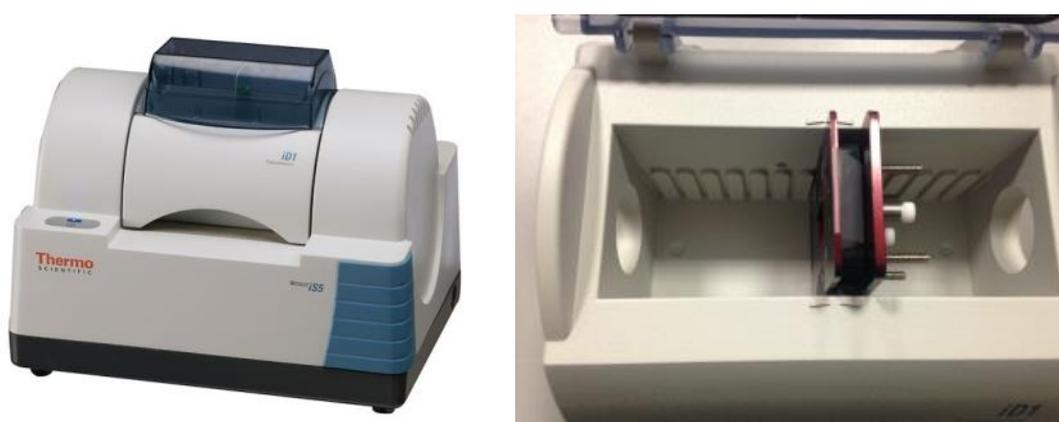
Figure A.3-2. The iD1 transmission accessory. Left, the device has been installed in an iS5 spectrometer, to measure transmission spectra. The position of the liquid cell in the transmission accessory is shown in the picture on the right.
