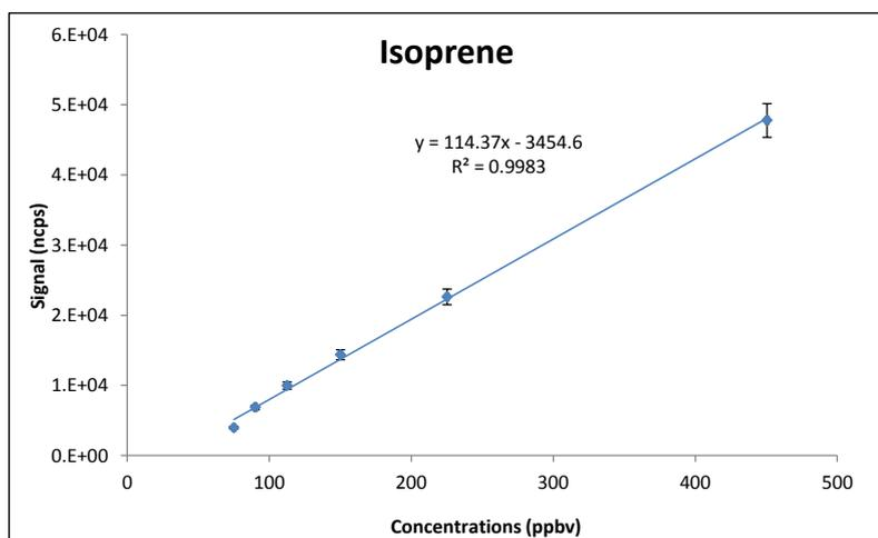
Figure 2.11 Calibration plots signal vs. concentration for protonated formaldehyde and isoprene at 1-minute integration times and  $E/N$  of 80/170 Td (0% RH).
