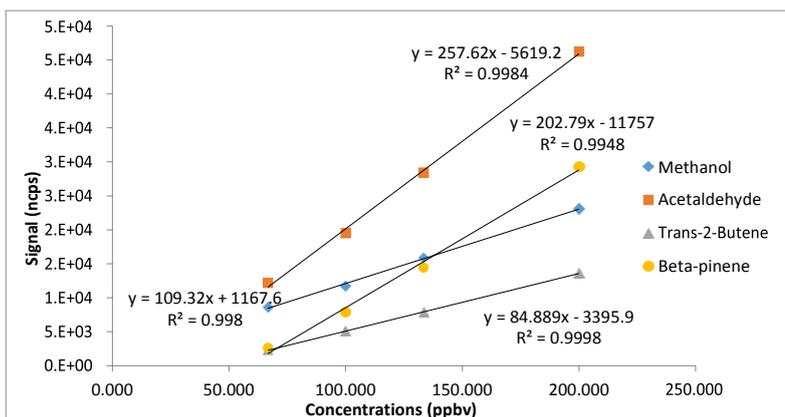
Figure 2.9 Calibration plots signal vs. concentration for protonated methanol, acetaldehyde, trans-2-butene and  $\beta$ -pinene at 1-minute integration times and  $E/N$  of 90/190 Td (0% RH).
