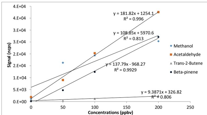
Figure 2.13 Calibration plots signal vs. concentration for protonated methanol, acetaldehyde, trans-2-butene and  $\beta$ -pinene at 1-minute integration times and  $E/N$  of 80/170 Td (0% RH).
