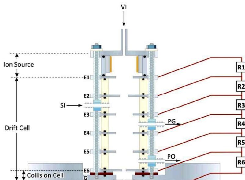
Figure 2.4 A schematic diagram of the drift tube. E1 – E6 represents electrodes 1 – 6 and R1 – R6 represents resistors 1 – 6, of which R1 – R5 are fixed a 1 M $\Omega$  and R6 is variable between 0 – 1 M $\Omega$ . S1, V1, PG and PO refer to the sample and vapour inlets, pressure gauge and pump outlet respectively. The main drift cell region is located between E1 and E6 and the collision cell between E6 and ground (G); the two regions can be operated at different E/N values.
