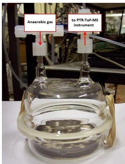
Figure 3.3 The glass container used for the headspace analysis of bacteria cultures.
