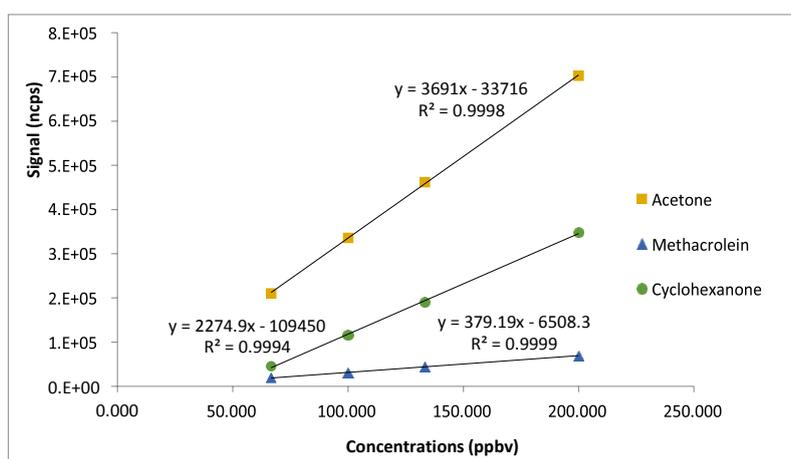
Figure 2.8 Calibration plots signal vs. concentration for protonated acetone, methacrolein, and cyclohexanone at 1-minute integration times and  $E/N$  of 90/190 Td (0% RH).
