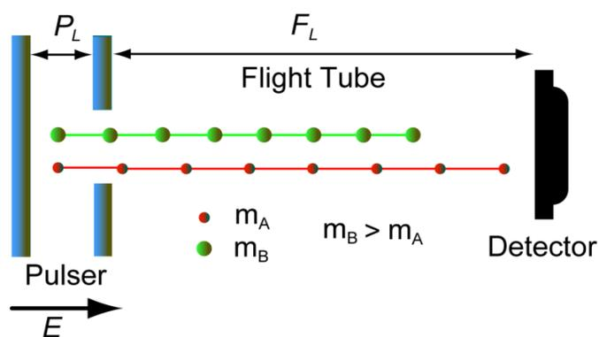
Figure 2.1 Diagram to show the basic components and principles of a linear ToF-MS system (adapted from Wyche (2008) [8]).
