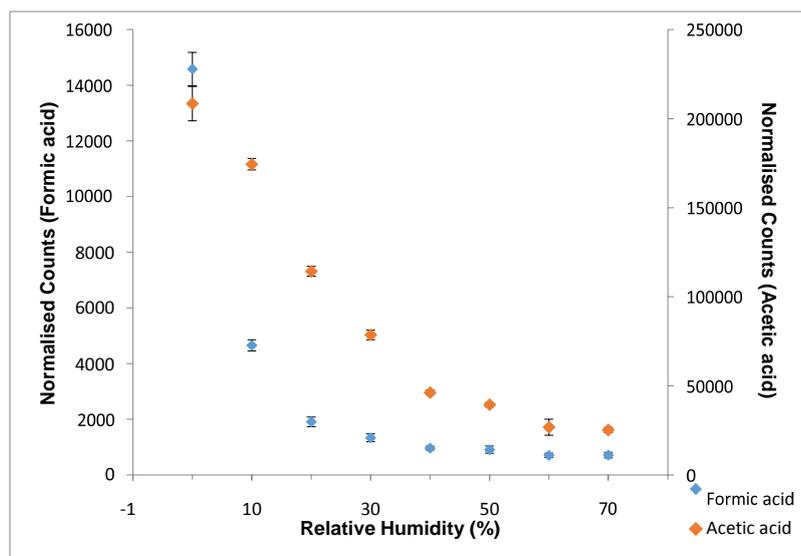
Figure 2.14 The change in the abundance of acetic acid and formic acid in normalised counts as a function of sample humidity at an  $E/N$  of 80/170 Td. The error bars denote the standard deviation calculated over the analysis time of 1 minutes.
