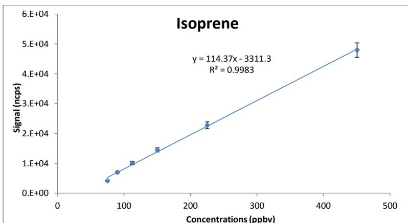
Figure 2.7: Calibration plots signal vs. concentration for protonated formaldehyde and isoprene at 1-minute integration times and  $E/N$  of 90/190 Td (0% RH).
