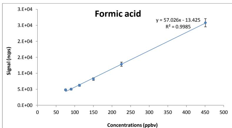
Figure 2.6: Calibration plots signal vs. concentration for protonated acetic acid and formic acid at 1-minute integration times and  $E/N$  of 90/190 Td (0% RH).
