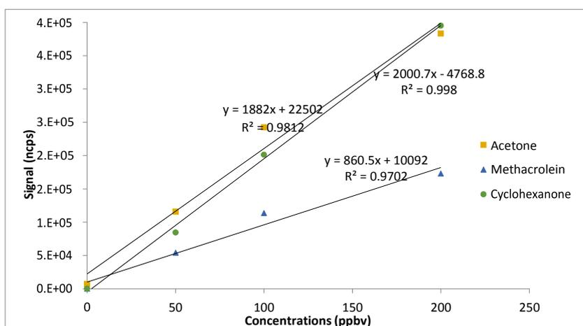
Figure 2.12 Calibration plots signal vs. concentration for protonated acetone, methacrolein, and cyclohexanone at 1-minute integration times and  $E/N$  of 80/170 Td (0% RH).
