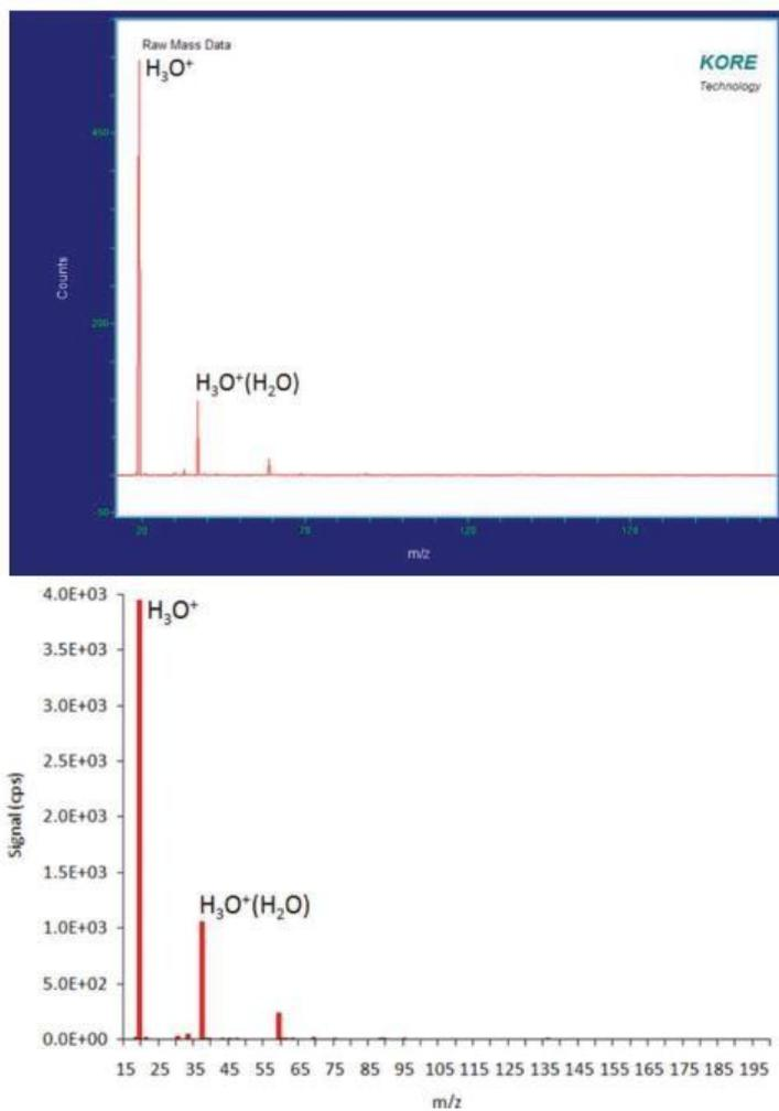
Figure 2.5 Comparison of raw (top) and processed (bottom) PTR-TOF-MS mass spectrum [9].
