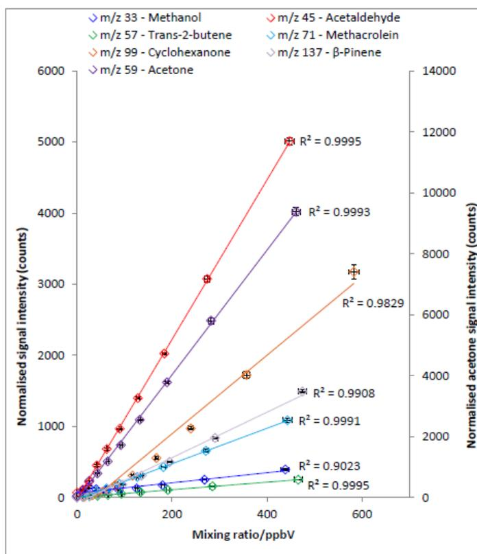
Figure 2.15 Multi-point calibration showing the normalised sensitivities for a seven-component VOC gas standard. The data was collected in the RF mode. The sensitivity is linear over dynamic range of at least three orders of magnitude [14].
