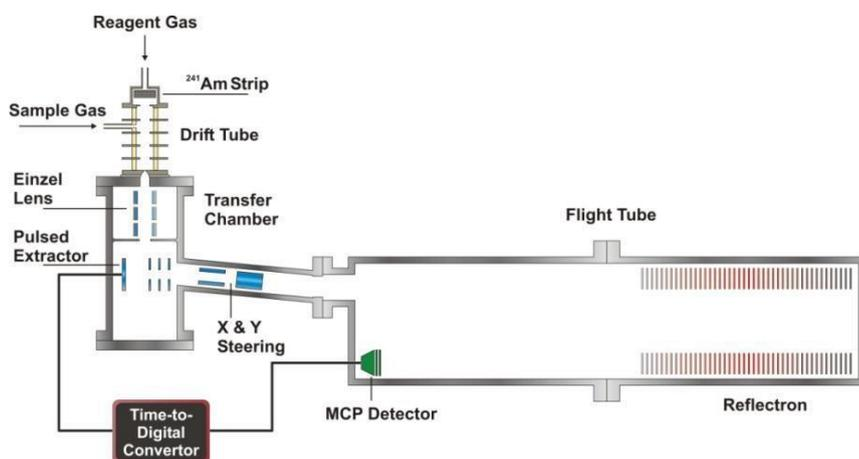
Figure 2.3: The schematic diagram of PTR-TOF-MS instrument
