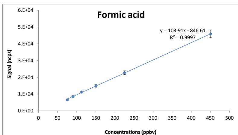
Figure 2.10 Calibration plots signal vs. concentration for protonated acetic acid and formic acid at 1-minute integration times and  $E/N$  of 80/170 Td (0% RH).
