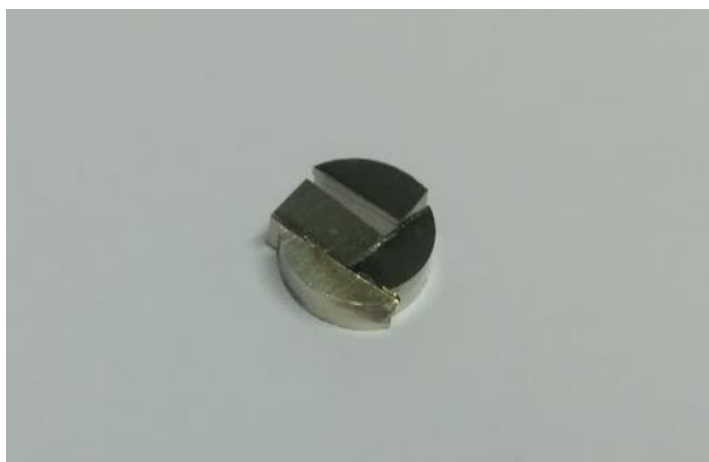
Fig. 6.6 Fragments of a cross-sectional slice (Ni 2 Cr 12 Al) prepared for KEMS experiments
