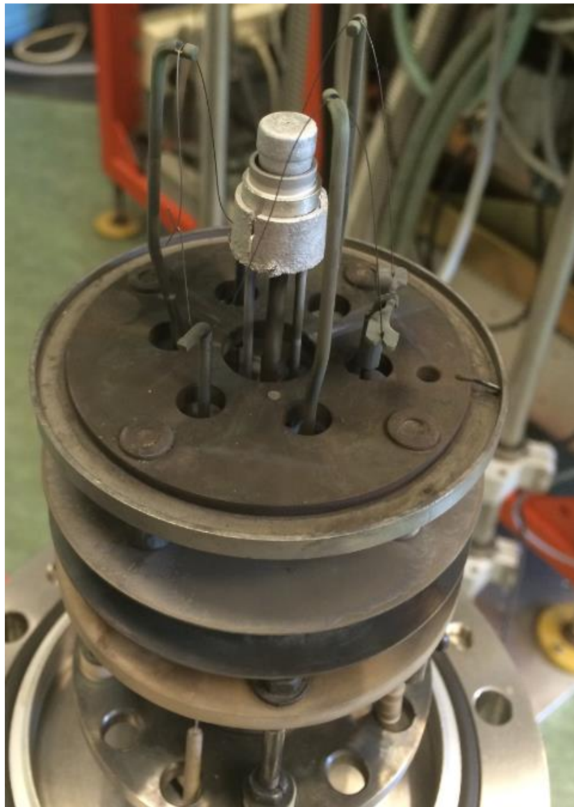
Fig. 3.3 Ir Knudsen cell used in KEMS facilities at Forschungszentrum Jülich
