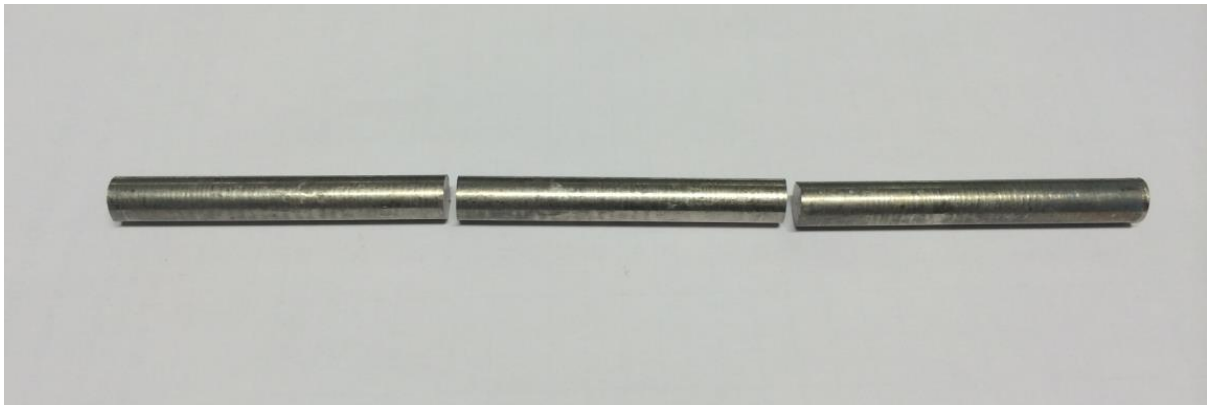
Fig. 5.4 A sample of as-cast Ni 2 Cr 5 Al model alloy
