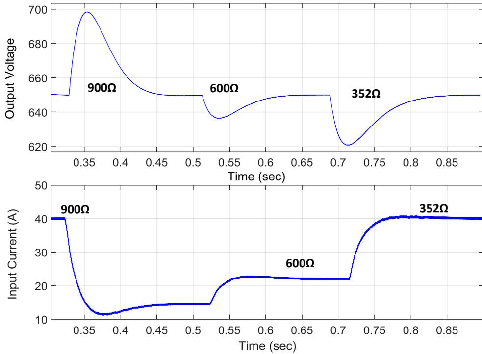
Fig. 4.17 Step response to load changes using physical model
