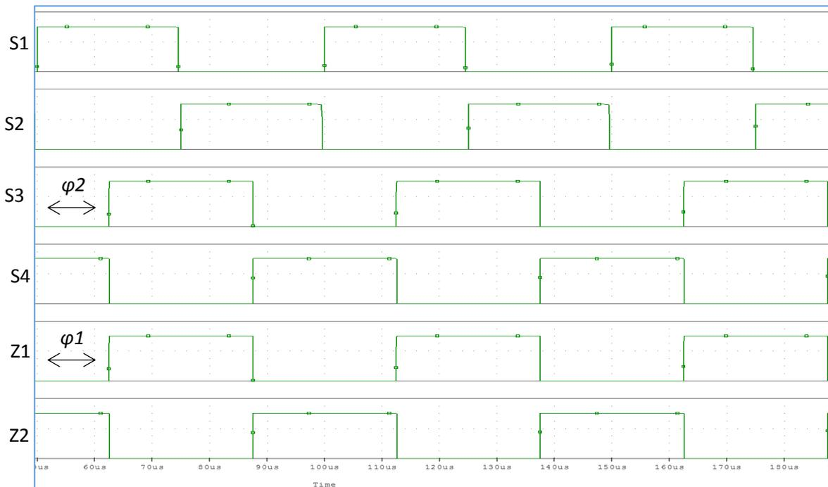
Fig.5.3. VFC timing pulses with 50% duty ratio
