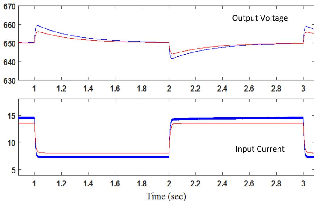
Fig. 4.16 Step response to load changes; red: transfer function model; blue: physical model
