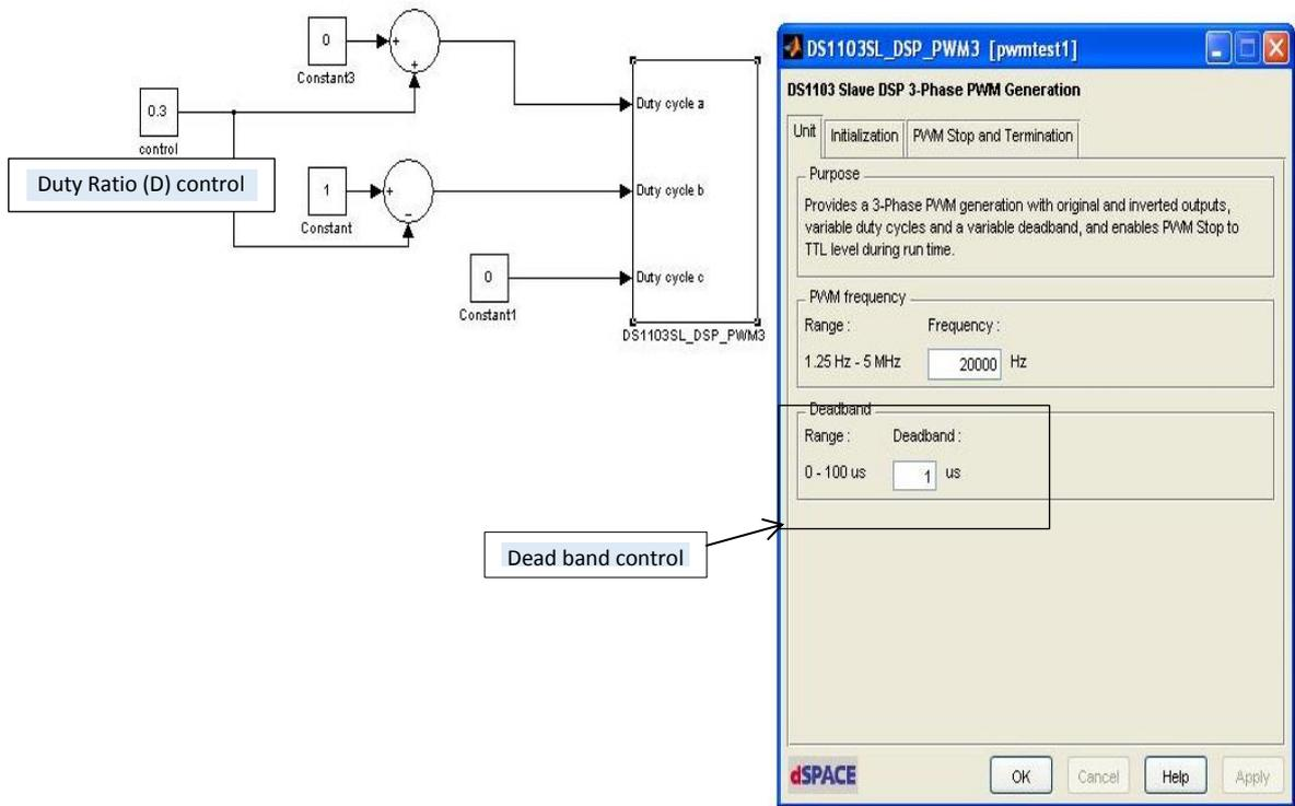
Fig.3.16 Bridge & active clamp pulses design using DS1103SL\_DSP\_PWM3 block
