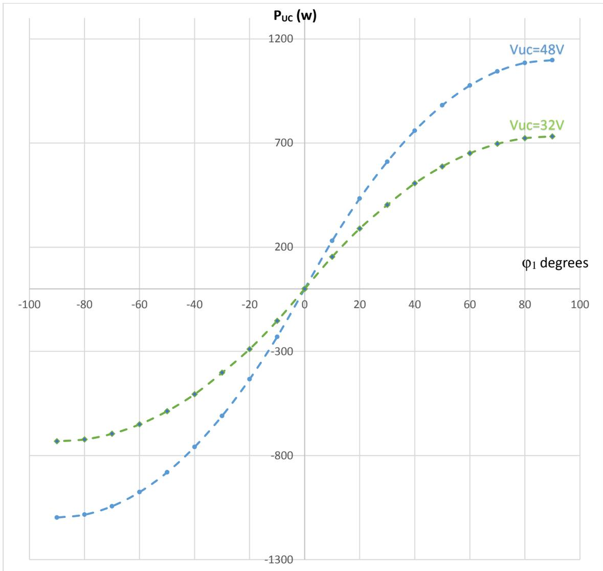
Fig.5.28 Input power for both power flow direction, ( $L_t=10\mu H$ ,  $n=7.4$ ,  $V_o=650v$ , and  $f_s=20$  kHz)
