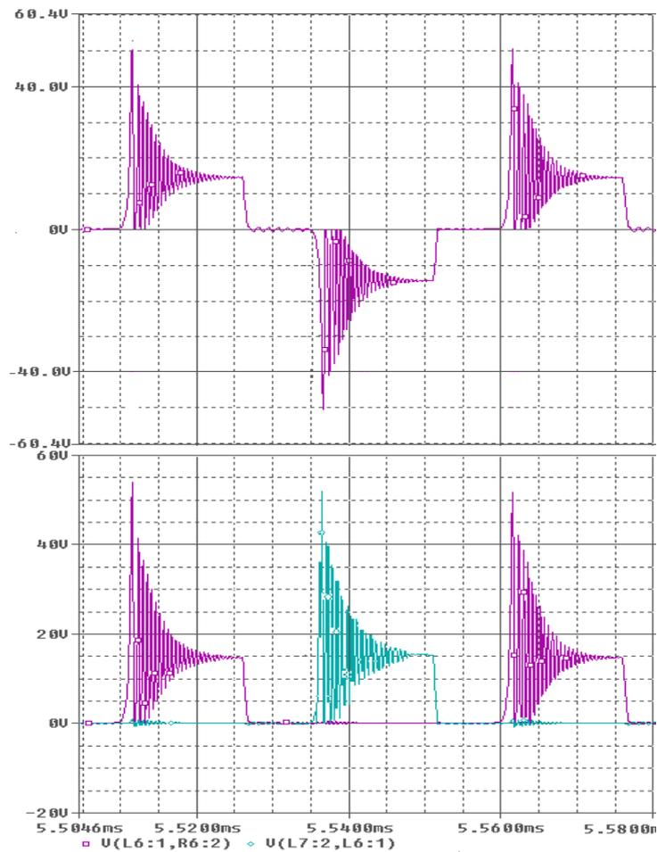
Fig.3.6 From the top: primary winding voltage, and voltages across the switches with super imposed ringing; frequency approx. 1.75 MHz
