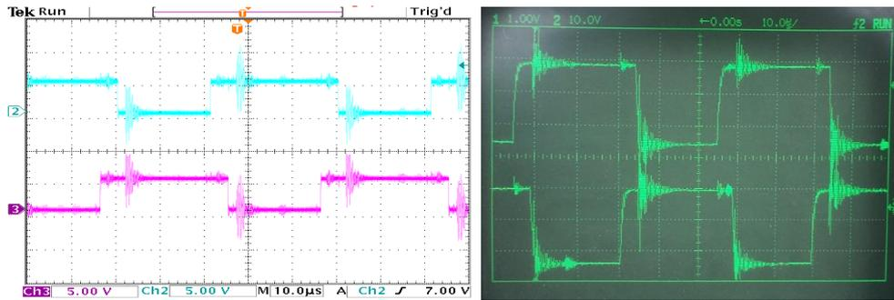
Fig. 3.22 (a) Switches drivers inputs (dSPACE output), (b) photograph for switches drivers output (gates pulses)
