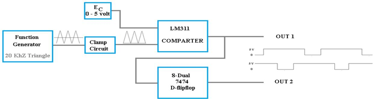
Fig.3.12 Block diagram for creating overlapping pulses
