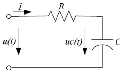
Fig. 2.18 Ultra-capacitor equivalent circuit [86]
