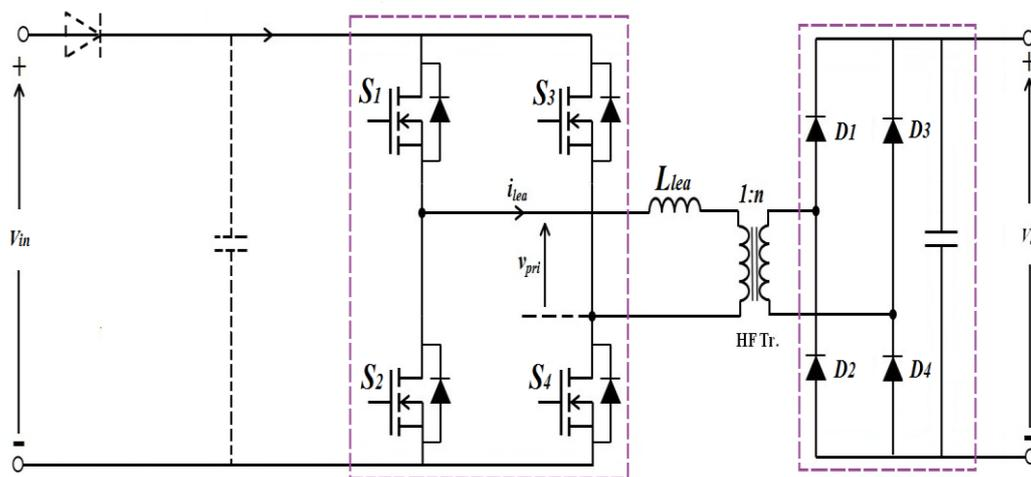
Fig.2.12 Typical topology of a voltage-fed DC-DC converter.
