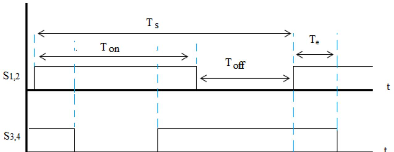
Fig. 3.2 Overlapping timing pulses
