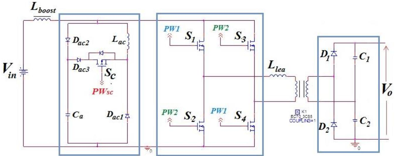
Fig. 3.35 Improved Modified active clamp circuit with series diode  $D_{ac3}$
