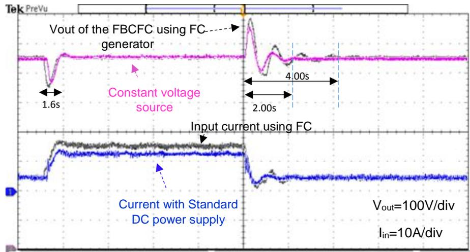
Fig.4.24 Time response for both the FC and the constant voltage source
