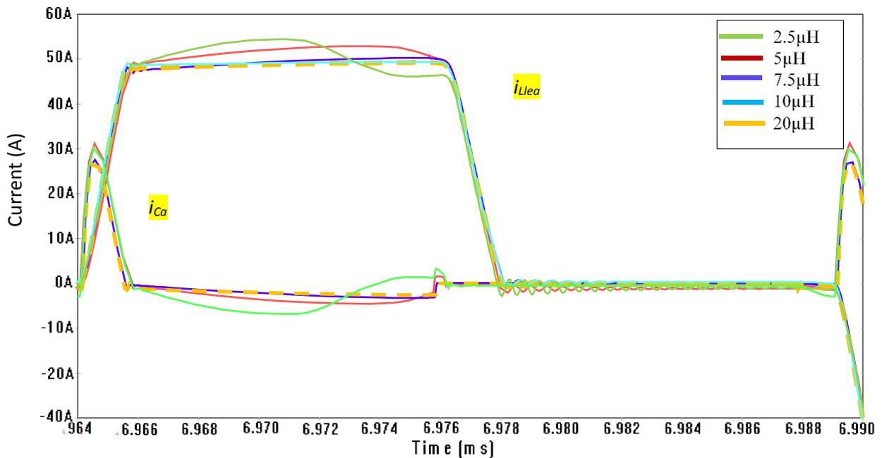
Fig.3.39 Bridge current  $i_{Llea}$  and the active clamp capacitor current  $i_{ca}$  with a different values of  $L_{ac}$
