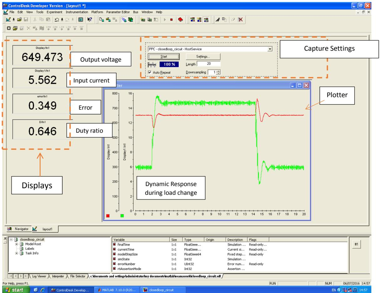
Fig.4.28 Control-Desk layout on the dSPACE PC
