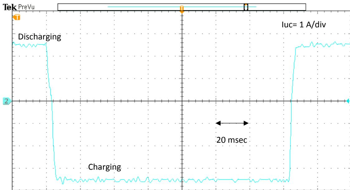
Fig.2.21 UC current during charging and discharging
