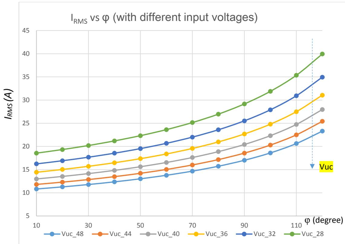
Fig.5.12 Relationship between  $I_{in\_RMS}$  and  $\phi_{outer}$  under CPC
