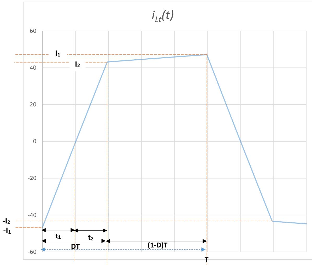
Fig.5.10 The primary winding current  $i_{L_t}$
