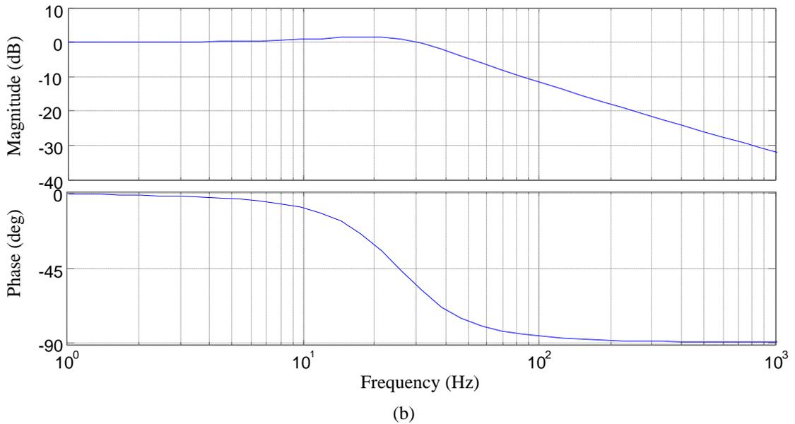
Fig. 4.6 Bode plots of the two transfer functions (a) Inner loop and (b) Outer loop
