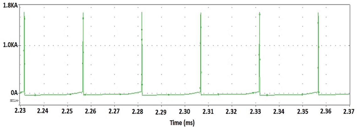
Fig.5.4. Input current spikes due to the zero-dead time
