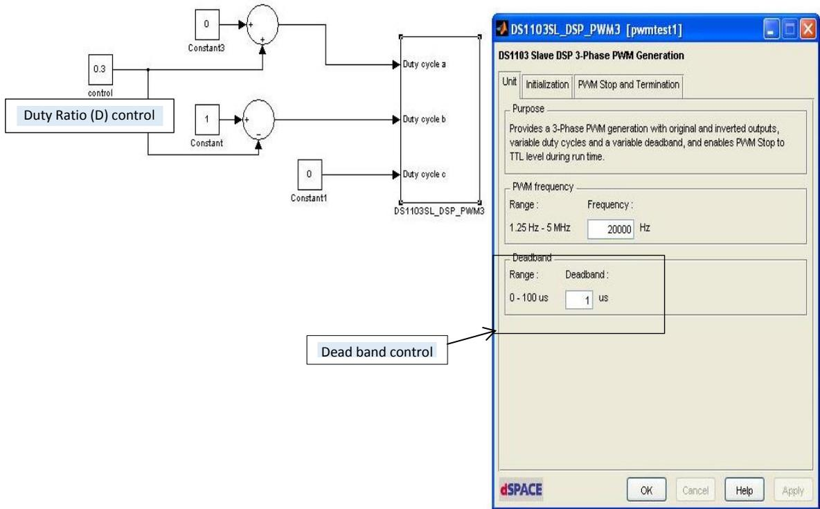
Fig.3.16 Bridge & active clamp pulses design using DS1103SL\_DSP\_PWM3 block
