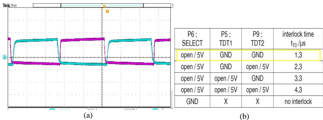
Fig.5.18 IGBTs timing signals and dead time selection
