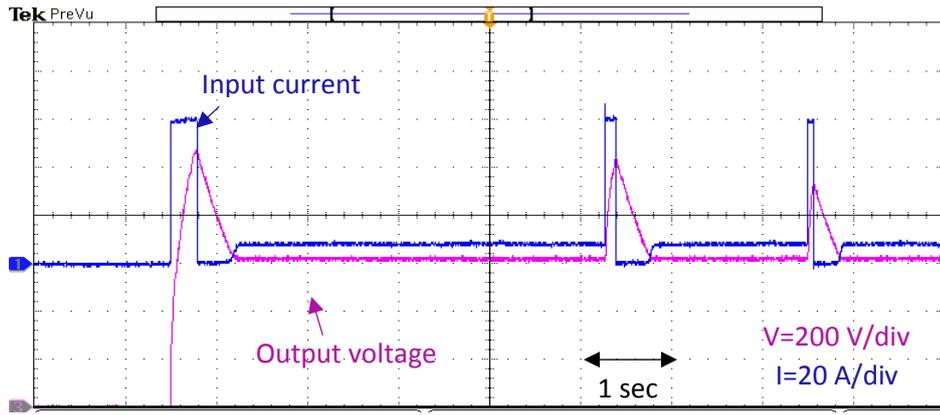
Fig. 4.11 Start-up test using a standard power supply with a current limiter (60 A) with the set gain values number (3) of the controller gains in Fig.4.10
