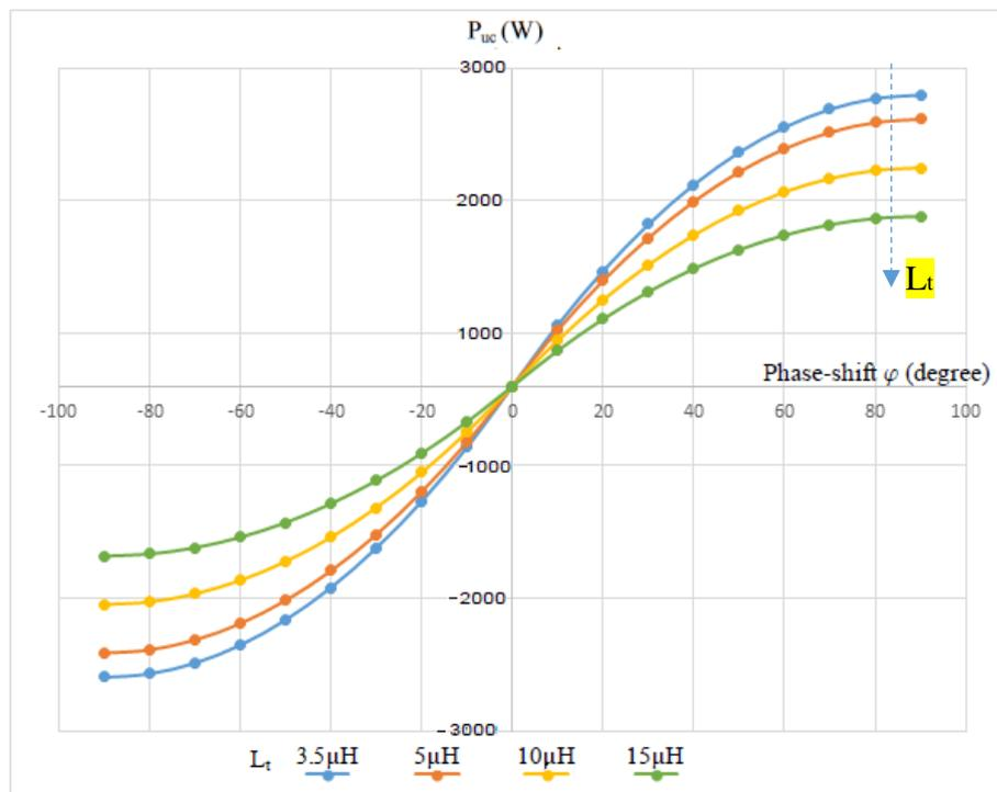
Fig. 5.13 Relationship between power and phase shift under various leakage inductance ( $V_{uc}=48\text{V}$ ,  $f_s=20\text{kHz}$ ,  $V_o=650\text{V}$ ,  $n=7.4$ )
