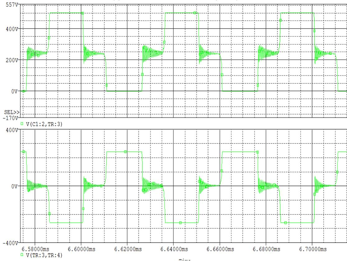
Fig3.8 From the top the voltage across the rectifier diode, and the secondary voltage
