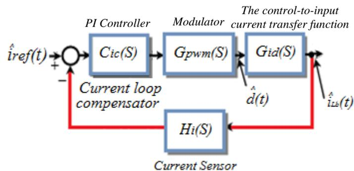
Fig. 4.3 Inner current control loop
