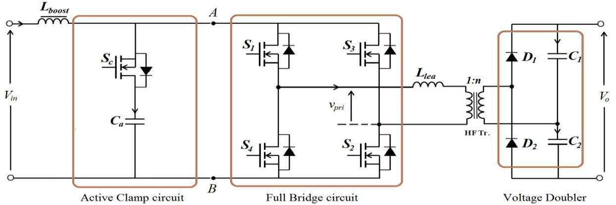
Fig.3.1 FBCFC with a regenerative clamp circuit
