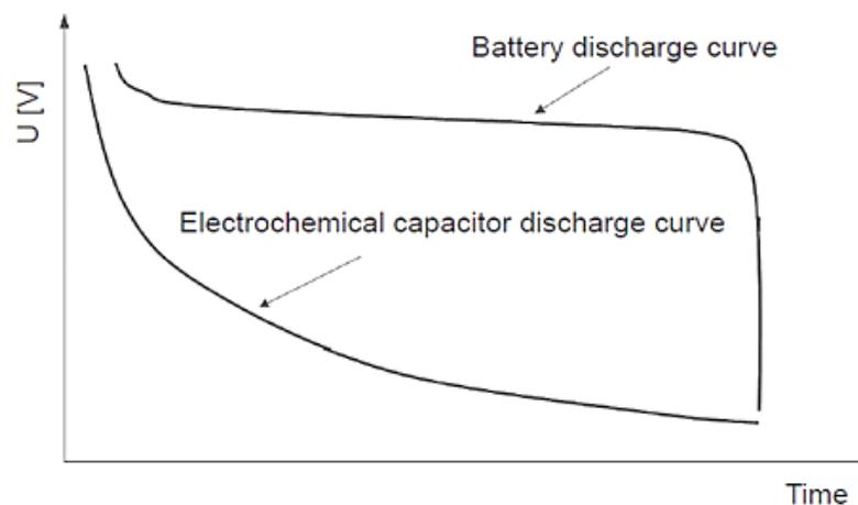
Fig. 1.4 Discharge curves of Electrochemical Capacitor and a Battery [42]
