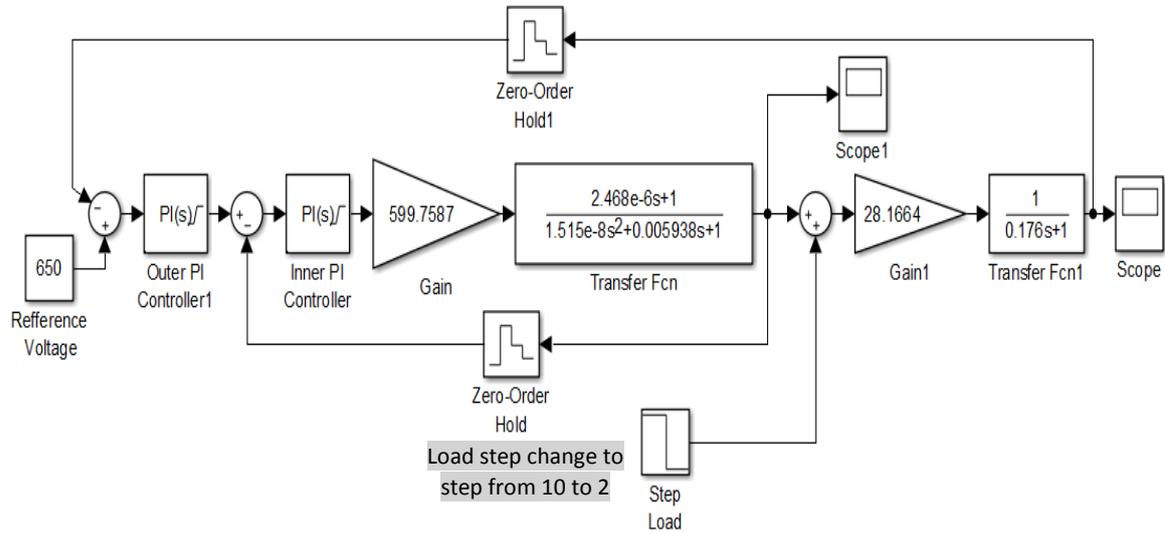
Fig. 4.8 Control block diagram of double-loop controller using Matlab Simulink
