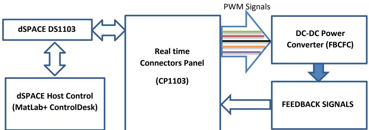
Fig.4.19 Block diagram of hardware setup
