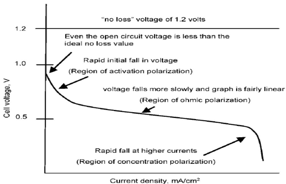
Fig.2.3 FC voltage-current characteristics [66, 67].
