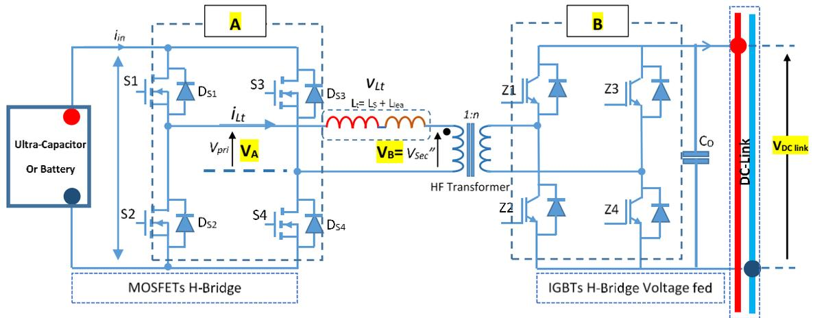
Fig. 2.24 Dual H–Bridge bidirectional converter
