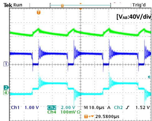
Fig.3.25 From the top: the boost current, bridge voltage, primary winding voltage when using the active clamp circuit with  $D=0.6$ .
