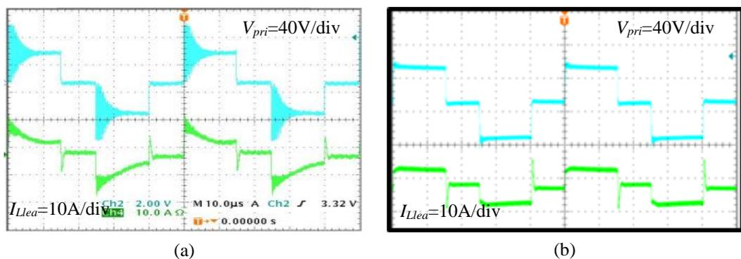
Fig. 3.43 Primary winding voltage (top) and current (bottom) at 15% of the full load for :a) CACC, b) IMACC
