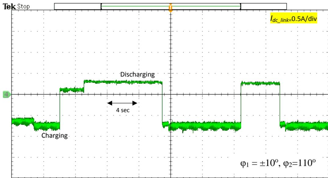
Fig.5.29 Current direction during charging and discharging of the batteries
