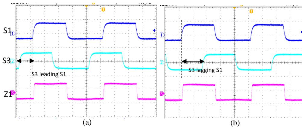
Fig.5.31 shows the firing pulses of the devices with: a) charging process, b) discharging
