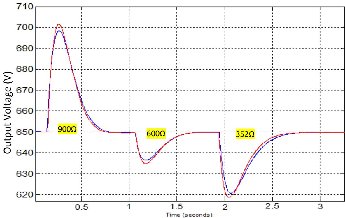
Fig.4.18 Time response comparison (the converter output voltage) between CACC (Red), and MACC (Blue) during different load change (352Ω (full load), 900Ω, 600Ω, 352Ω)
