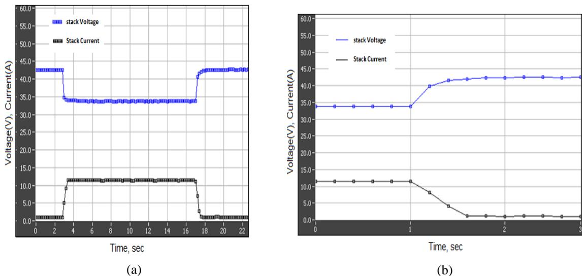
Fig.2.8 Measured transient response of Nexa FC Power Module using “Nexamon OEM” data log file
