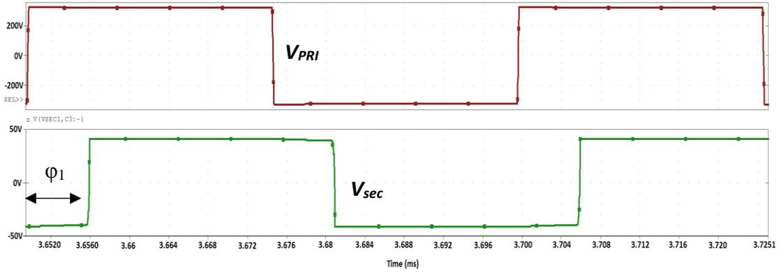
Fig.5.6 VFC voltages, from the top: primary voltage, secondary voltage
