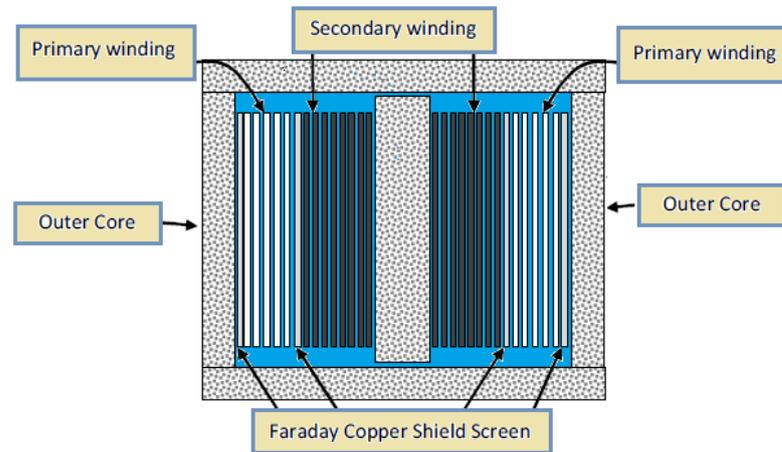
Fig. 3.27 Transformer-winding Modification
