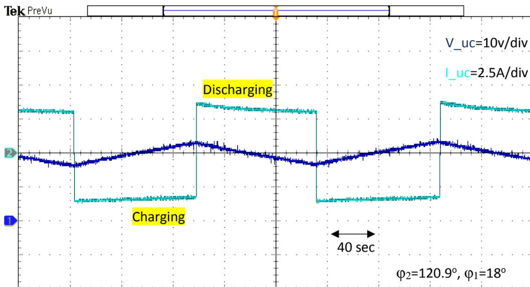
Fig.5.32 Ultra-capacitor voltage and current
