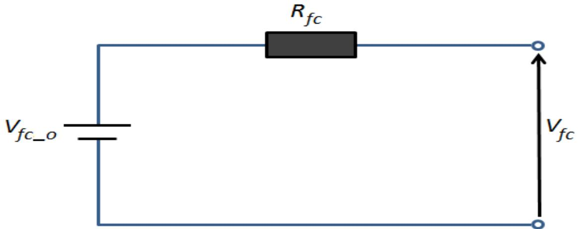
Fig.2.4 Simplified equivalent circuit of a FC
