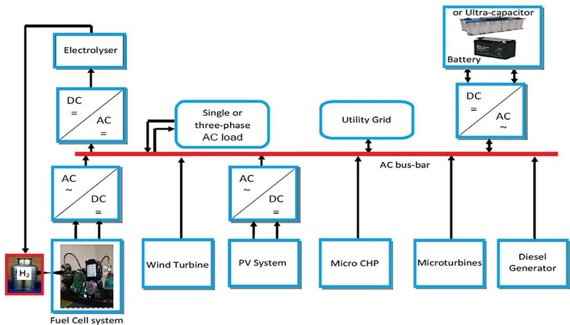
Fig. 1.2 AC micro-grid system configuration
