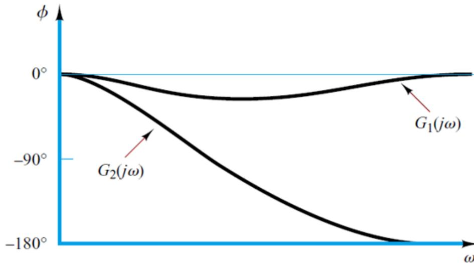
Fig.4.2 Phase-angle characteristics of the systems  $G_1(s)$  and  $G_2(s)$  shown in Fig.4.2
