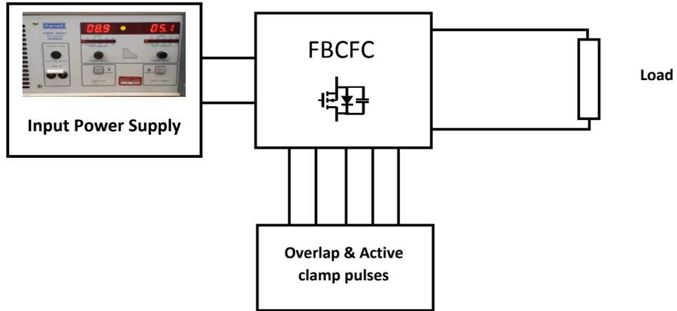
Fig. 3.20 A block diagram of the FBCFC setup
