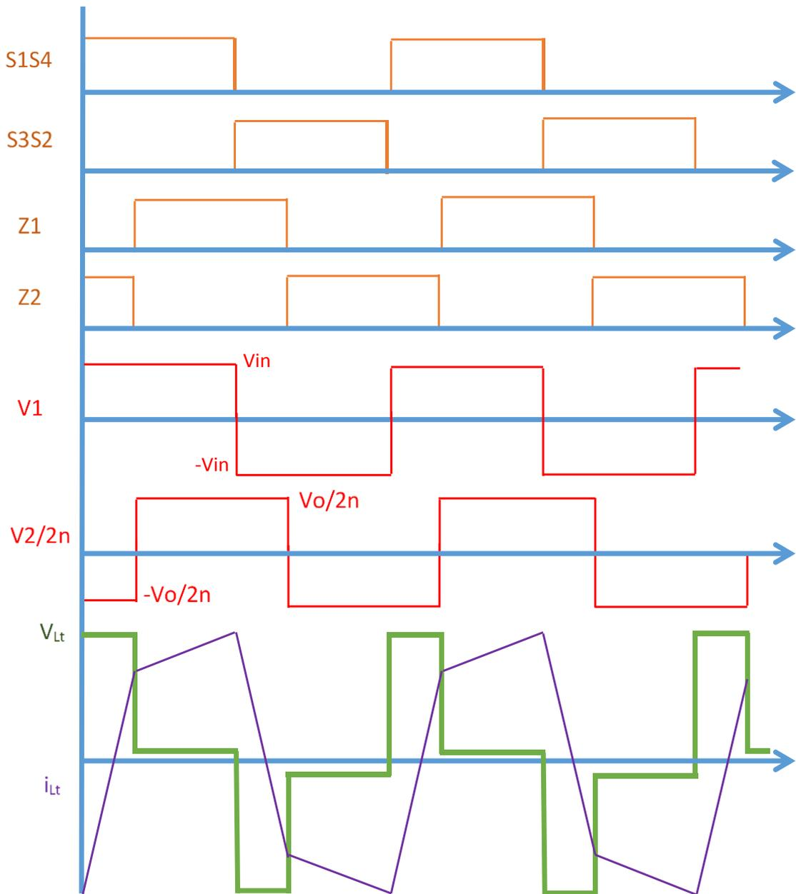
Fig.5.9 Main IBDC waveforms
