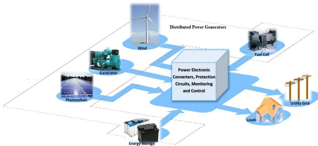
Fig.1.1 Parts of a typical micro-grid
