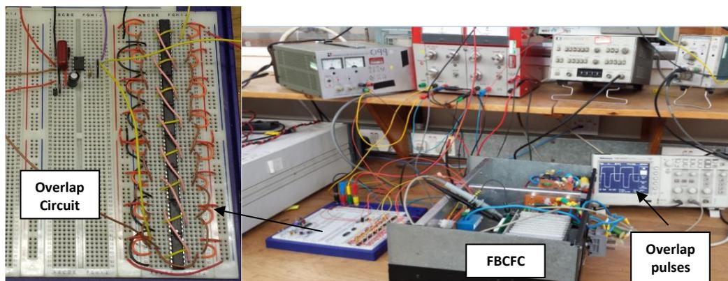
Fig.3.13 Photograph of overlap pulses circuit test on the FBCFC
