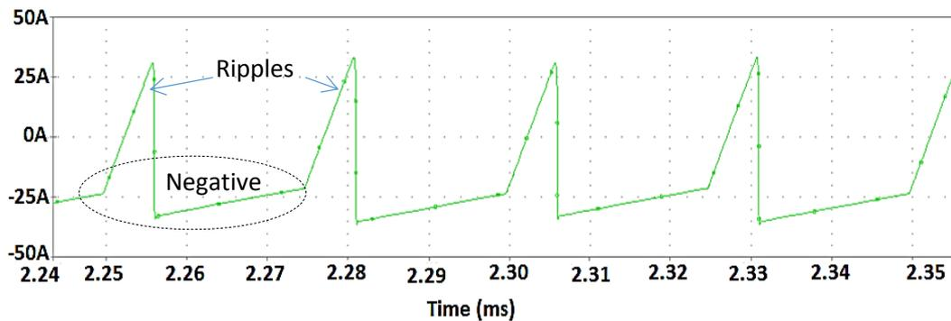
Fig.5.5 Input current due to 0.5  $\mu$ Sec dead time
