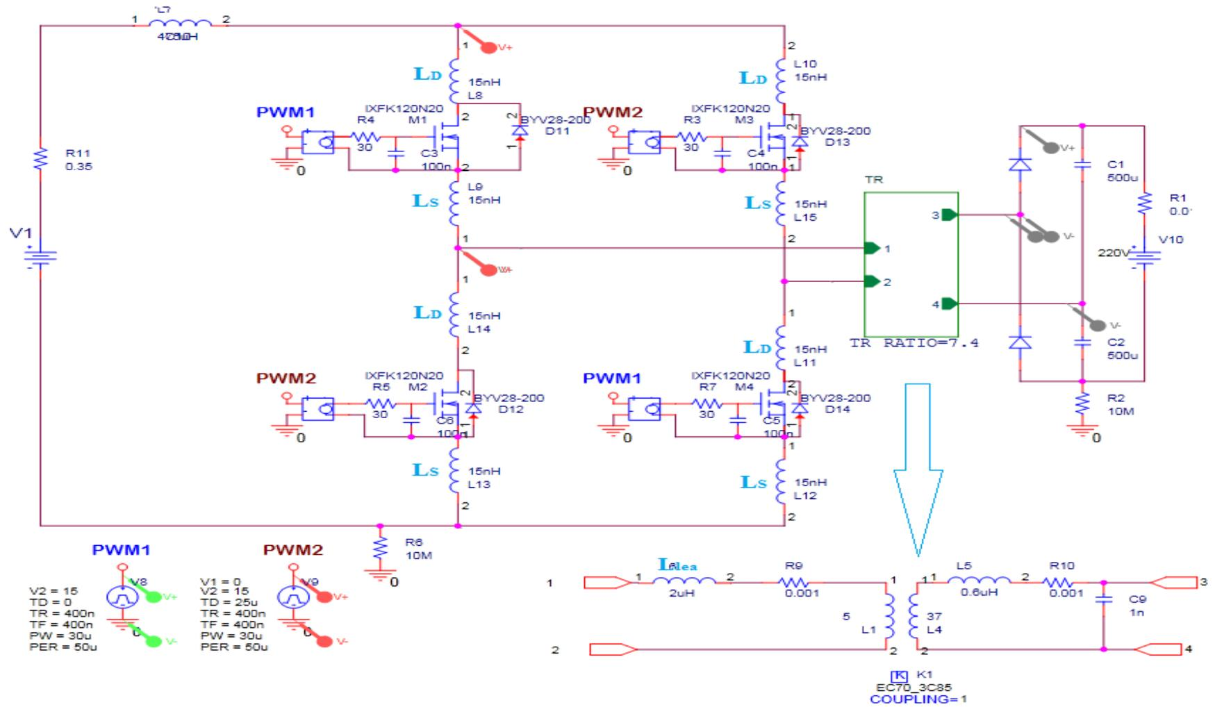
Fig. 3.5 The FBCFC model in PSPICE using non-ideal components
