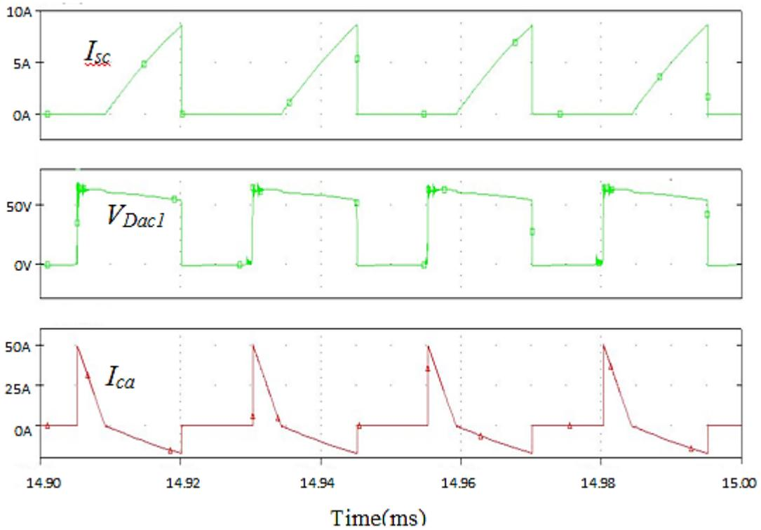
Fig. 3.36 Simulation results for the FBCFC with MACC; top: clamp switch current, middle: voltage across  $D_{ac1}$ , bottom: clamp capacitor current
