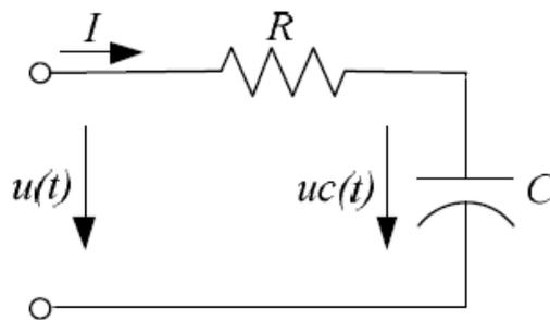
Fig. 2.18 Ultra-capacitor equivalent circuit [86]
