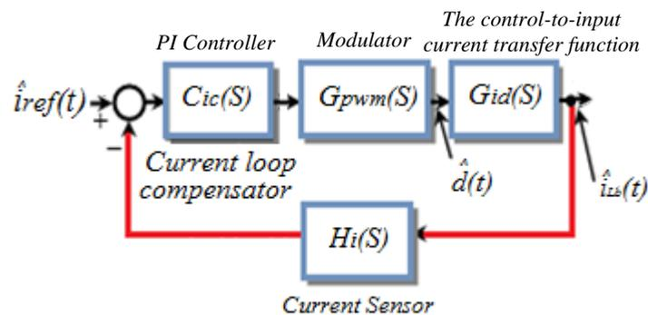
Fig. 4.3 Inner current control loop
