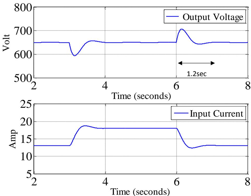
Fig. 4.9 Converter time response to load changes (applied after 3sec and removed after 6sec) using Matlab simulation of the system in Fig.4.5
