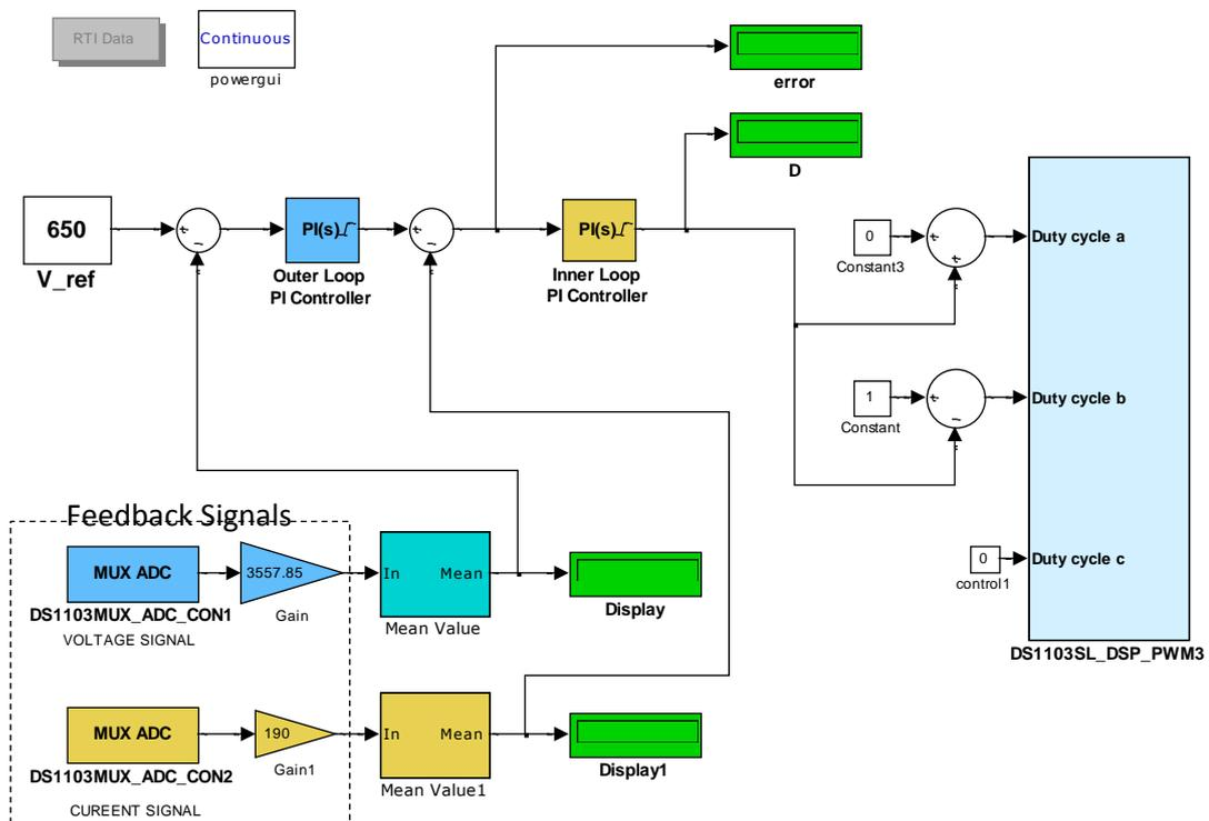
Fig.4.22 Controller Implementation using dSPACE
