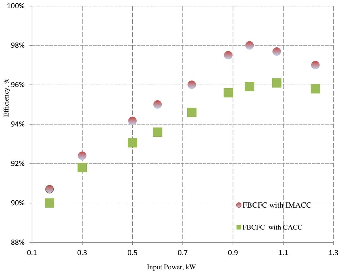
Fig. 3.37 Efficiency at constant input voltage (simulation)
