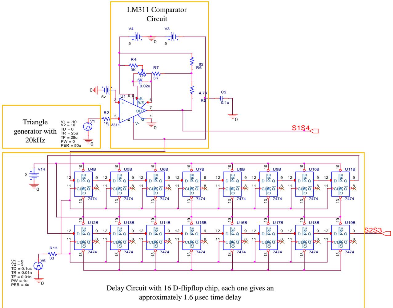
Fig. B. A circuit diagram for creating overlapping pulses for the FBCFC
