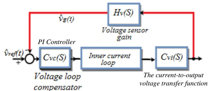
Fig.4.4 Voltage control loop using controller
