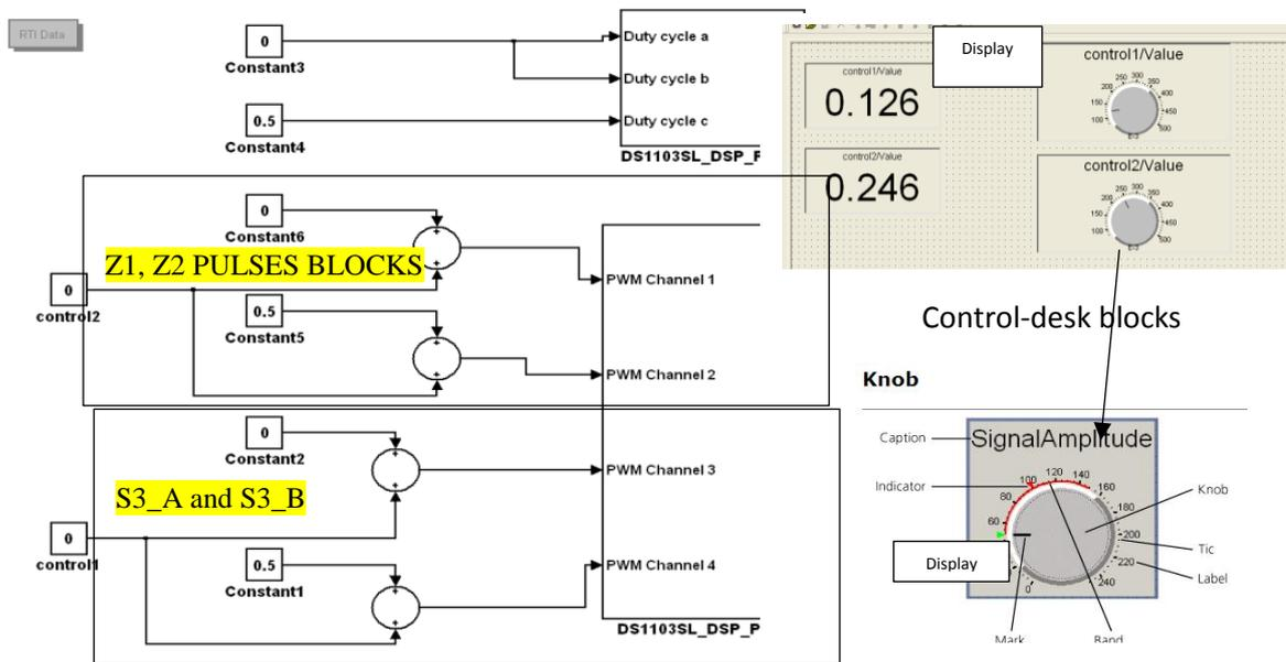
Fig.5.16 Matlab/dSPACE pwm blocks, and the Control-Desk layout
