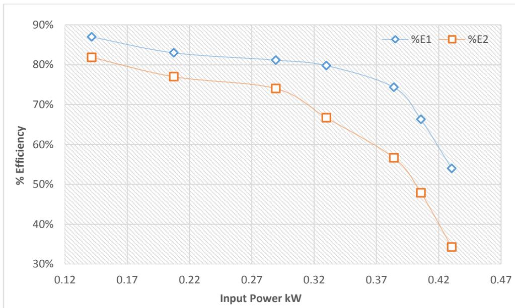
Fig.5.21 Converter efficiency test with different L design (%E1= new inductor, %E2= existing inductor)
