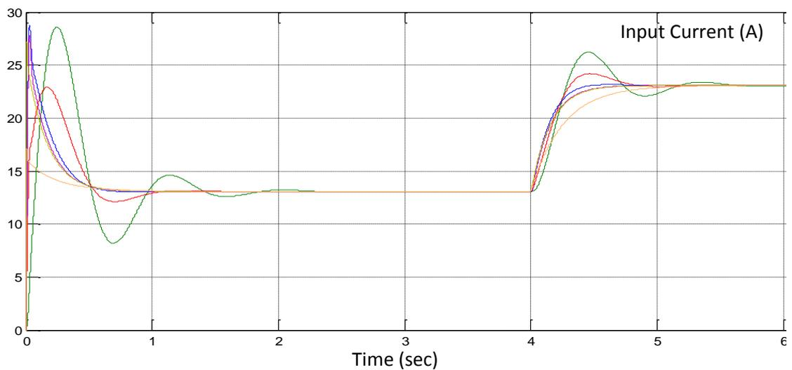
Fig.4.12b Different time response for the tuned gain values for the controller gain set up in table 4.2
