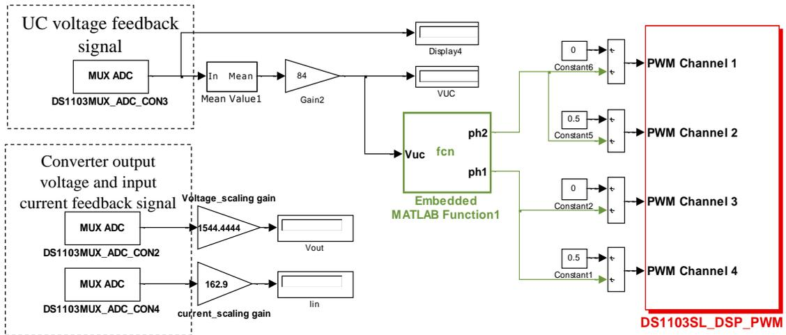
Fig.5.33 dSPACE Matlab configuration for BDC control
