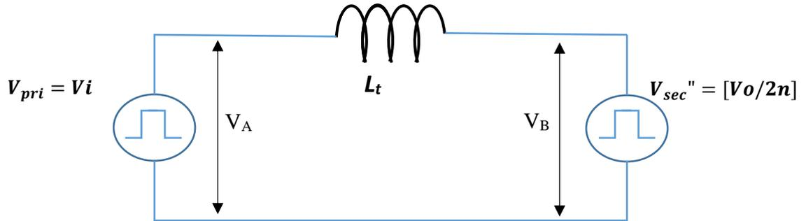
Fig.5.8 Simplified IBDC equivalent scheme
