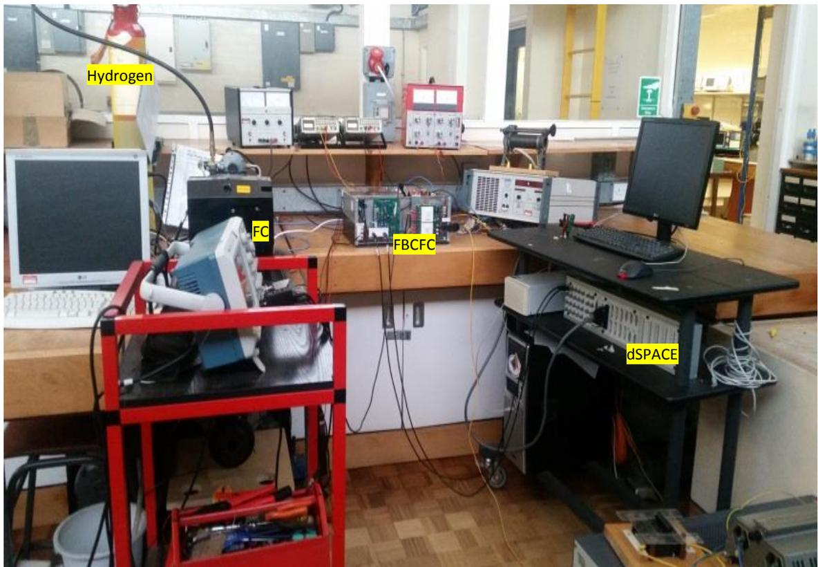
Fig. 4.23 Experimental set-up of the FC and the FBCFC in the laboratory (see Fig.3.38 for the block diagram of the test arrangement)
