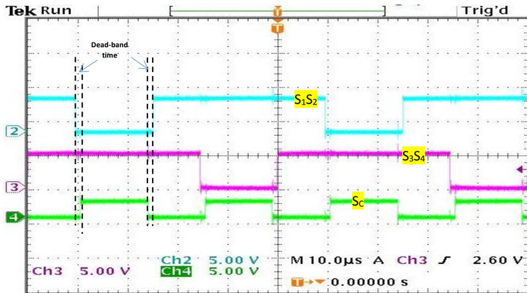
Fig.3.18 Overlap PWM signals for the bridge and clamp switches using dSPACE
