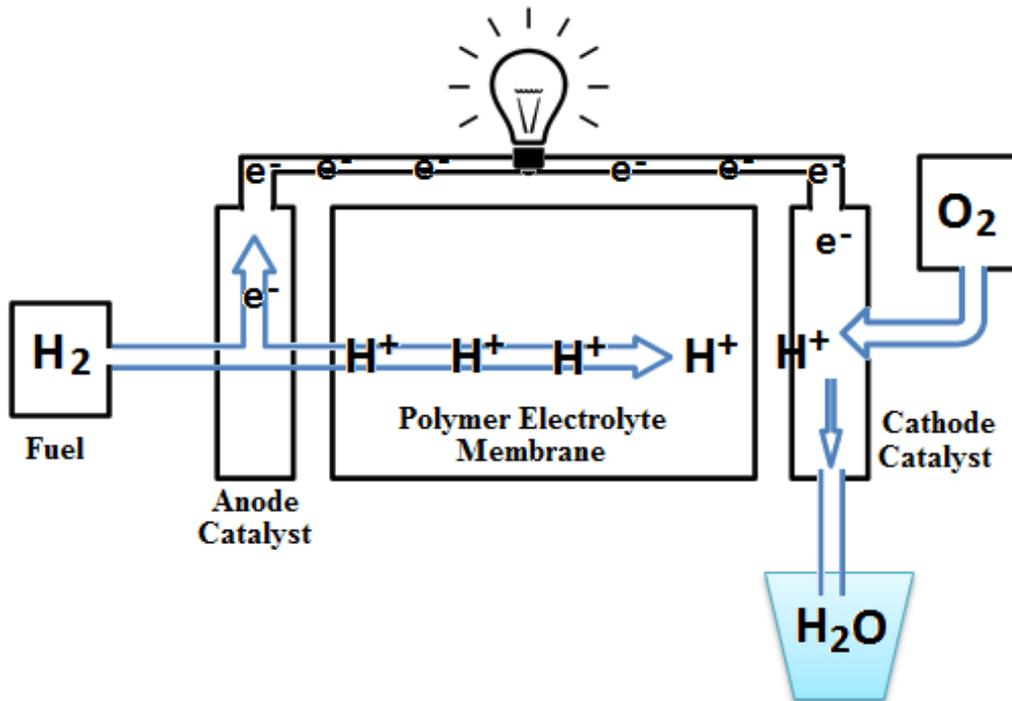
Fig.2.2 PEM Fuel cell principle
