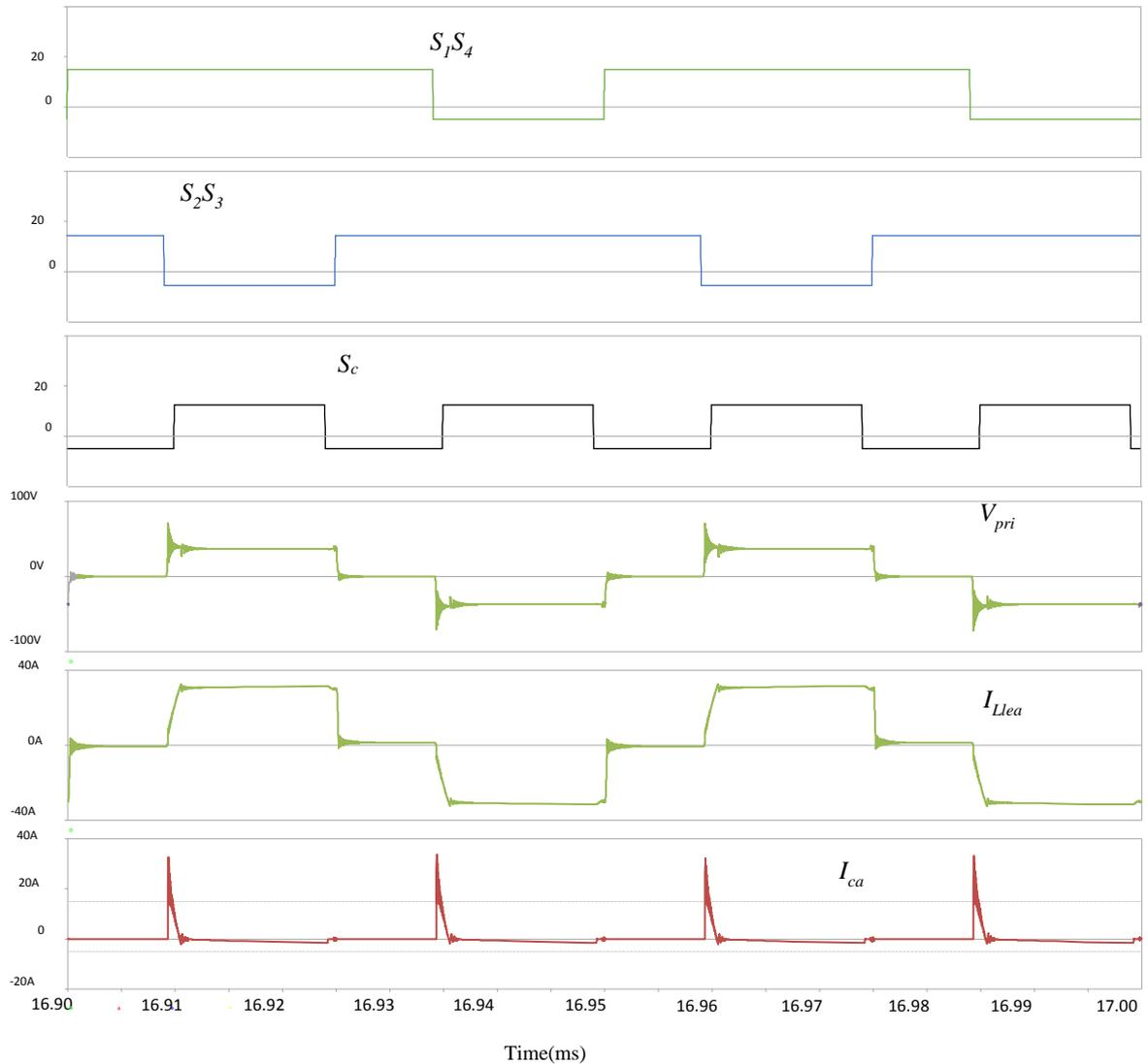
Fig. 3.33. Simulation result of the FBCFC circuit combined with IMACC; from the top: the gate pulses, the primary winding voltage and current, and the clamp capacitor current
