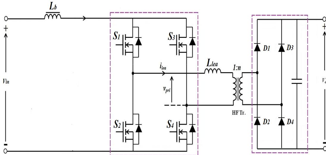
Fig. 2.13 Typical topology of current-fed DC/DC converter.
