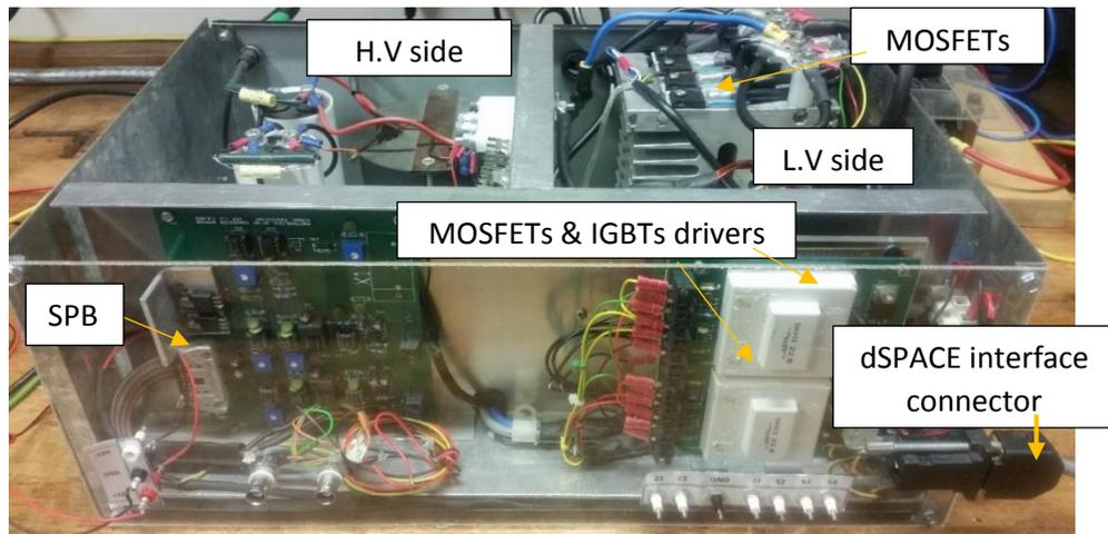
Fig.5.15 Voltage fed converter
