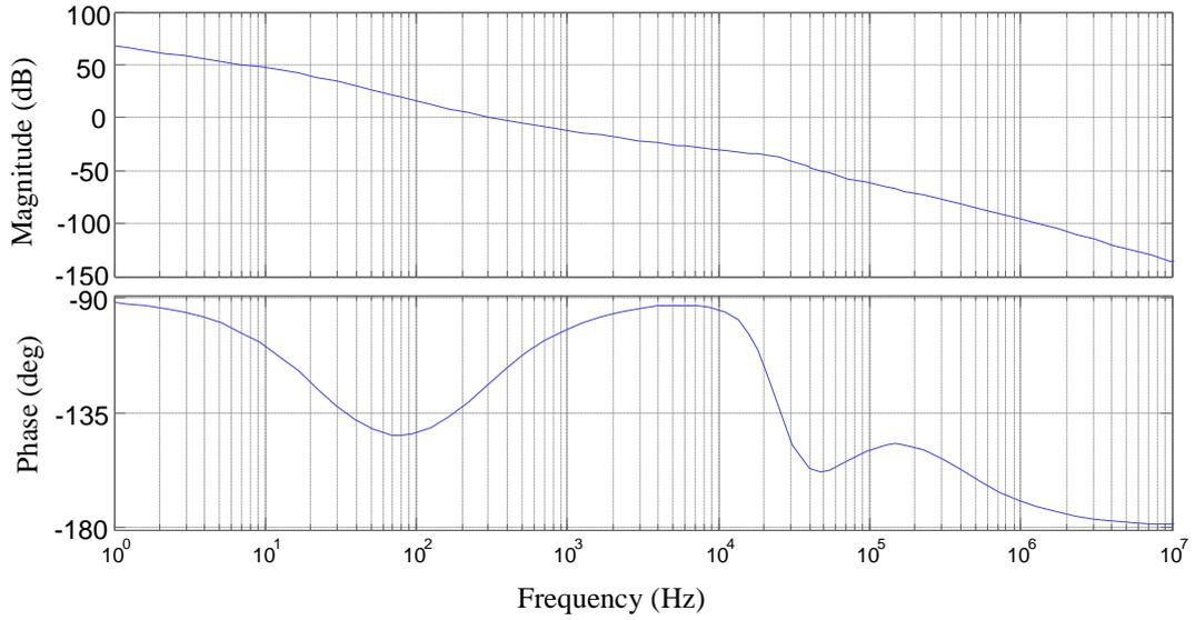
Fig. 4.7 Bode plot of open loop transfer function  $T_{op}(s)$
