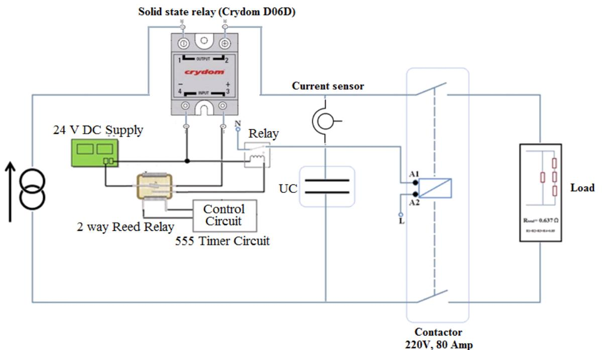
Fig.2.19 The experimental set-up of the UC Maxwell module
