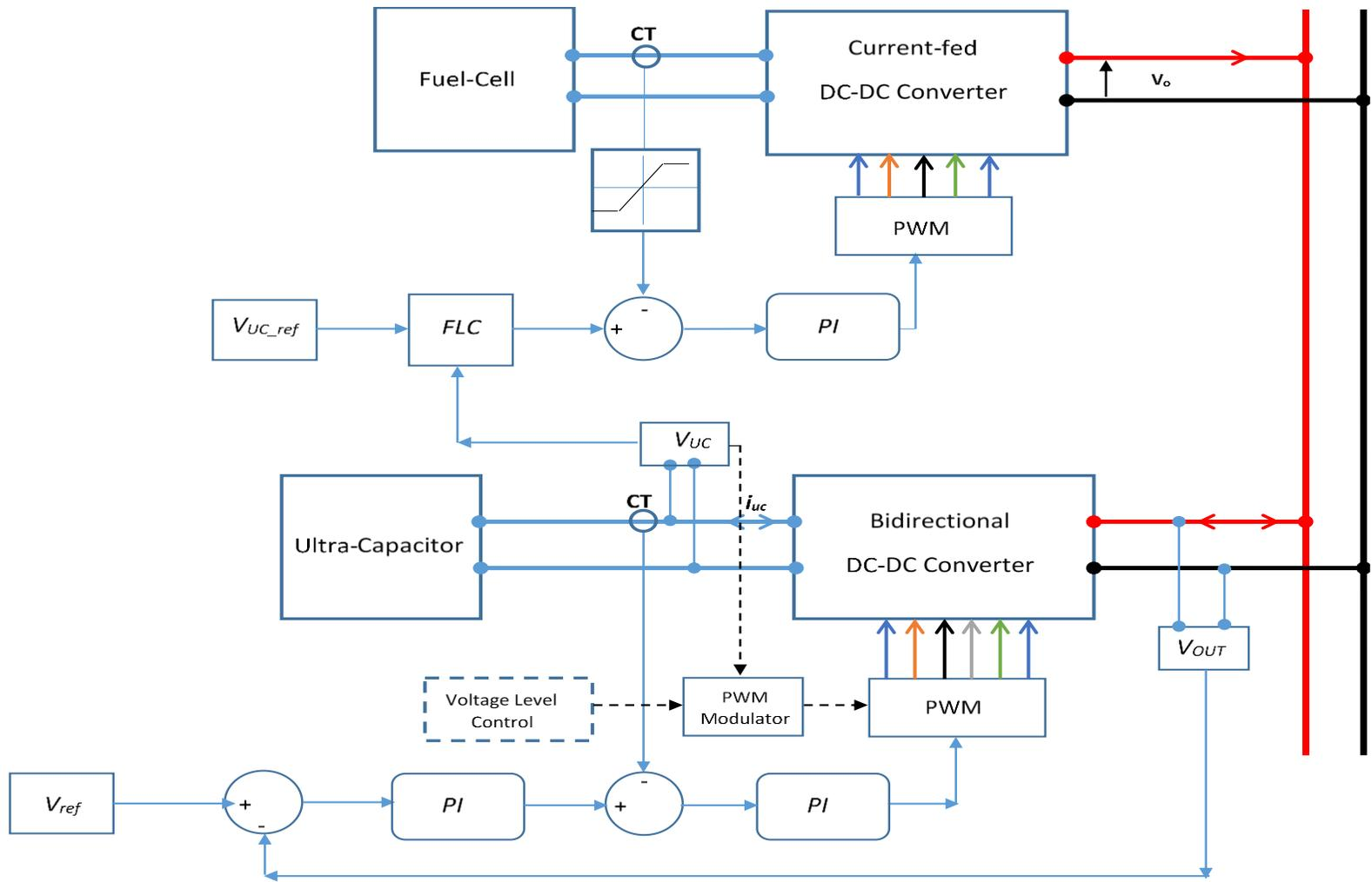
Fig.2.30 Control scheme for the FC-UC DC micro-grid
