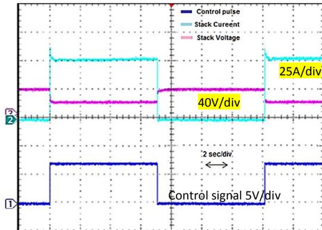
Fig. 2.9 Accurate transient response using experimental set-up in Fig.2.7
