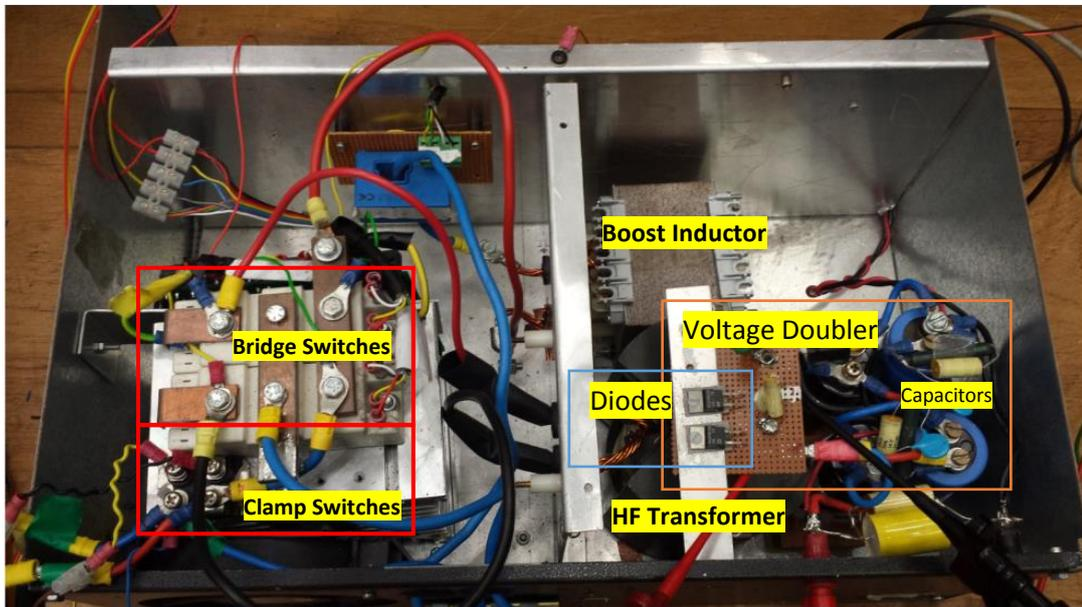
Fig.3.21 1.2 kW power converter
