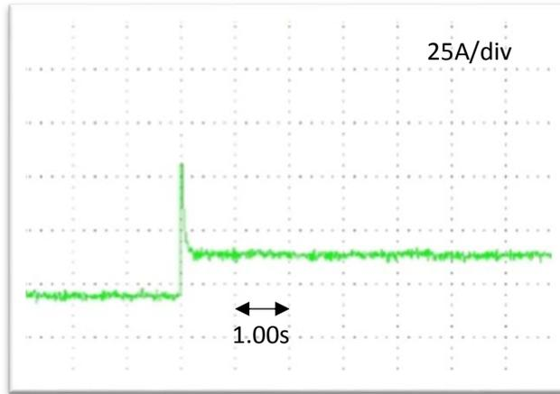
Fig.2.10 Fuel cell current transient at load application from no-load on first load application
