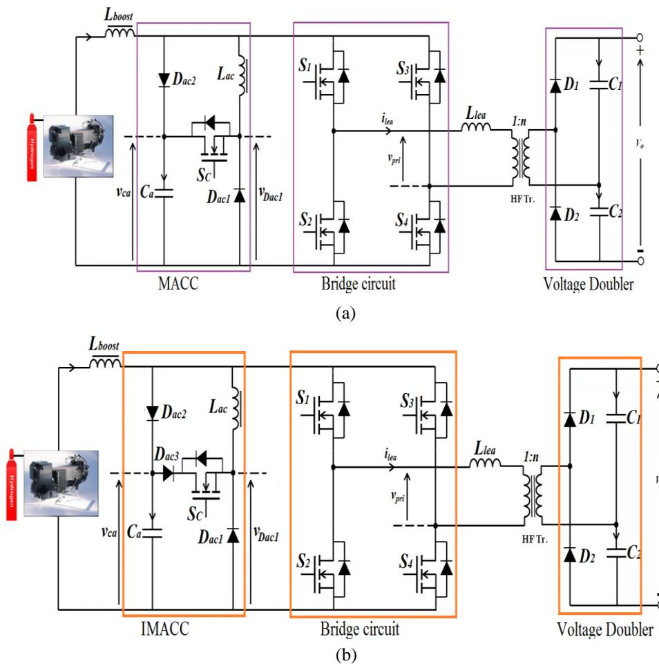
Fig.3.30. FBCFC with: a) MACC, b) IMACC
