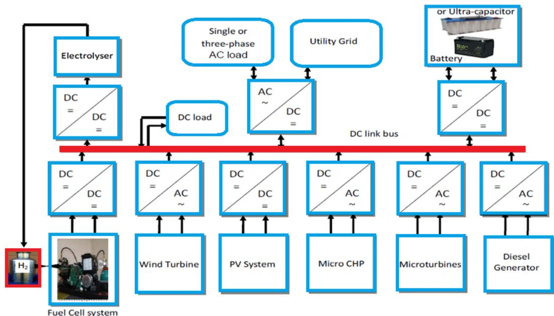
Fig. 1.3 Basic configuration of the DC micro-grid system
