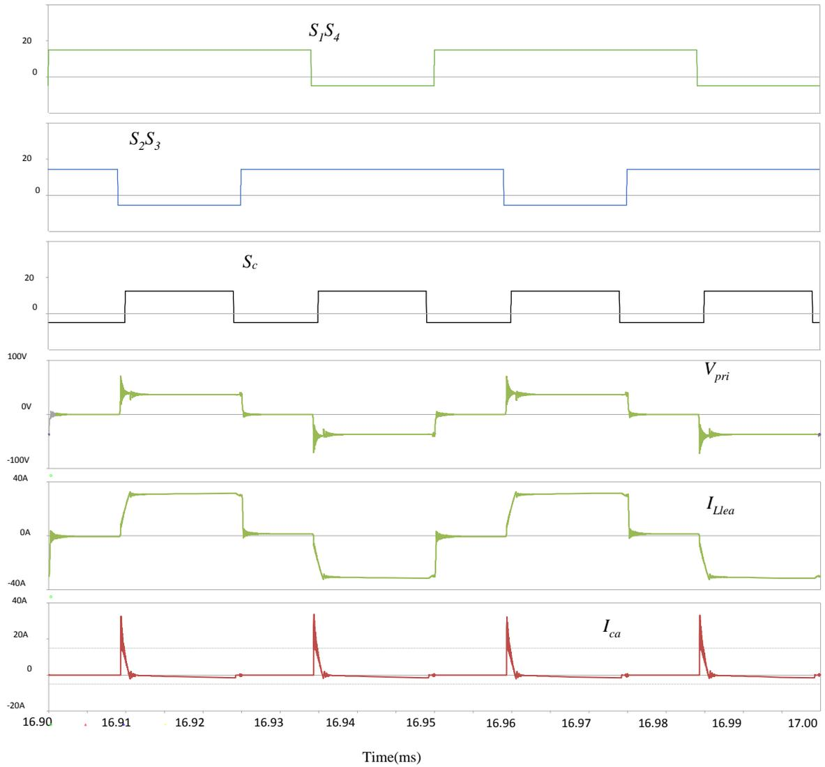
Fig. 3.33. Simulation result of the FBCFC circuit combined with IMACC; from the top: the gate pulses, the primary winding voltage and current, and the clamp capacitor current
