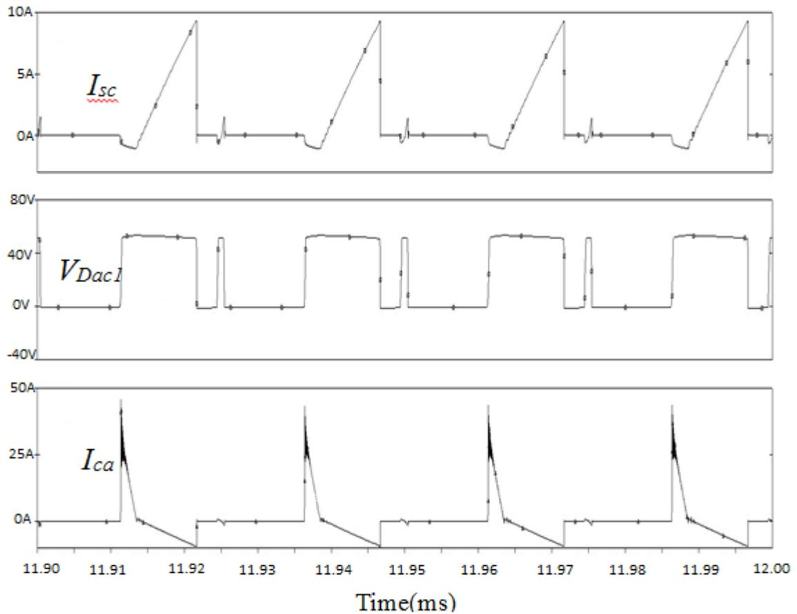
Fig.3.34 Simulation results for the FBCFC circuit showing the effect of the intrinsic diode of the active clamp MOSFET; top: clamp switch current, middle: voltage across  $Dac1$ , bottom: clamp capacitor current
