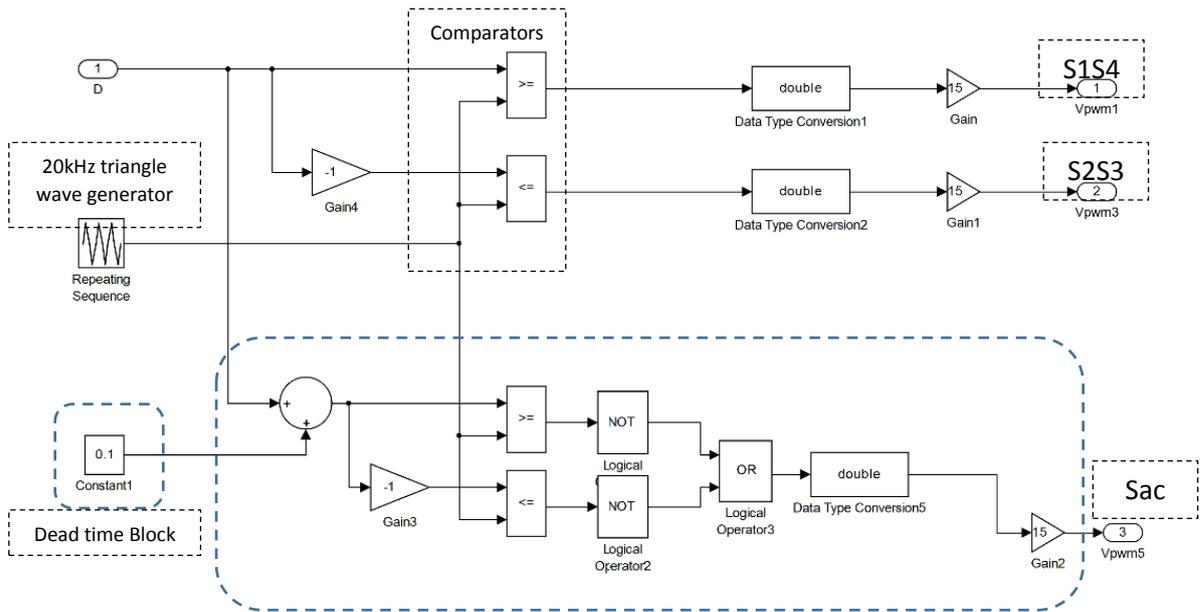
Fig. 4.15 PWM generating circuit in Simulink for the CFC devices
