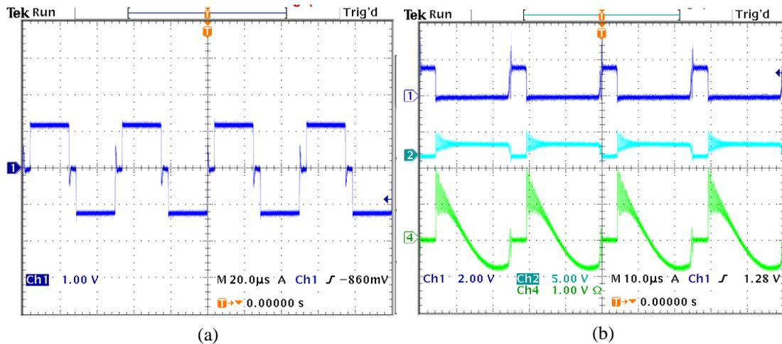
Fig.3.28 Results with the RC snubber modification [312 watt,  $D=0.6$ ]: (a) transformer secondary voltage, (b) From the top active clamp voltage, voltages across the bridge switches, and the active clamp current
