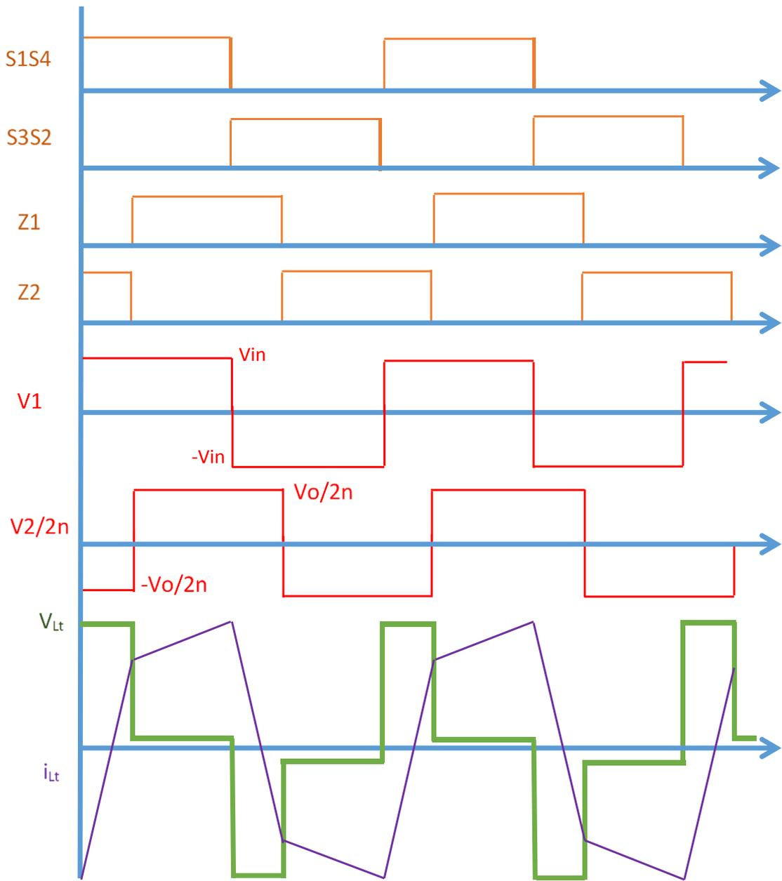
Fig.5.9 Main IBDC waveforms
