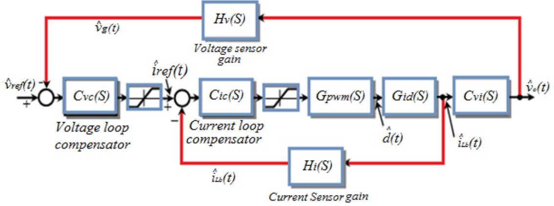
Fig. 4.5 Two loop average control system
