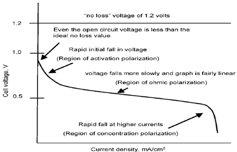
Fig.2.3 FC voltage-current characteristics [66, 67].
