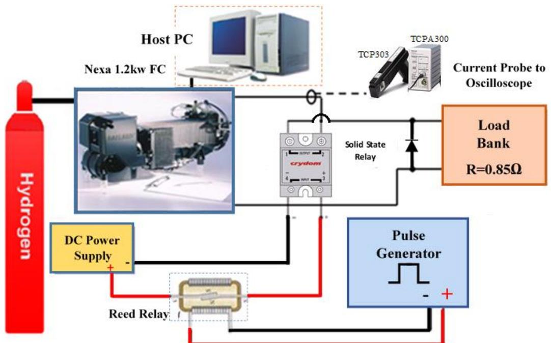
Fig.2.7 The experimental set-up of the Nexa 1.2kw power module
