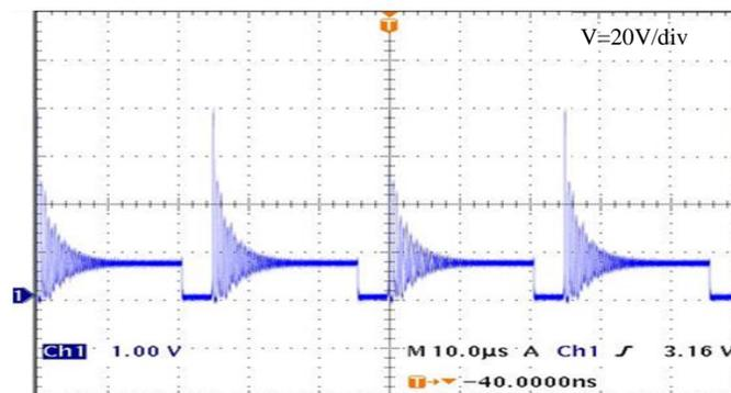
Fig. 2.14 Voltage overshoot across the switches of the FBCFC
