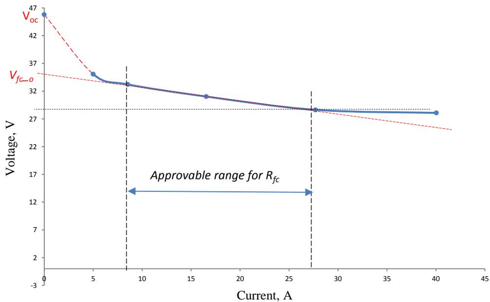
Fig. 2.11. Measured Nexa 1.2kW FC voltage-current characteristic
