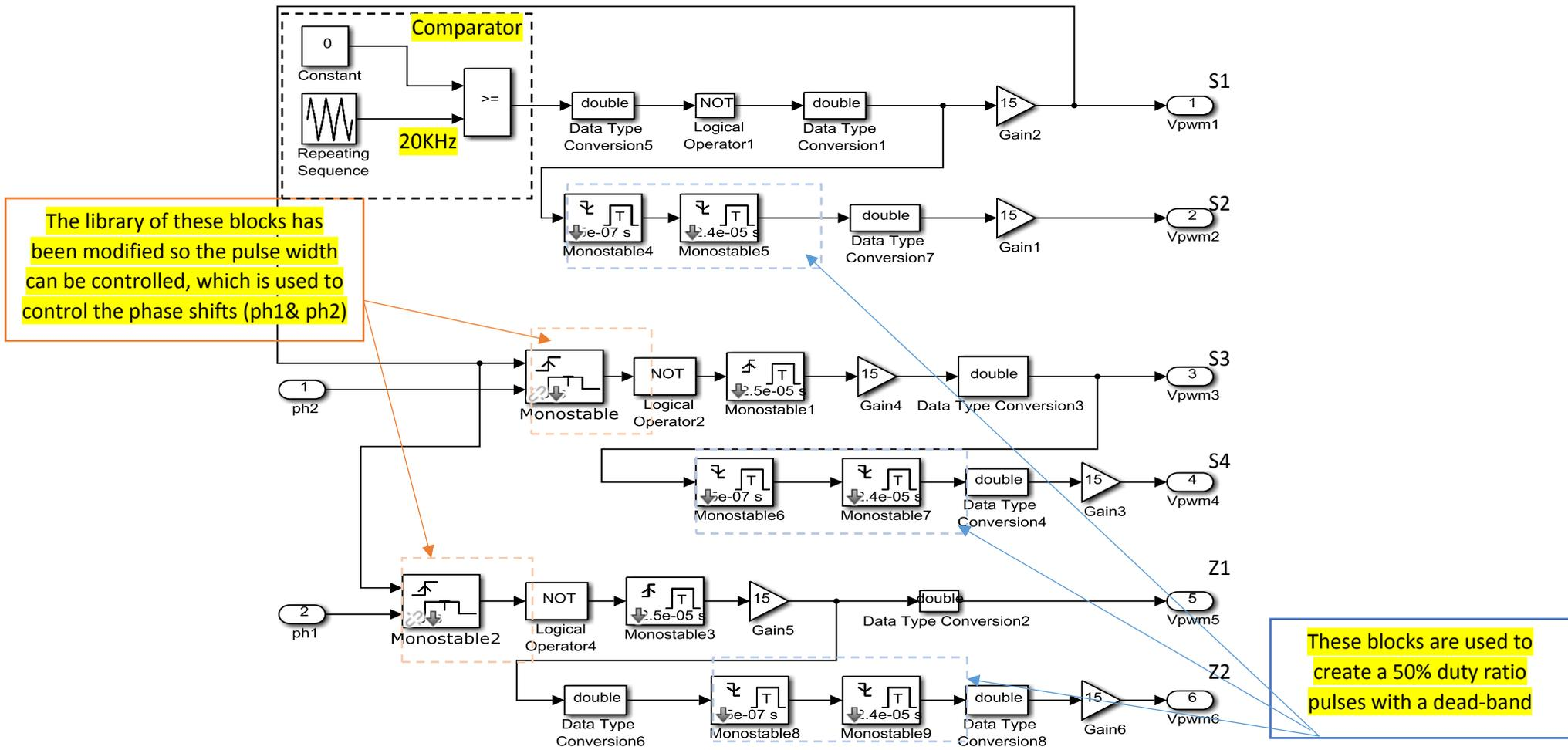
Fig.5.22 VFC timing signals using Matlab Simulink
