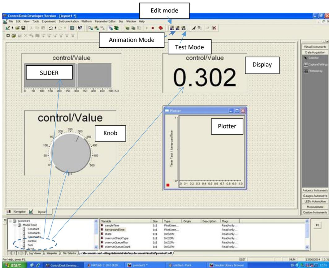
Fig. 3.19 Layout in ControlDesk with system running and slider and knob used to change the Duty Cycle
