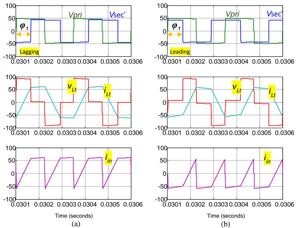
Fig.5.27 BDC with two operation modes: a) UCDM for  $\phi_1=90^\circ$ ,  $\phi_2=180^\circ$ , b) UCCM  $\phi_1=-90^\circ$ ,  $\phi_2=180^\circ$
