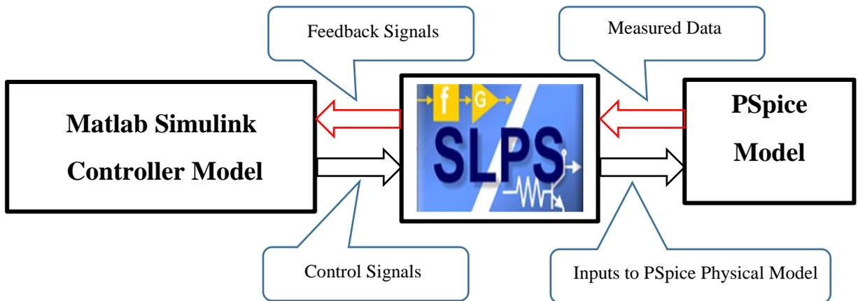
Fig. 4.13 Block diagram of the basic operation of the SLPS system
