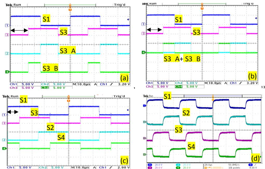
Fig.5.17 Steps for generating phase shifted timing pulses for the VFC
