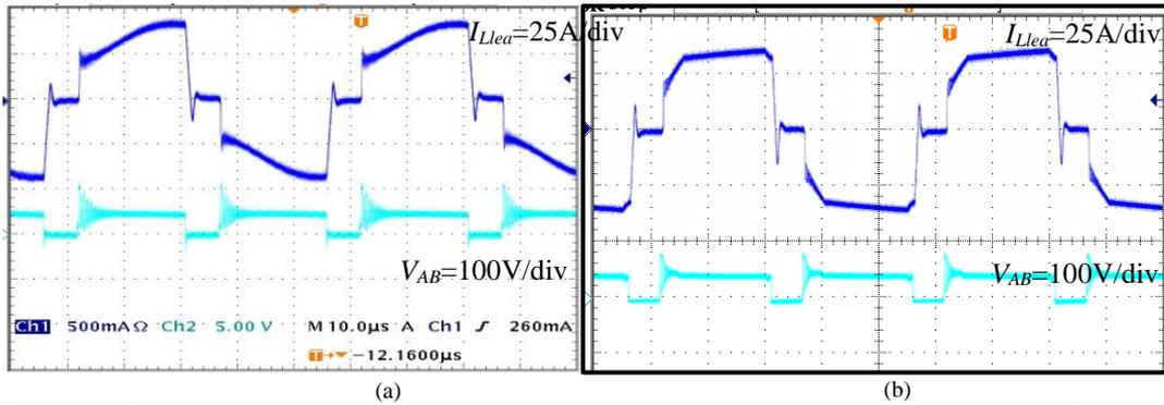
Fig. 3.44 Primary winding current (top) and voltage (bottom) across the main devices at 90% of full load: a) CACC, b) IMACC
