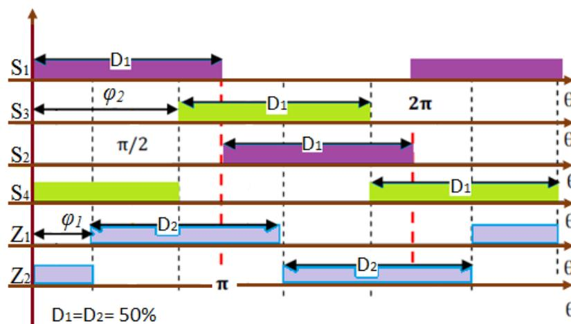
Fig. 5.14 Switching control algorithm for the BDC
