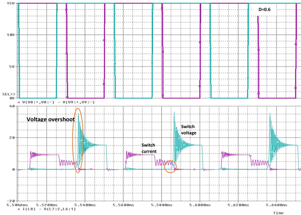
Fig.3.7 From the top: the overlap pulses with a duty ratio of 0.6, the voltage and the current of one bridge switch
