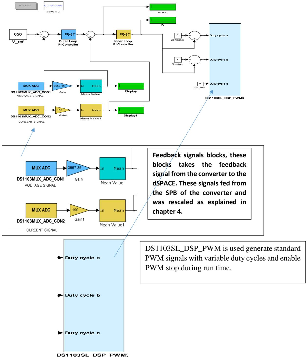
Fig.B FBCF Controller Blocks using dSPACE
