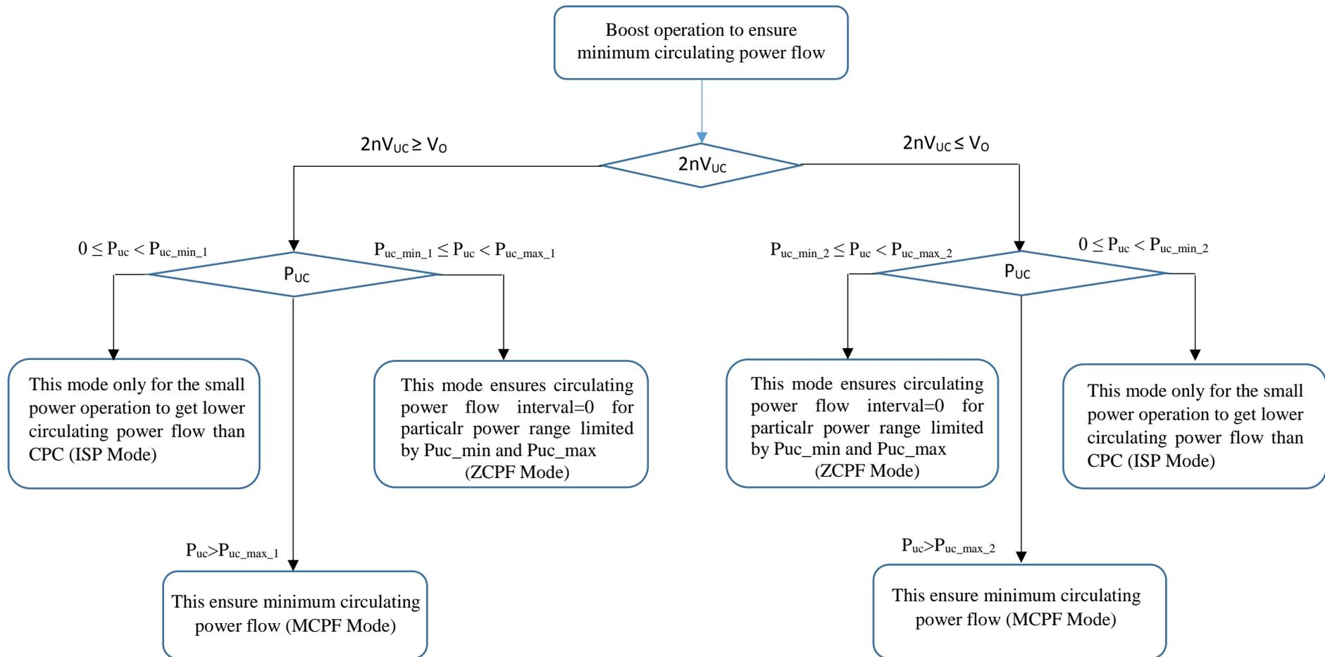
Fig.5.37 A flow chart of the optimum phase shift control algorithm (boost operation)
