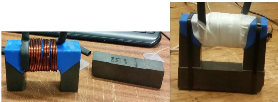
Fig.5.20 Designed inductor steps
