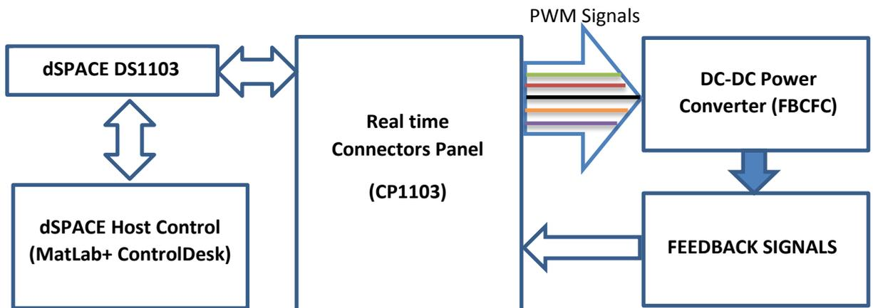
Fig.4.19 Block diagram of hardware setup
