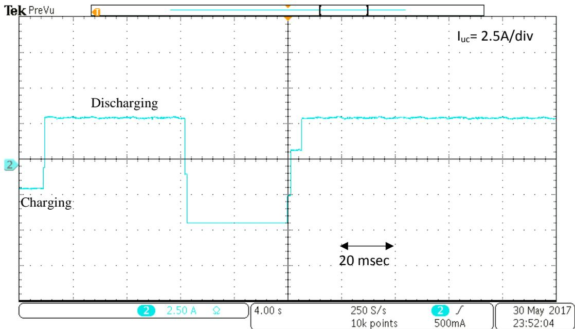
Fig.5.34 UC current during the charging and discharging
