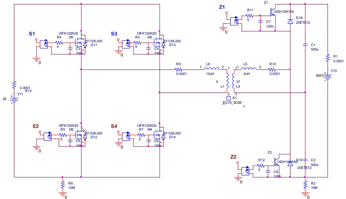
Fig 5.2. Bidirectional Voltage Fed Converter (VFC)
