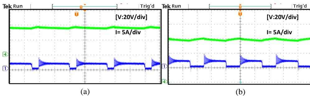
Fig.3.26 Boost current and bridge voltage [at 312 W] for (a)  $D=0.6$ , (b)  $D=0.7$
