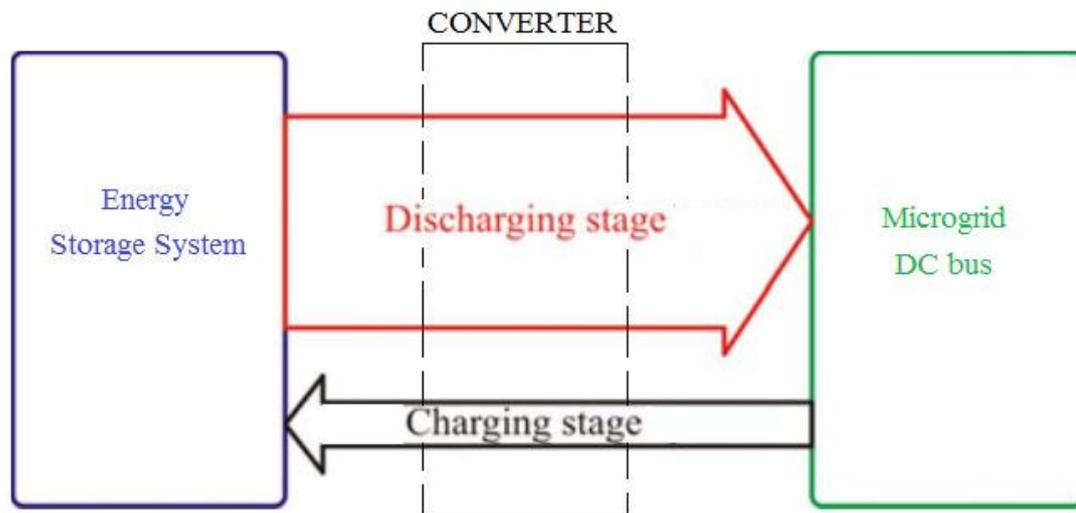
Fig.2.22 Power flow diagram between storage system and micro-grid DC bus
