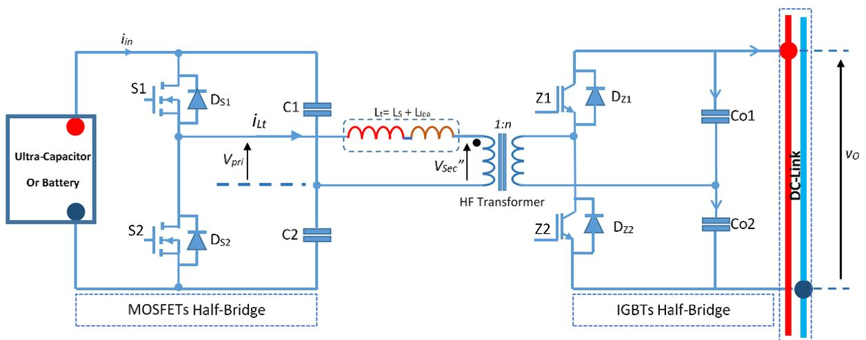
Fig. 2.26 Dual half bridge bidirectional converter
