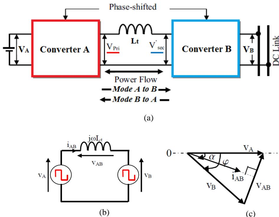
Fig. 2.23 Operating principle of a BDC (a) simplified block diagram (b) equivalent circuit model (c) phasor diagram of the fundamental components of the voltages and current
