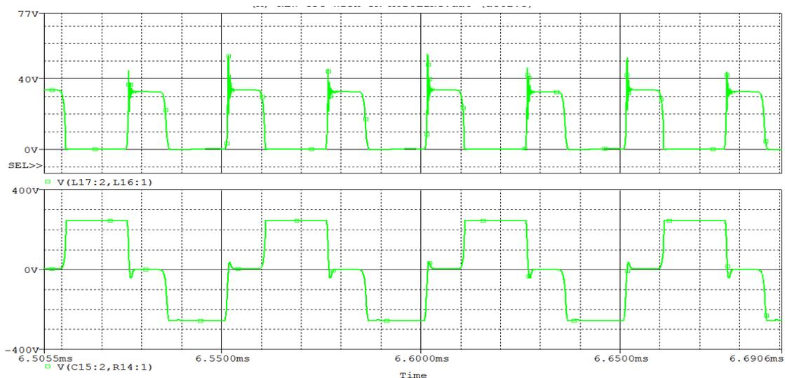
Fig. 3.29 The results in PSpice model, from the top the active clamp voltage, secondary winding voltage
