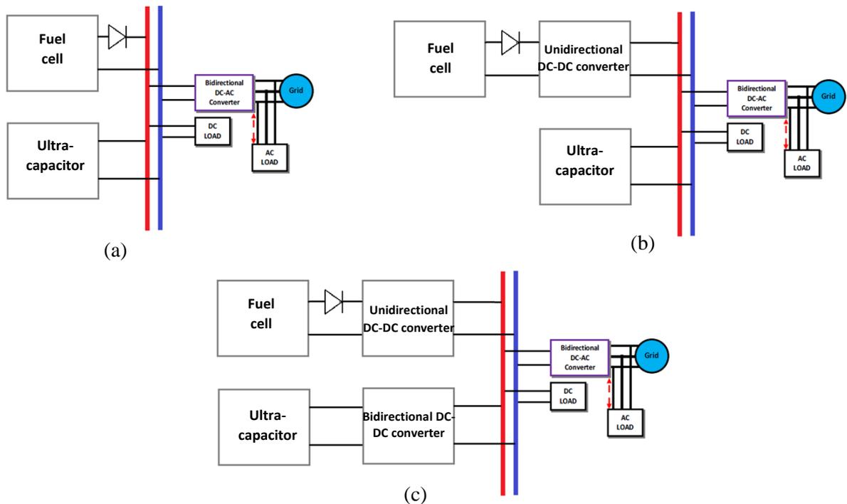
Fig.2.28 Different connection configurations of the FC–UC DC micro-grid: (a) direct connection structure, (b) one-converter connection, and (c) two-converter connection
