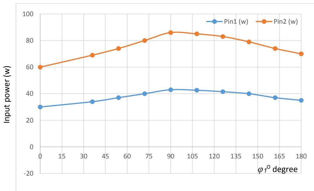
Fig.5.35 Test results for measuring the BDC input power
