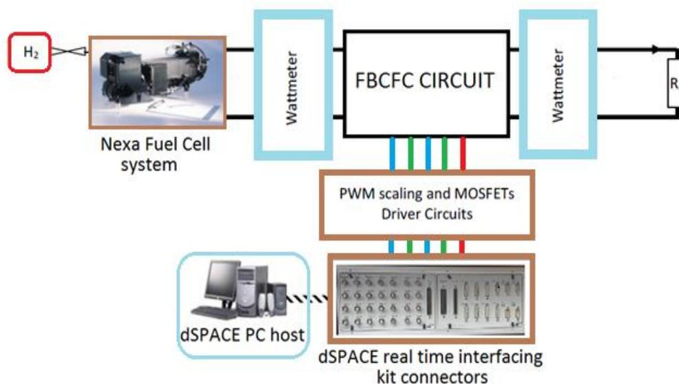
Fig. 3.38 Block diagram of experimental set-up
