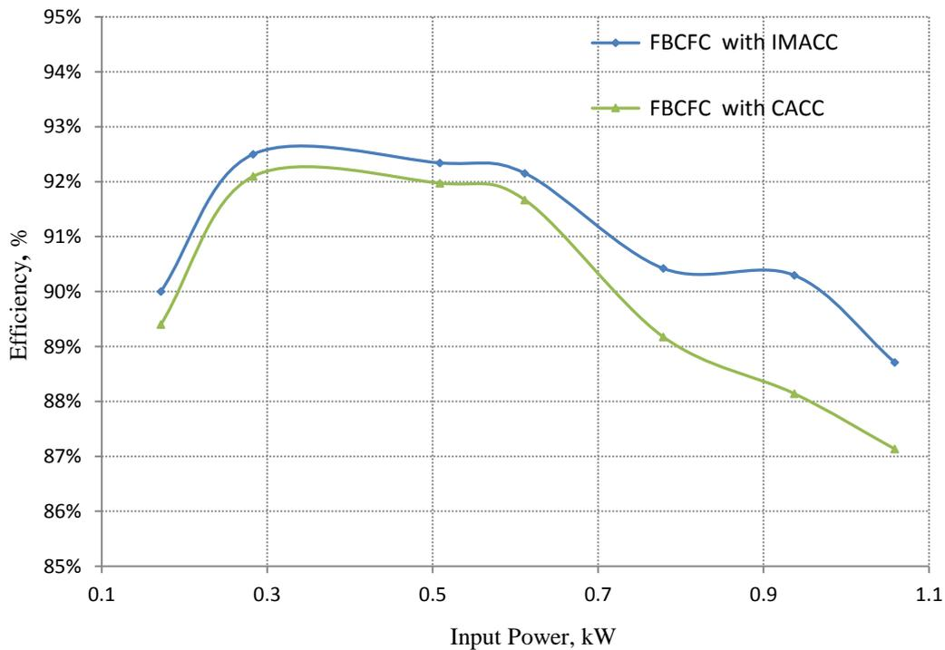
Fig. 3.46. Converter efficiency using a Nexa 1.2kW FC as source
