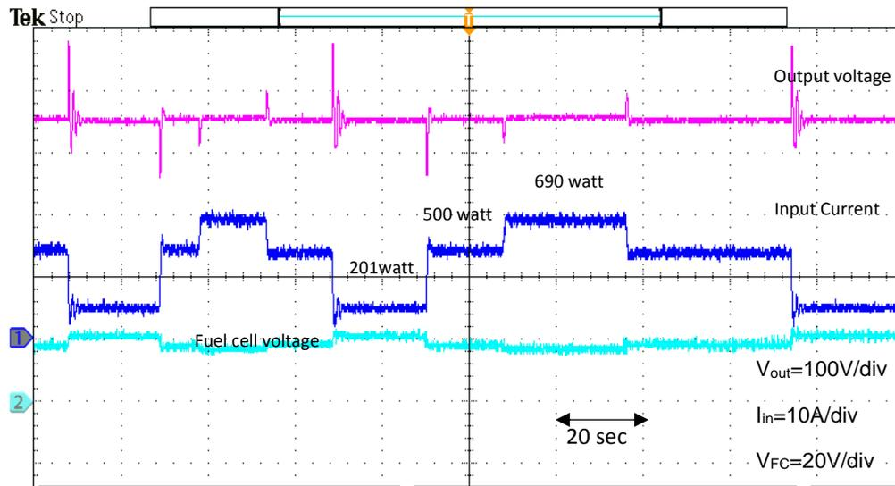
Fig.4.26 Time response for different loads set: from the top: converter output voltage, input current, and fuel cell voltage
