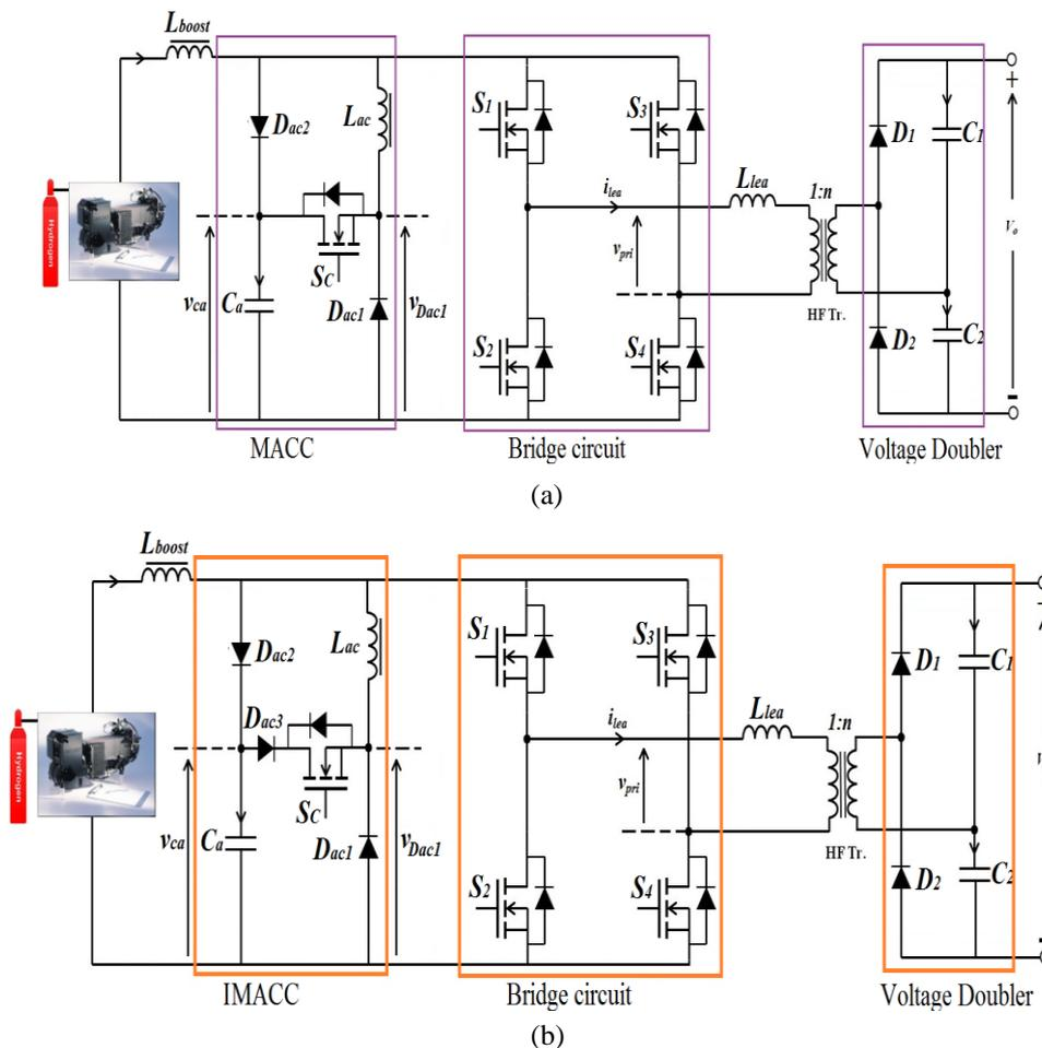
Fig.3.30. FBCFC with: a) MACC, b) IMACC
