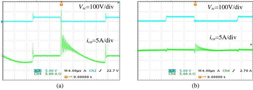
Fig. 3.42 Clamp switch voltage (top) and clamp capacitor current (bottom) at 15% of the full load for: a) CACC, b) IMACC
