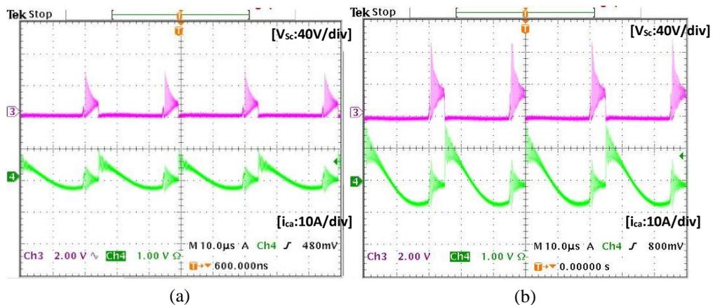
Fig.3.24 (a) Active clamp voltage (top) and active clamp current at 60 W, (b) Active clamp voltage (top) and active clamp current @ 312 W
