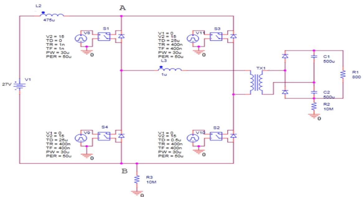
Fig. 3.3 FBCFC model using ideal components
