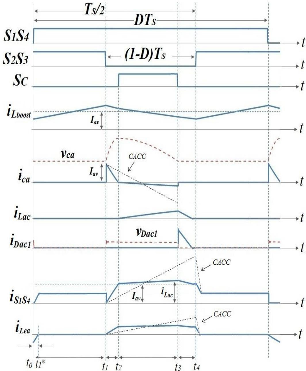
Fig. 3.31. Waveforms of the FBCFC with the modified regenerative clamp circuit
