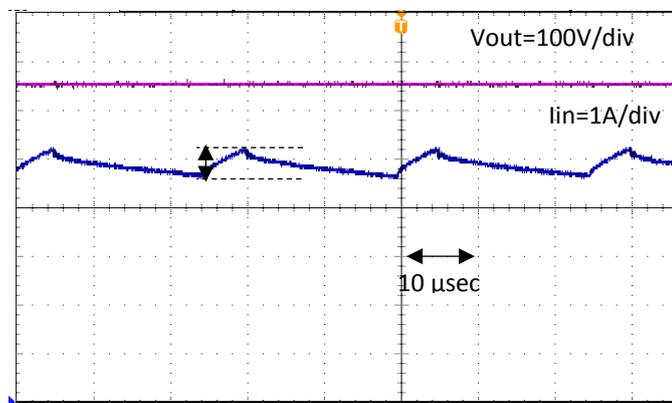
Fig.4.25 Output voltage and the input current of the converter
