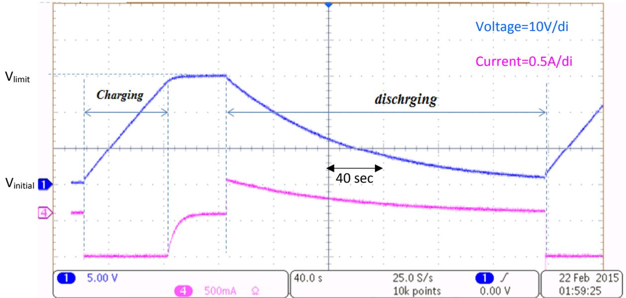
Fig.2.20 UC charging and discharging waveforms from the top: the capacitor voltage, and the capacitor current
