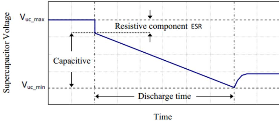
Fig. 2.17 Constant current discharge profile of the UC [85]
