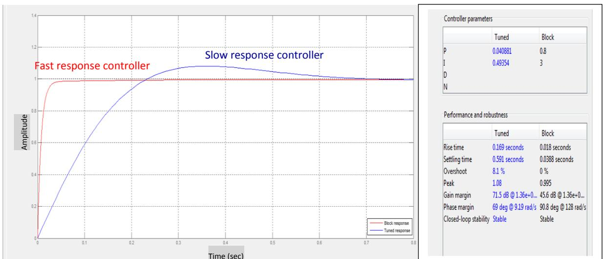
Fig. 4.12a Comparison to previous controller gain settings and the new ones
