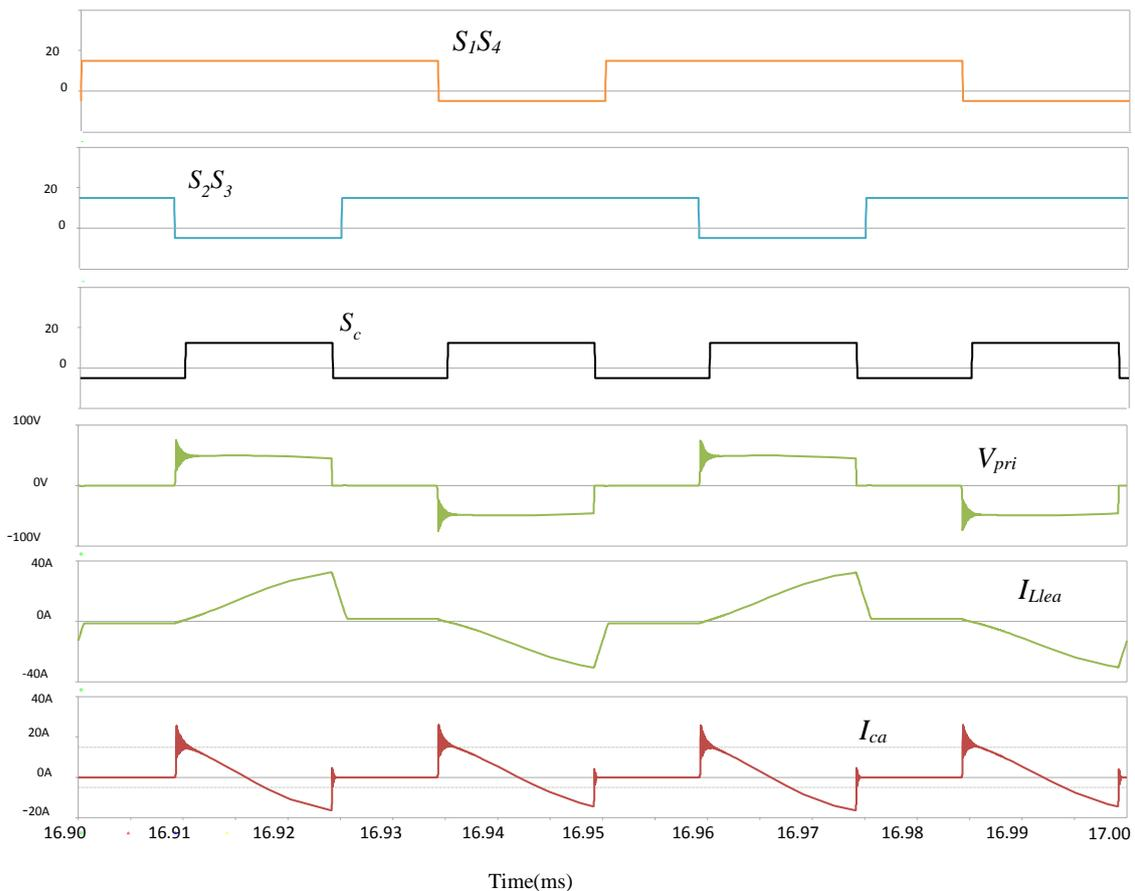
Fig. 3.11. Simulation result of the FBCFC circuit combined with CACC; from the top: the gate pulses, the primary winding voltage and current, and the clamp capacitor current
