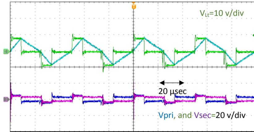
Fig.5.19 Converter wave forms during the test: from the top: inductor  $L_t$  Voltage (green), inductor  $L_t$  Current (light blue), primary winding voltage (dark blue), secondary winding voltage (purple)
