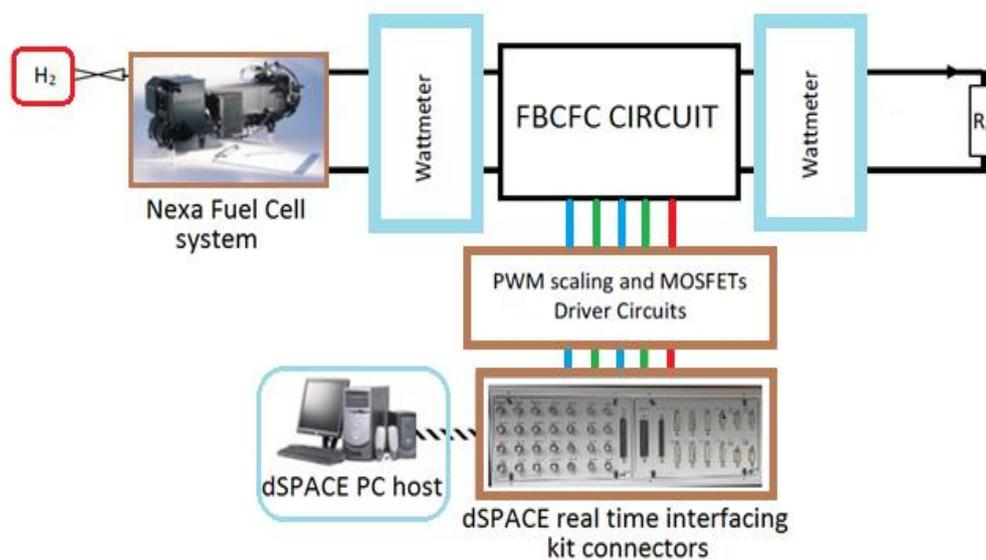
Fig. 3.38 Block diagram of experimental set-up
