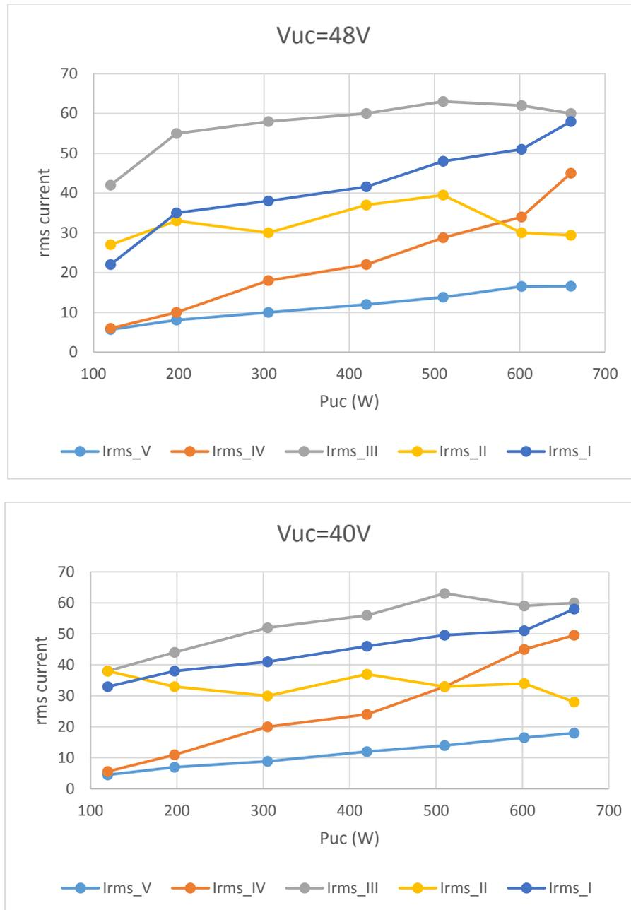
Fig.5.36 The resulting primary RMS current of the BDC operating with different modes under UCDM ( $L_f=10\mu H$ ,  $V_o=650$ ;  $n=7.4$ ;  $f_s=20kHz$ ) for (a)  $V_{uc} = 48V$ , (b)  $V_{uc} = 40V$
