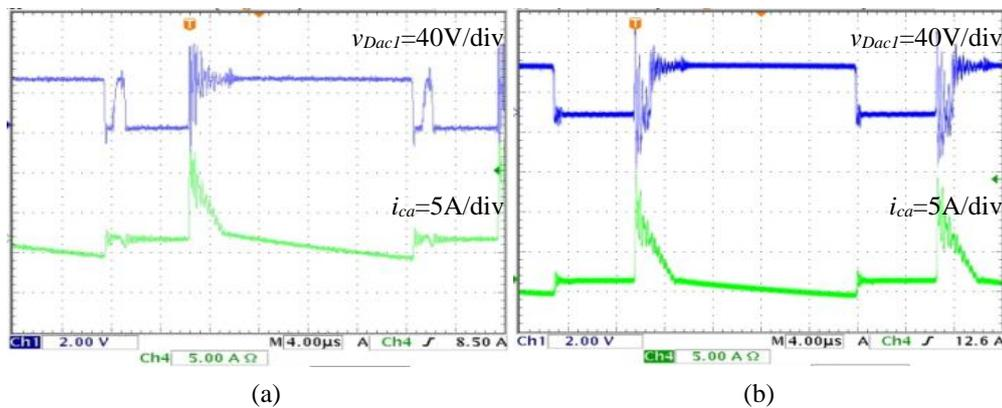
Fig. 3.41 Voltage across  $D_{ac1}$ , and clamp capacitor current of the IMACC at 40% of the full load: a) without series diode  $D_{ac3}$ , b) with series diode  $D_{ac3}$
