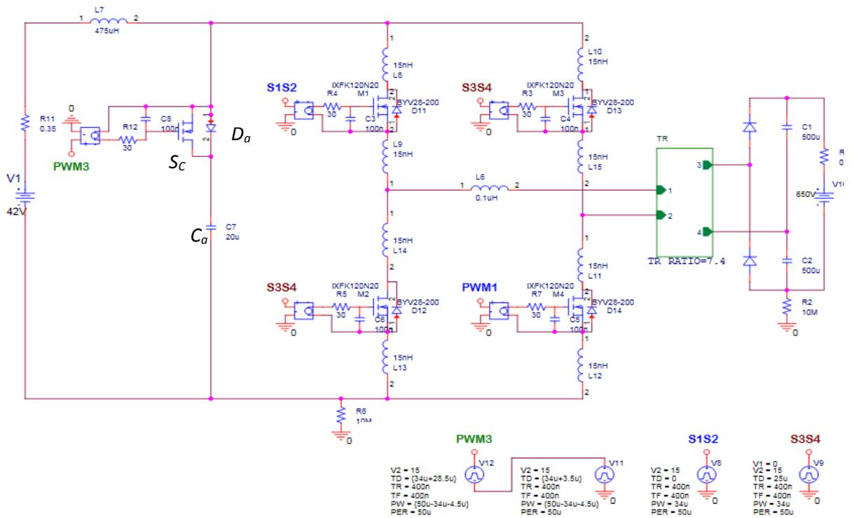
Fig.3.10 the FBCFC with active clamp circuit using PSpice
