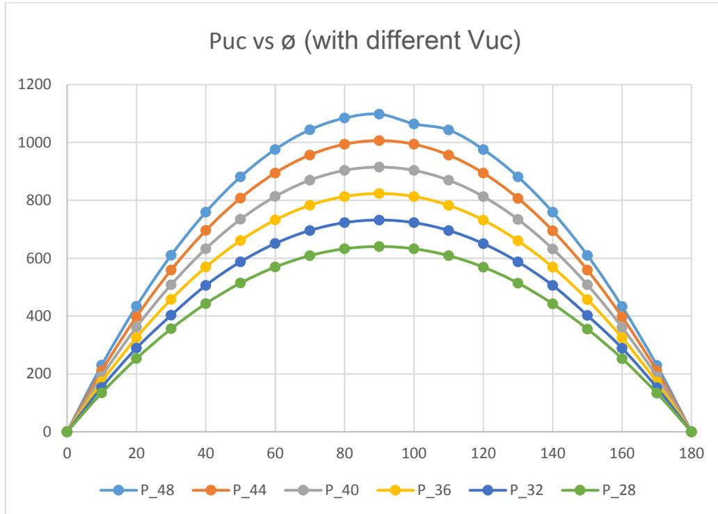
Fig. 5.11 BDC power flow under CPC modulation ( $L_t=10 \mu\text{H}$ ,  $n=7.4$ ,  $V_o=650\text{V}$ , and  $f_s=20\text{kHz}$ )
