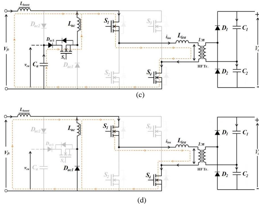
Fig. 3.32. Equivalent circuits of the FBCFC for each operating stage of the IMACC according to the time intervals in Fig.3.30: (a)  $t_1$  (b)  $t_2$  (c)  $t_3$  (d)  $t_4$
