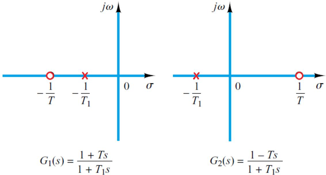
Fig.4.1 Pole-zero configurations of a minimum-phase system  $G_1(s)$  and non-minimum-phase system  $G_2(s)$
