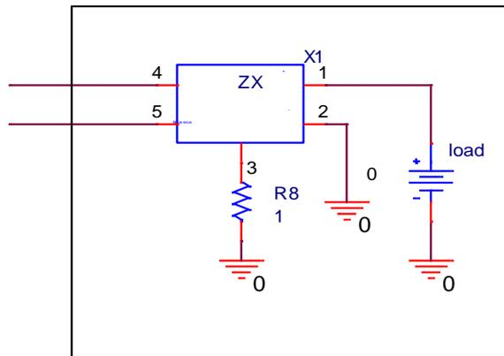
Fig.5.25 Load model in PSpice to be controlled in Matlab/SLPS
