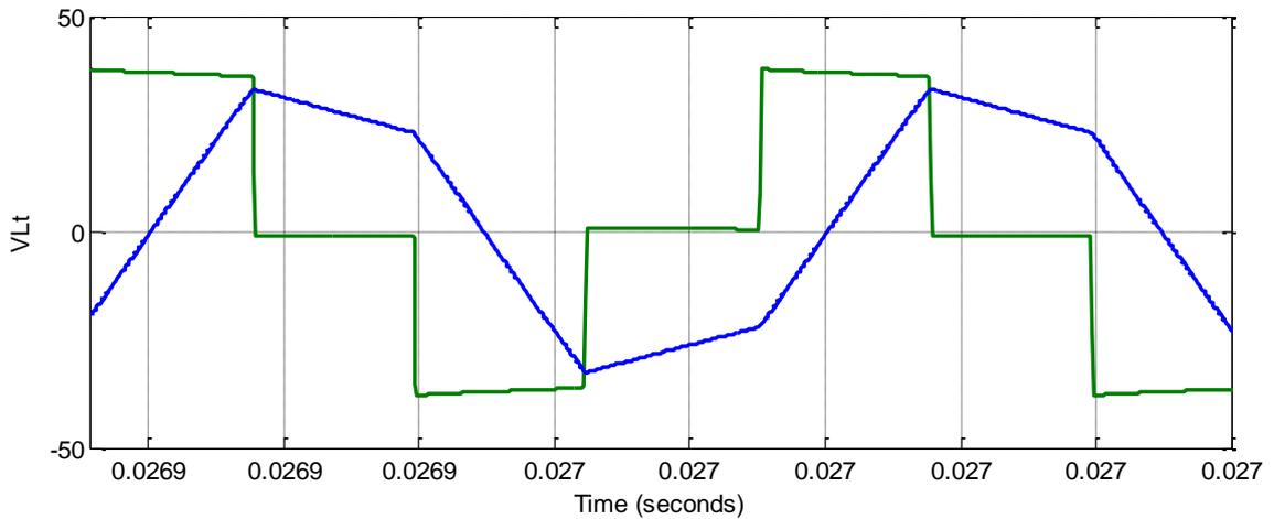
Fig.5.7 Voltage across the Inductor  $L_t$  (green), and the Current through  $L_t$   $i_{Lt}$  (blue)
