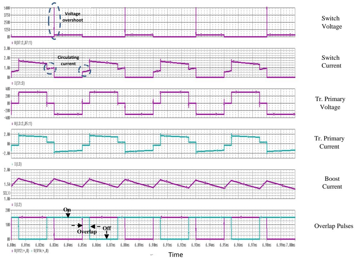
Fig.3.4 Output waveforms of the circuit of Fig. 3.3. From the top: voltage across the switches, switches current, transformer primary voltage, transformer primary current, boost inductor current, and overlap pulses
