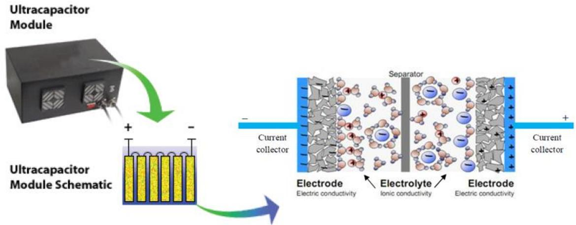
Fig. 2.16 Principle of the ultra-capacitor [42]
