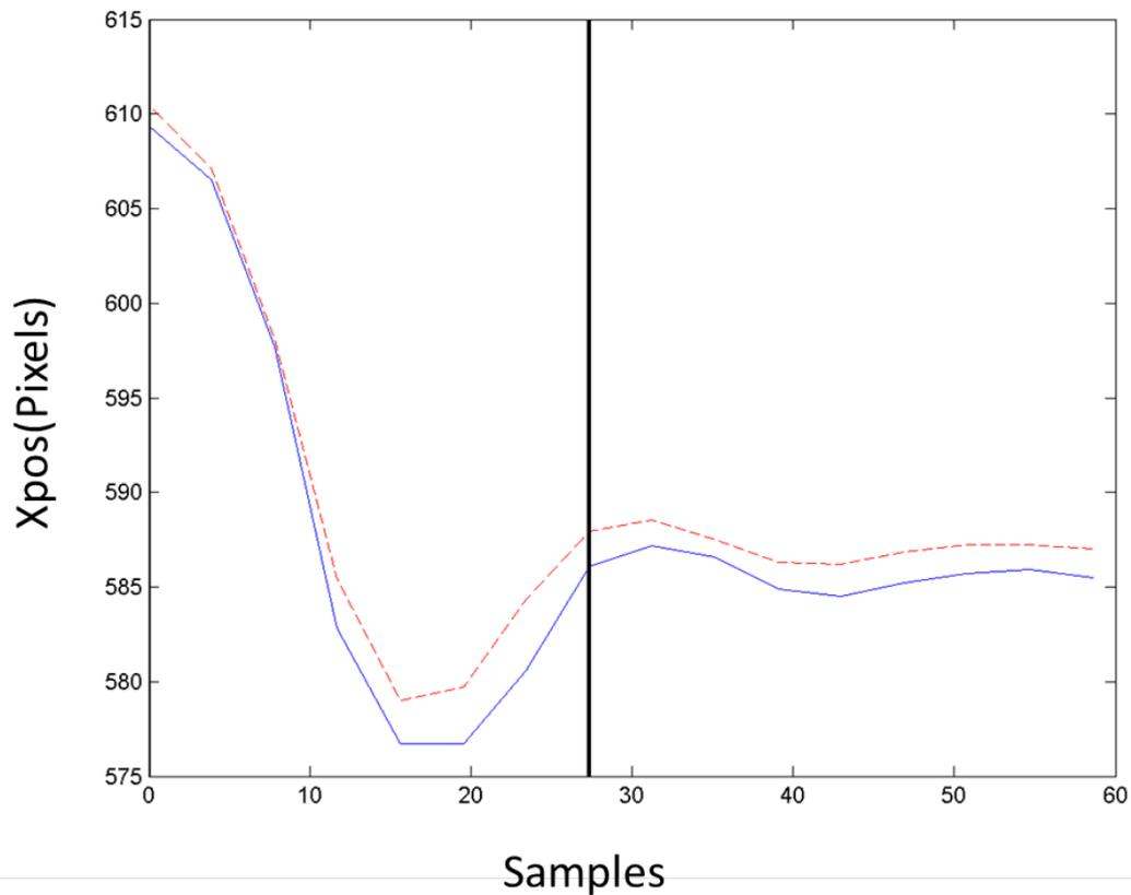
**Figure 2.21 Re-Aligned signal between EEG and ET trace:** The EEG traces (dashed red) are the ET traces sent to the EEG during the experiment, and the ET (solid blue) is the original signal. The artificial delay has been added and the signal is now properly aligned.
