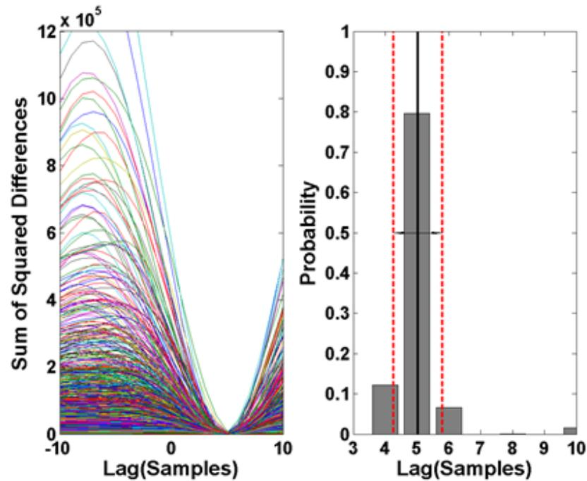
**Figure 2.20 Subject 1 lag vector test results:** The left part of the figure shows the sum of the squared difference between the two signals for all the EEG channels. On the right, is a histogram of the different sample lag, between the two signals, for all the channels.
