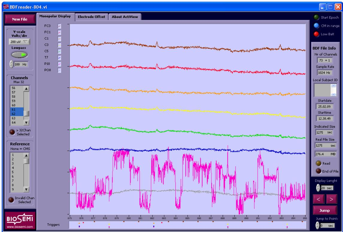
**Figure 2.2 Biosemi ActiView Software:** Records the EEG data at the settings set by the user. The right hand side bar shows the settings of the recording. The left hand side of the figure shows the various channels and the variable views. And in the centre are the digitized EEG traces.
