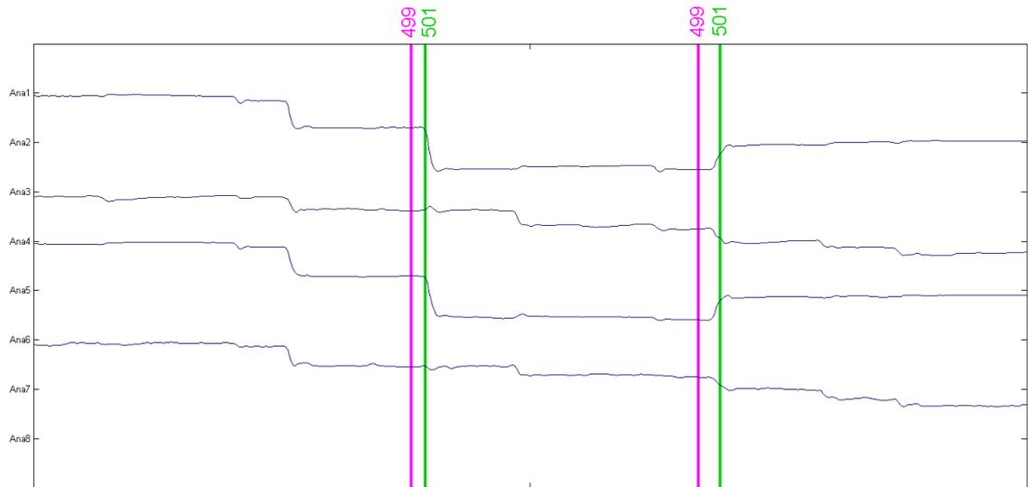
**Figure 2.8 Example of ET traces being sent to the EEG:** Different channel traces are shown in the navy blue each labelled in the y-axis. The ET traces are the step shaped traces. Flat lines indicate a fixation while an increase or decreases in amplitude signify a saccadic eye movement. Different artificial triggers (coloured vertical lines) have been added to the data.
