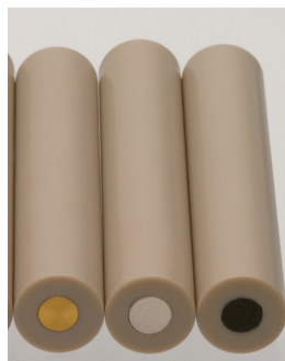
Fig. 3.6 5 mm electrode tips used with the Autolab RDE during these experiments; from (L to R): Gold and platinum electrodes. 16
