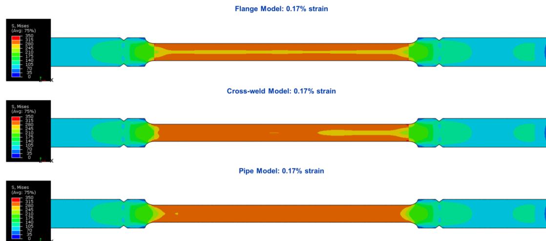
Figure 7.12: Von Mises stress distribution at 0.17 % applied strain. The influence of the residual stresses is almost completely removed at this stage.
