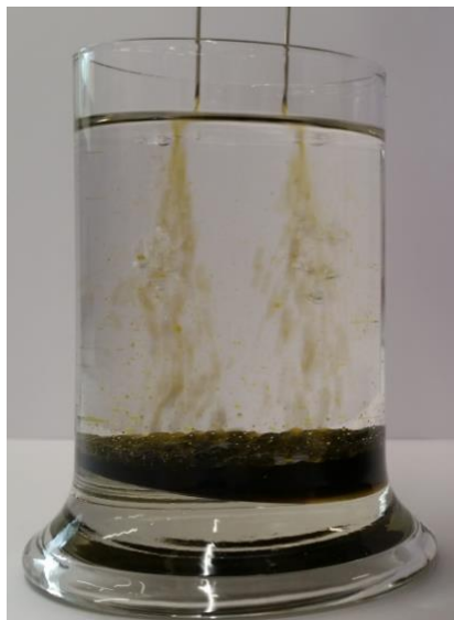
Figure 5.22: Nebulising (\text{Bmim})\text{Cl} : 2\text{FeCl}_3 mixture by injection into the decane fuel.
