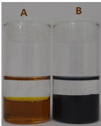
Figure 5.8: 100 mmol L -1 thiophene in decane with (A) 1:5 molar ratio of CuCl 2 :(Bmim)Cl, (B) 2:1 molar ratio of FeCl 3 :(Bmim)Cl.
