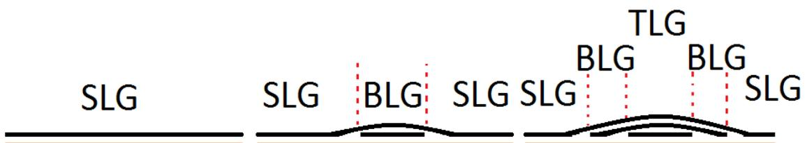
Figure 5.3. The difference in graphene growth for single layer, bilayer and trilayer graphene, showing growth underneath the single layer sheet.
