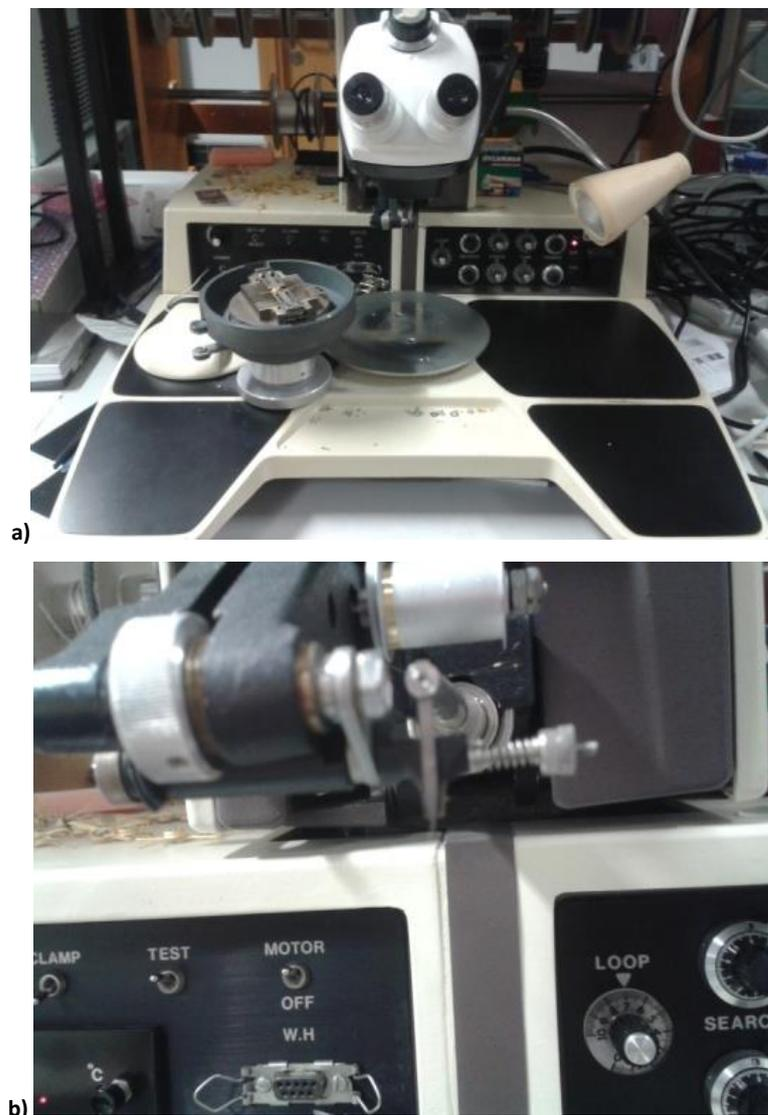
Figure 5.13 showing a) the wire bonder and b) the needle
