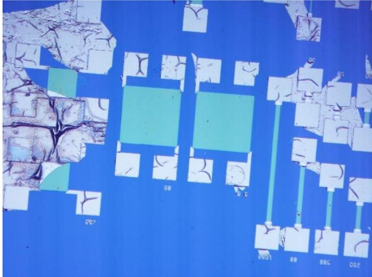
**Figure 5.29**, showing the device with an alumina encapsulation that was removed from over the contacts by an alumina phosphoric acid etch.
