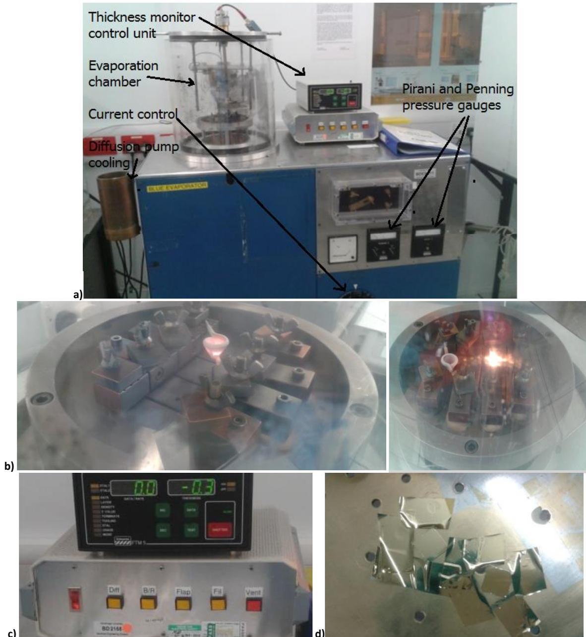
Figure 5.8 showing a) the bespoke diffusion pump thermal evaporator, locally known as the Blue Evaporator, b) the vessel with the current causing it to glow, c) the Edwards FTM5 film thickness monitor, and d) the chip, coated in an evaporated fold film, held on by Capton tape.
