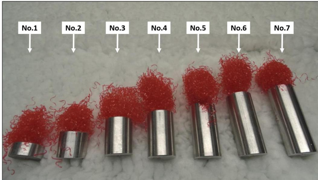
**Figure 2-3: Various weights used for weight lifting tests**
