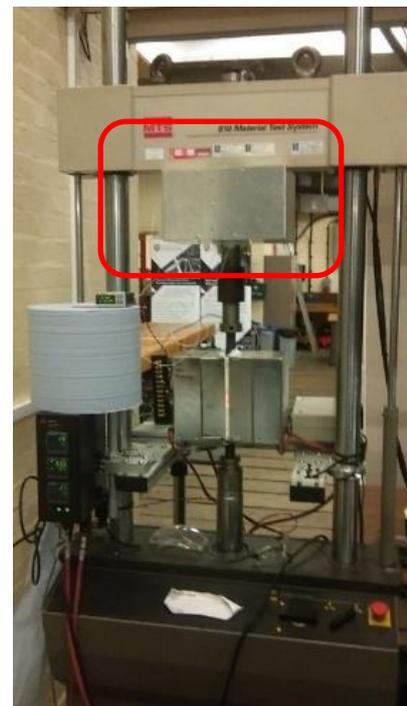
Figure 24: Left: insulation box, right: implementation around load cell (shown in red)
