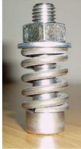
Figure 19: Photograph constrained by nut-and-bolt method, compressed by tightening the nut
