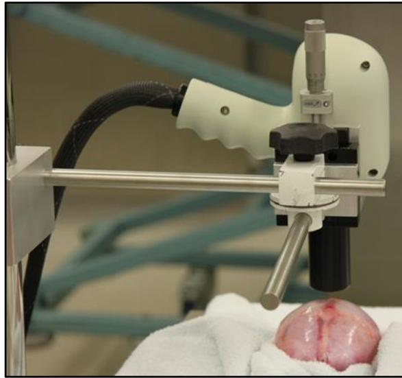
Figure 6.6 Stand for the benchtop OCT imaging probe
