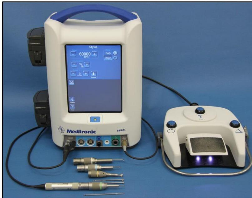
**Figure 4.3 The Midas Rex® Legend EHS Stylus®, high-speed neurosurgical drill**
