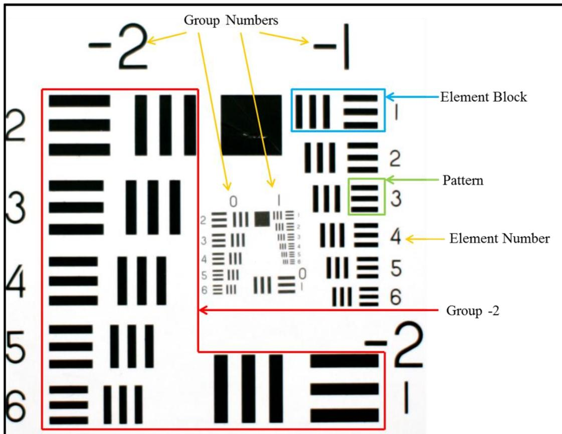
Figure 5.1 The group and element numbers on a USAF 1951 resolution test target
