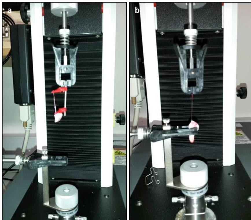
Figure 8.2 Tensile testing machine a) Bridging vein attached with VASCU-STRATT clamp b) vein attached directly to machine without approximator clamp
