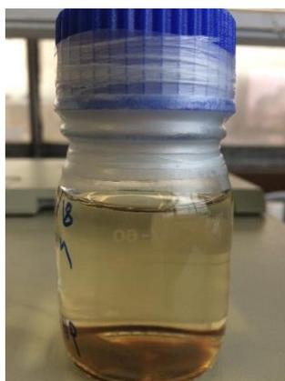
Figure 5.10: The image of the eluted MIP NPs obtained in one synthesis cycle.
