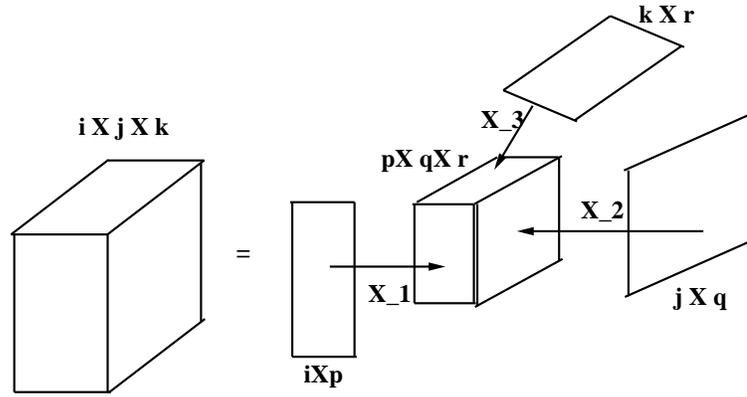
Figure 1.1: Cartoon to represent the sequential multiplication of 3 matrices with a core tensor of order 3, to convert the original core tensor dimensions to that of the final 3-rd ordered tensor. The  $X_i$  in the figure represents the mode- $i$  multiplication between a tensor and a matrix,  $i = 1, 2, 3$ .
