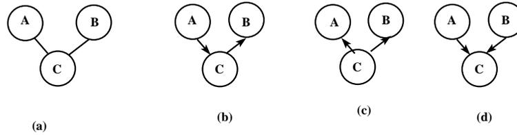
Figure 1.2: Panel (a) represents an undirected graph; (b), (d) and (c) DAGs each, with panel (b) representing a serial graph, (c) a diverging and (d) a converging graph.
