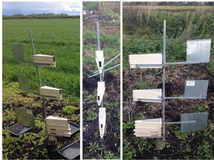
**Figure 5.5:** Photographs of BSNE sampling arrays, installed at measurement heights of 0.15, 0.2, 0.3, 0.65 and 1 m, photos taken by author.
