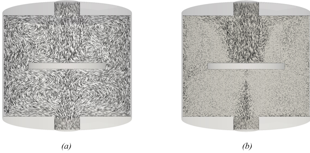
Fig. 7.19 Velocity vector plot for \Delta T = -900 K, (a) SCVD, (b) RCVD.
