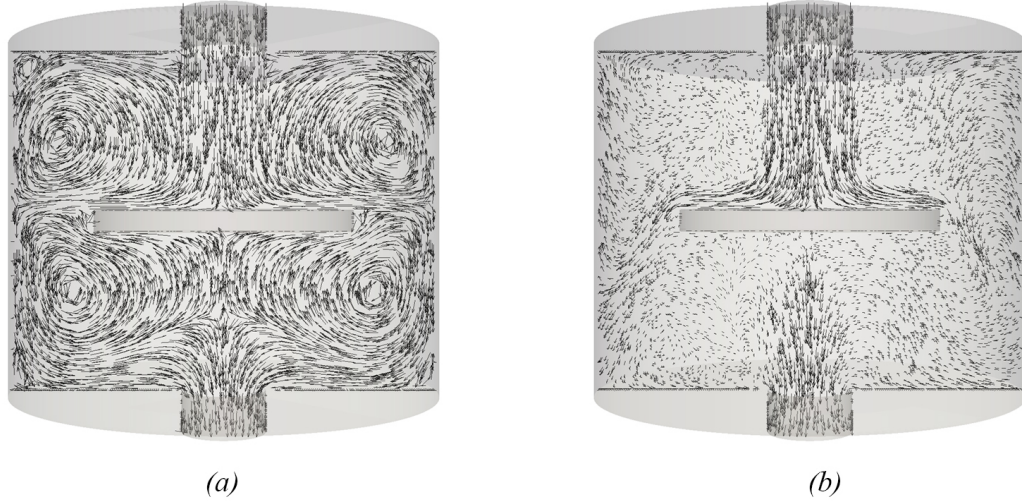
Fig. 7.4 Instantaneous velocity vector plot at \Delta T = 200 K, (a) SCVD, (b) RCVD.
