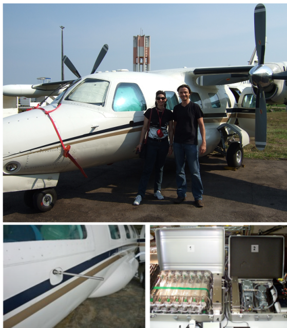
Figure 4.1: Top: The aircraft used to perform measurements for the Amazonian Carbon Observatory project. Bottom left: Close-up of the air inlet. Bottom right: Air collection flasks and control box.
