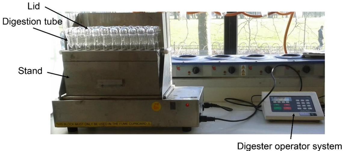
**Figure 3.1: Digestion Unit structure.**
