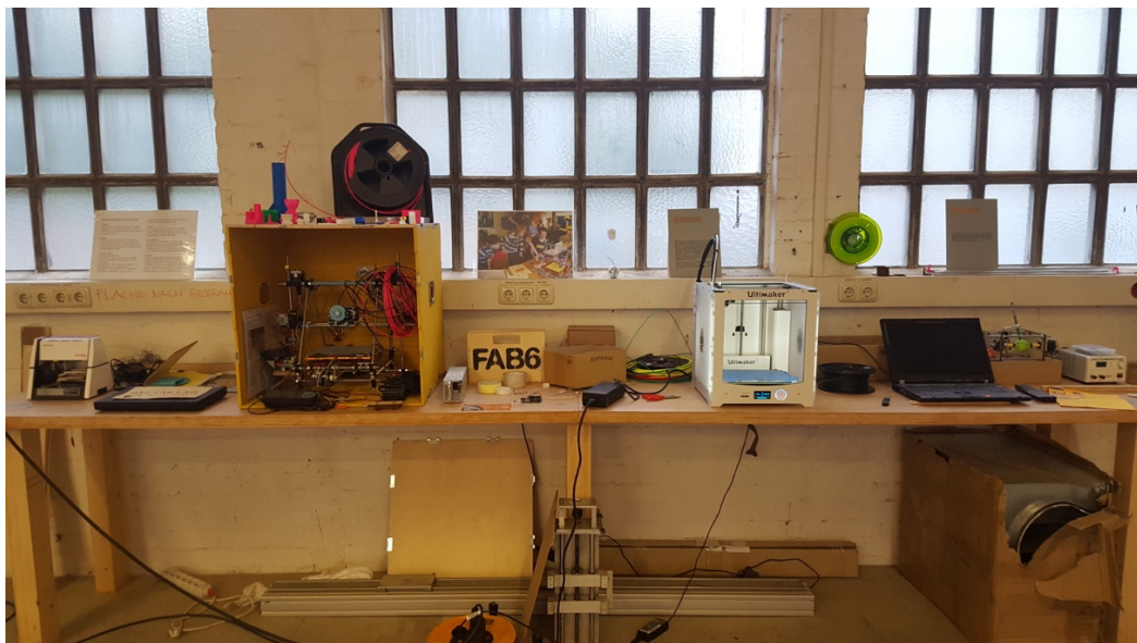
Figure 27 To the left is a RepRap under construction; to the right, an Ultimaker 3D printer. St. Pauli, Hamburg, Germany. Photo Credit: Leandros Savvides
