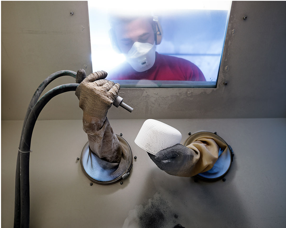
Figure 4 'A worker at HSL polishes a lampshade created by a 3D printer.' Photo credit: Luca Locatelli for Bloomberg Businessweek
