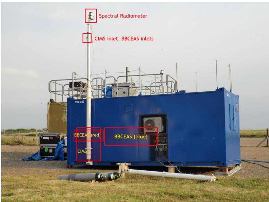
Figure 5.4 Housing for University of Leicester instruments during WAO campaign.
