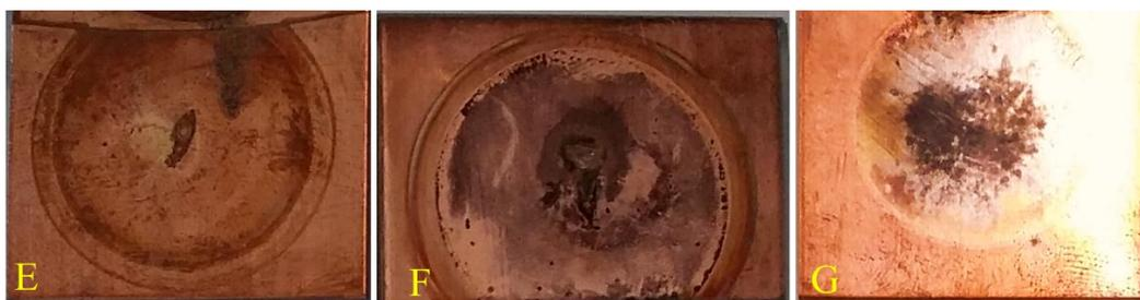
**Figure 4.8** Deposited 3 cm x 3 cm substrate images for experiments with applied +35 and -10 mA at  $47.5 \pm 2.5$  °C for deposition pulses of 80 ms, 800 ms, 1.5 s, and for dissolution pulses of 30 ms, 300 ms, and 500 ms, labelled as **E**, **F** and **G** respectively.
