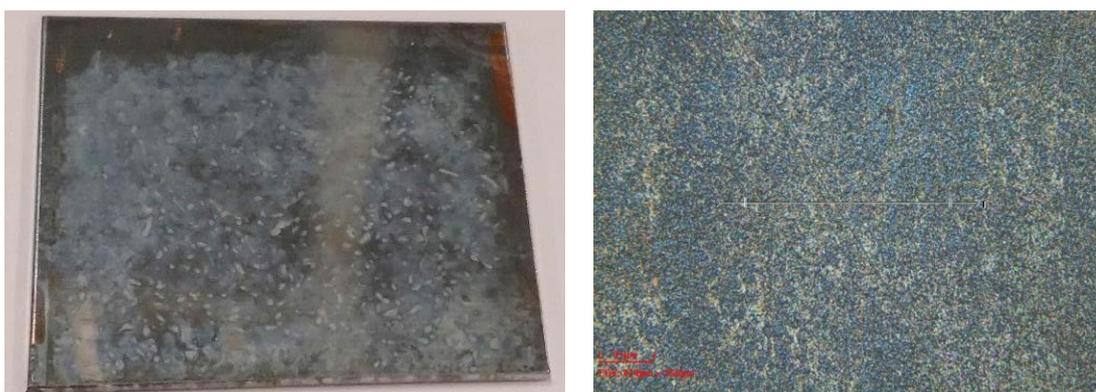
**Figure 4.14** photograph (left) and 3DM image (right) obtained using the cell shown in **Figure 4.13** by pasting zinc powder with 63 mA for 10 seconds deposition current, and 18 mA for 1 seconds dissolution current as given condition in **Table 4.3**. Powder applied with spatula onto substrate.
