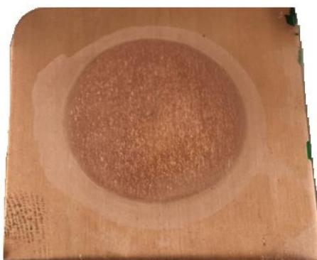
**Figure 4.7** Photograph of the 3 cm x 3 cm copper substrate after 3h experiment **A** with applied +50 mA for 1 ms, and -10 mA for 1 ms  $47.5 \pm 2.5$  °C.
