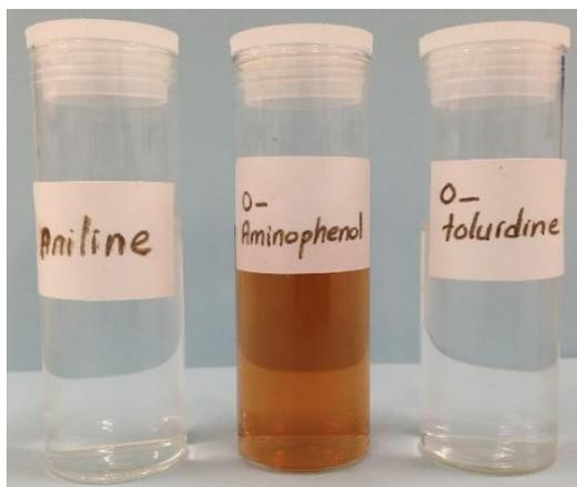
**Figure 3.4.** The images of monomer solutions of aniline, *o*-aminophenol, and *o*-toluidine in aqueous solutions, respectively
