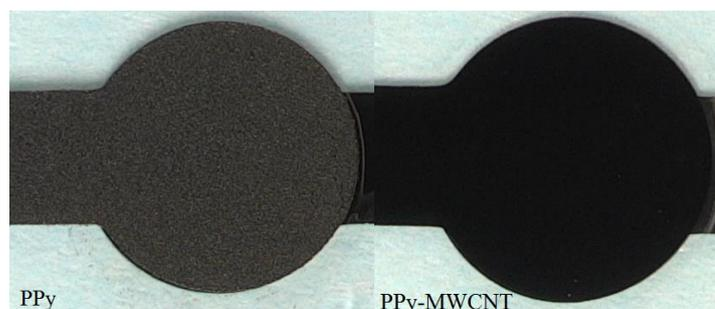
**Figure 7.16.** Images of the PPy and the PPy/MWCNTs films synthesised in Ethaline
