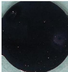
**Figure 7.5.** An image of the PPy without MWCNTs
