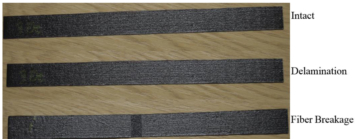
Fig 5-8: Actual shape of intact, delaminated and fibre breakage narrow laminated plate structures.
