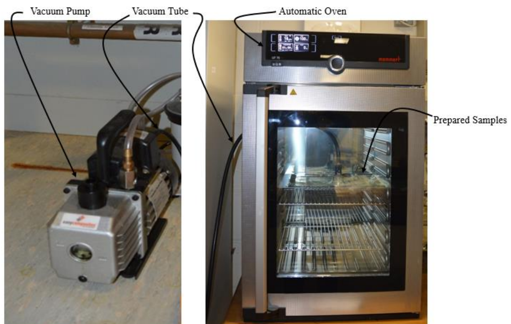
Fig 5-11: Automatic oven with vacuum pump.
