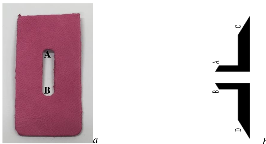
Figure 2.4: a) the shape of the cut sample tested in the double edge tear test and b). Test piece holder.
