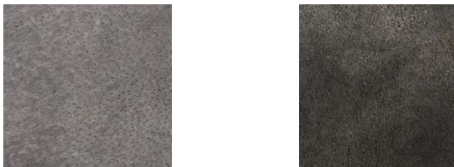
Figure 4.20: photographs of two samples of ovine skin (left) and bovine suede sample (right) treated with 10 wt% graphite in Ethaline.
