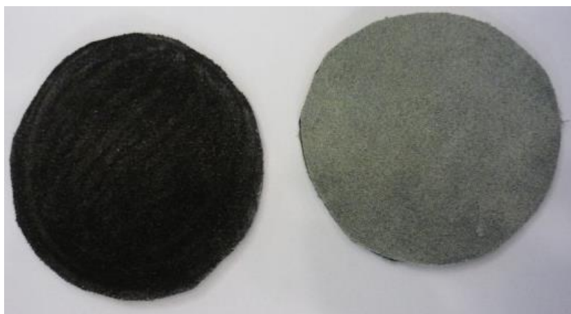
Figure 4.19: photographs of two samples of suede treated with graphite particles (left) 10 wt% graphite in Ethaline and (right) 10 wt% graphite in water.
