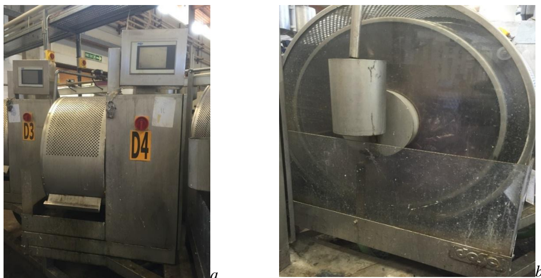
Figure 5.1: a) Drum used for pilot scale post tanning of ovine hide with DESs b) Photograph showing bag containing hide and DES in drum.
