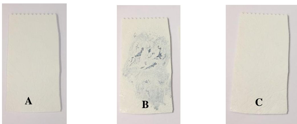
Figure 2.1: A) White leather sample, B) sample treated with indigo clothes dye C) sample after treating with DES.
