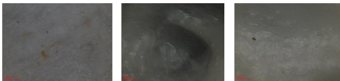
Figure 3.18: 2D Images for untreated bovine hide (A), and the sample treated in Ethaline for 24 h at (B) 50 °C and (C) 70 °C.
