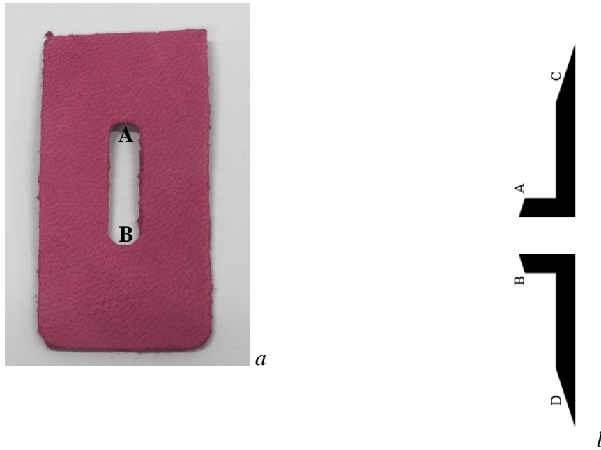
Figure 5.12: a) The shape of the cut sample tested in the double edge tear test and b) shape of the test piece holder.
