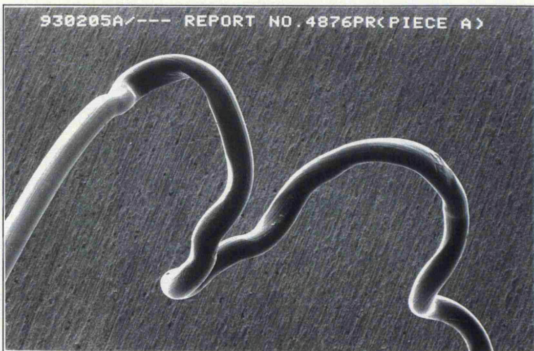
Figure 17.3: Scanning electron micrograph of middle of piece A: an unravelled knot.
