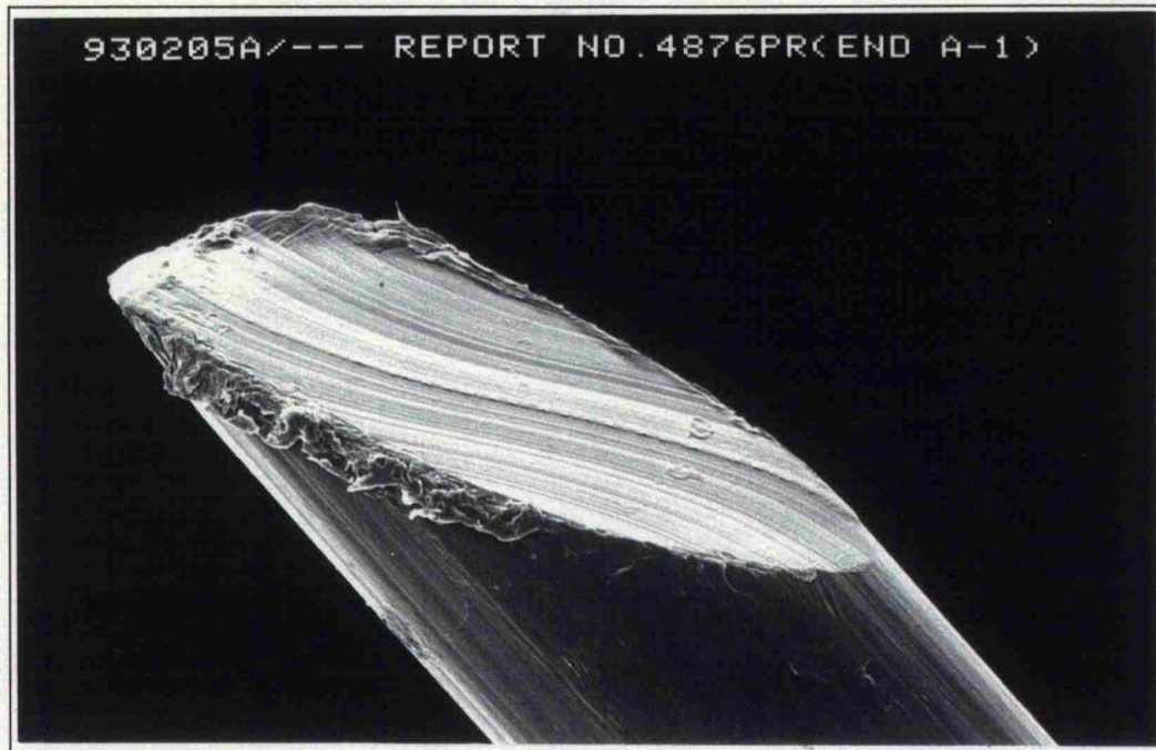
Figure 17.4: Scanning electron micrograph of end A1: A scalpel cut.
