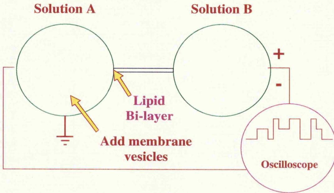
**Fig 6.** Diagram of the voltage clamp technique used to measure the conductance of ions through voltage operated ion channels in the membrane.
