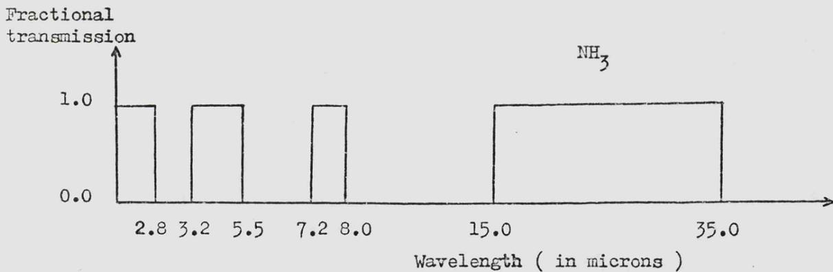
Step function approximation to the transmission curve of ammonia used by Sagan and Mullen (1971). Even for the small mixing ratio considered ( $10^{-5}$  by volume of NH<sub>3</sub> in 1 bar of H<sub>2</sub>) ammonia is seen to be a very efficient absorber - particularly around the peak of Planck curves for the temperature ranges of interest. Addition of even small amounts of NH<sub>3</sub> would lead to large temperature increments.
