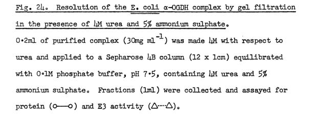
Table 12. Resolution of E. coli  $\alpha$ -OGDH complex by the method of Mukherjee et al. (1965). Detailed experimental conditions are described in section III.2.2. (+), activity
