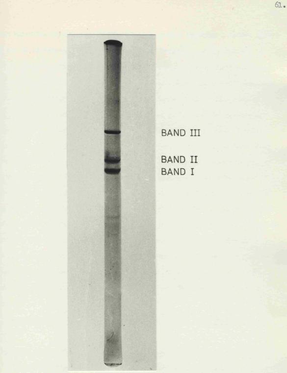
Fig. 18. Polyacrylamide gel electrophoresis of A. lwoffi  $\alpha$ -OGDH complex in the presence of sodium dodecyl sulphate. The gel was stained for protein with Coomassie Brilliant Blue. All experimental details are described in section II.2.9.
