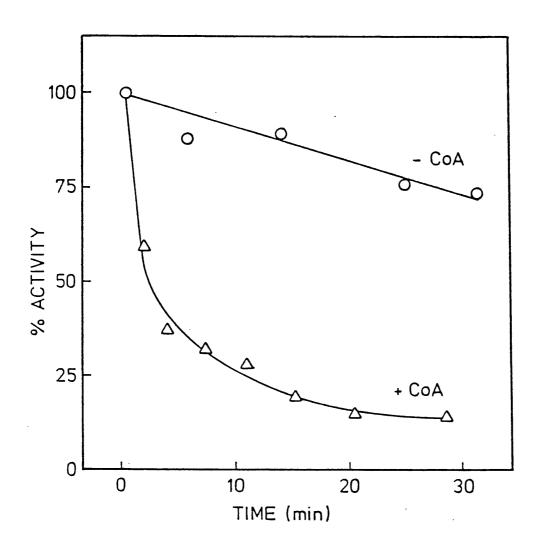
Fig. 49. Inactivation of E. coli  $\alpha$ -OGDH complex by CoA. 50µl of 5mM CoA were added to 200µg of E. coli  $\alpha$ -OGDH complex in lml of MET-8 buffer and incubated at 0°C. At intervals samples were removed and assayed for complex activity.
