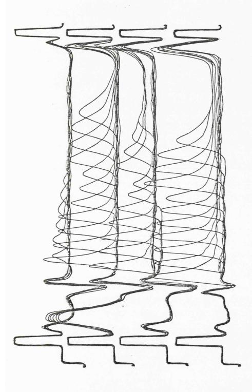
8% glycerol) were sedimented at 40,000rpm at  $5^{\circ}$ C in an MSE Centriscan 75 ultracentrifuge Samples of  $\alpha$ -OGDH (2.56, 5.13, 6.83 and 10.25mg ml<sup>-1</sup>in 0.1M Tris-HCl, pH 8.0 containing using Schlieren optics to observe the boundary position at suitable time intervals. Fig. 20. Sedimentation analysis of purified  $\alpha$ -OGDH complex from A. lwoffi. Experimental details are given in section II.º2.10.
