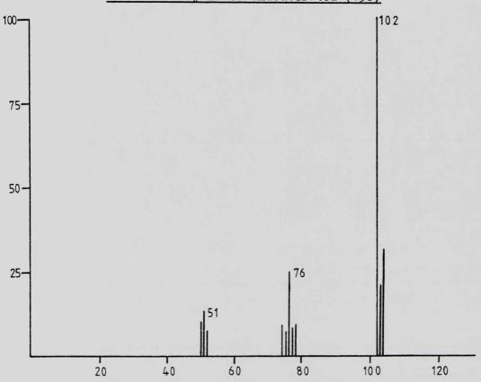
Figure 3.4 Mass spectrum of phenyl acetylene produced from thermolysis of deuterated (136)
