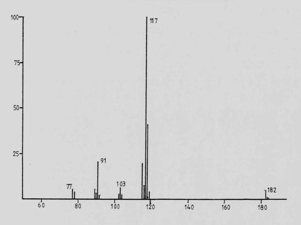
of the m/e = 137 peak - a metastable ion at 103.1 supports this proposition. Loss of SO from m/e = 165 to give m/e = 117 is also a possible fragmentation although there is no metastable ion to confirm this process. Loss of  $C_2H_2$  from this species would give m/e = 91.
