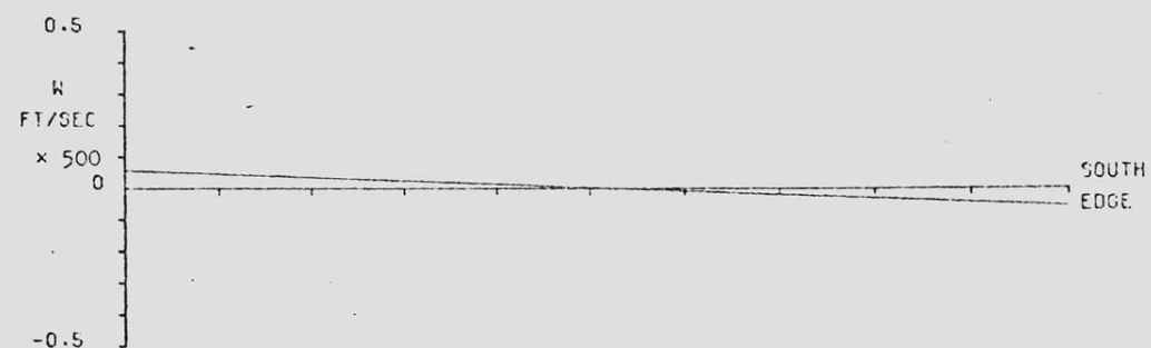
FIG 4.6 W FT/SEC (FIRST ORDER COMPONENT) SHOWN AS A FUNCTION OF DEPTH AND OF E THE DISTANCE FROM NORTH EDGE TO SOUTH EDGE CANAL WIDTH= 37.9 MLS, NEP=139.5 MLS \beta = 0.001
