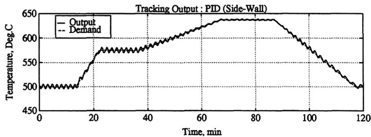
Figure 7.12: Response of Side-Wall Thermocouple under PID Control
