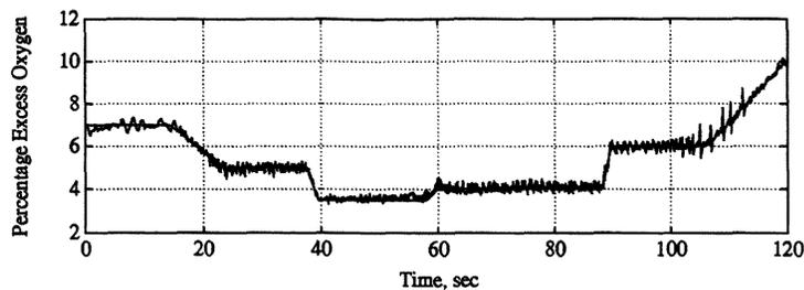
Figure 8.7: Excess oxygen in the flue compared to the reference (3rd design)
