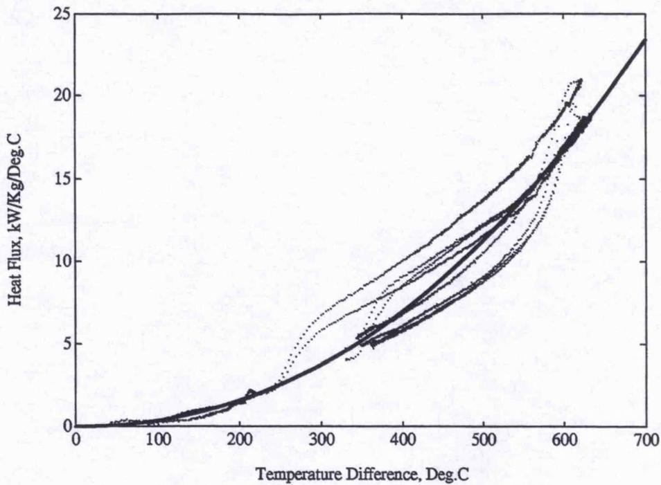
Figure 6.7: Measured heat Flux compared to the empirical relationship
