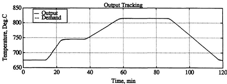
Figure 7.4: Nonlinear simulation under sliding mode control
