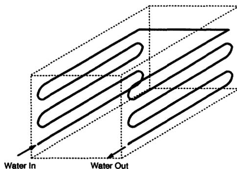
Figure 6.6: Schematic of the pipe arrangement in the water cooling system
