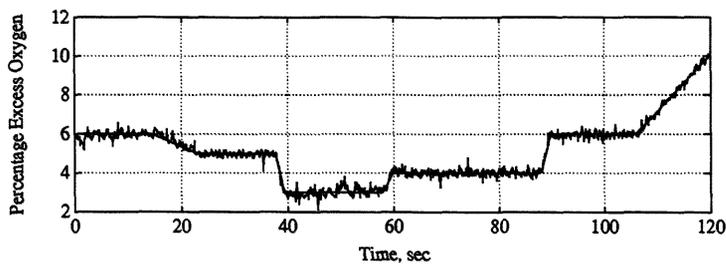
Figure 8.5: Excess oxygen in the flue compared to the reference (2nd design)
