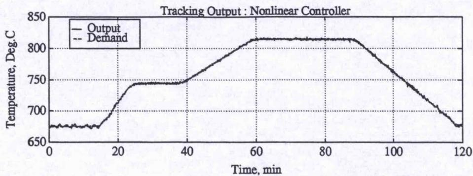
Figure 7.9: Response of End-Wall Thermocouple under Nonlinear Control
