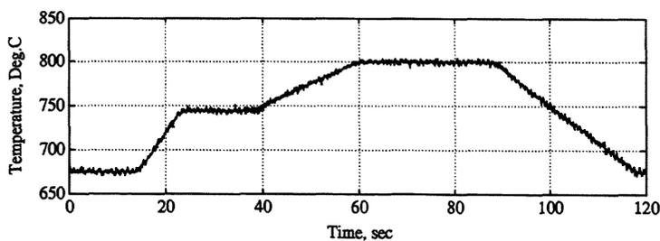
Figure 8.4: Furnace temperature compared to the reference (2nd design)
