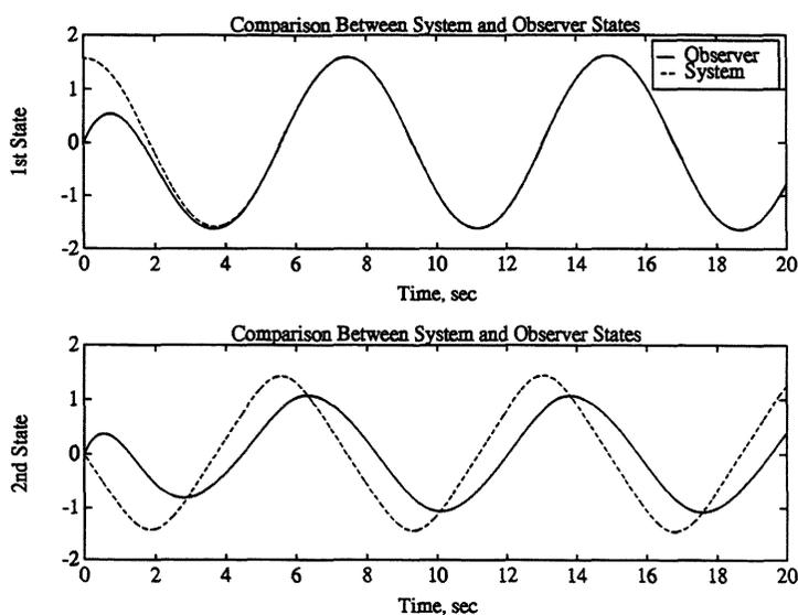
Figure 3.5: Comparison between system and observer states
