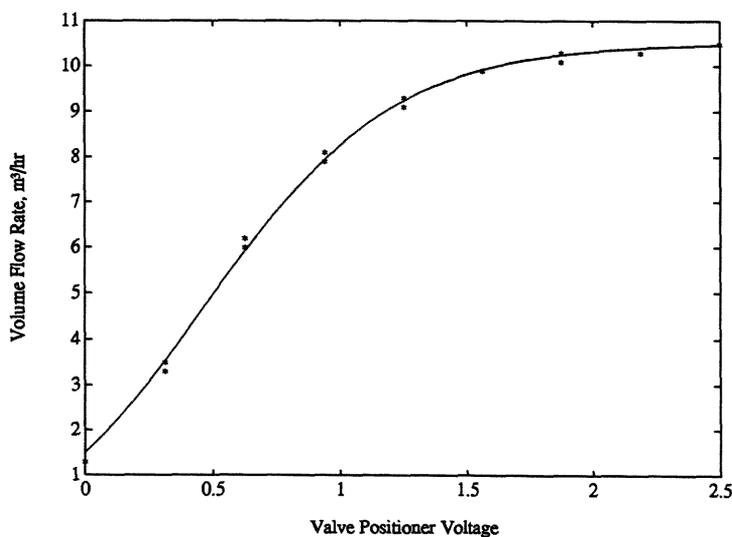
Figure 6.9: Steady state volume flow rate against valve position
