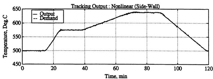
Figure 7.11: Response of Side-Wall Thermocouple under Nonlinear Control
