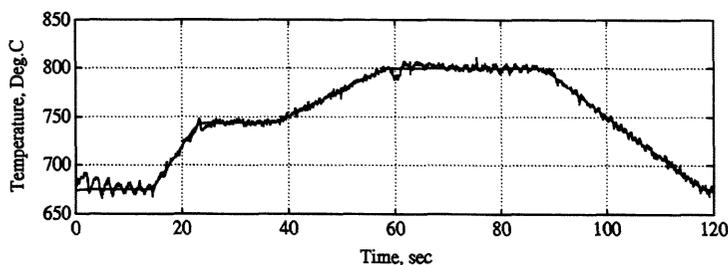
Figure 8.2: Furnace temperature compared to the reference (1st design)
