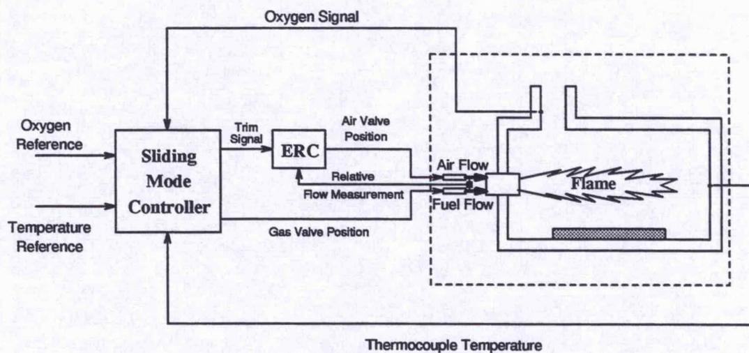
Figure 8.1: Schematic of proposed multivariable control scheme
