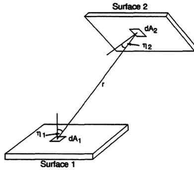
Figure 6.2: Direct exchange area between surfaces
