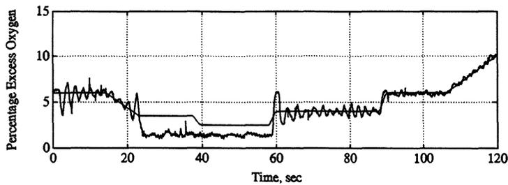
Figure 8.3: Excess oxygen in the flue compared to the reference (1st design)
