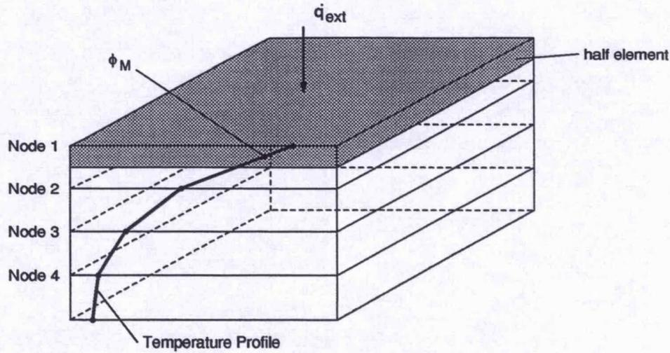
Figure 6.4: Half element at the surface
