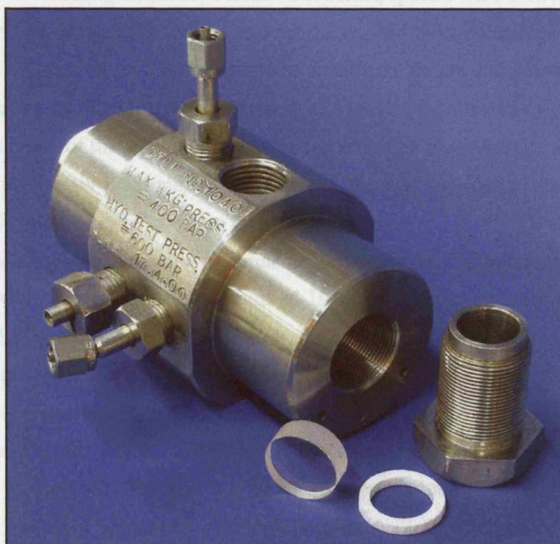
Figure 2.5 High-pressure optical cell used for visual observations
